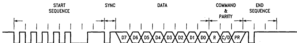
FIGURE 1-2. IBM 3270 Message Format
