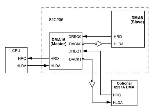
When programming cascaded controllers, begin with the device which is actually generating HRQ to the system (first level device) and then proceed to the second level devices. RESET causes the DACK outputs to become active low and
