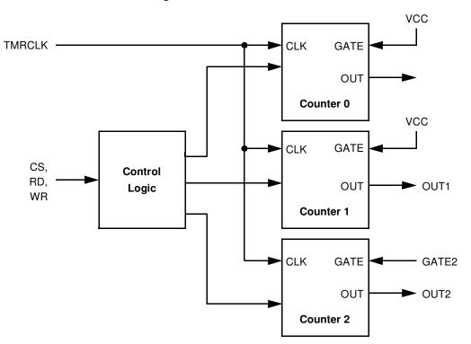
Figure 4-6 Counter/Timer Block Diagram
