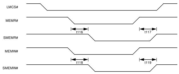
Figure 6-8 Master Mode Word SA to CA Address Timing
