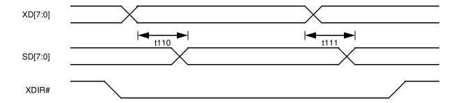
Figure 6-5 SD[7:0] to XD[7:0] Timing
