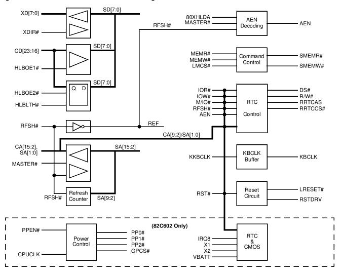
Figure 2-2 82C802G/82C601/602-Based System Block Diagram
