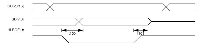
Figure 6-2 SD[7:0] to CD[23:16] Timing
