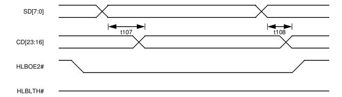
Figure 6-4 XD[7:0] to SD[7:0] Timing
