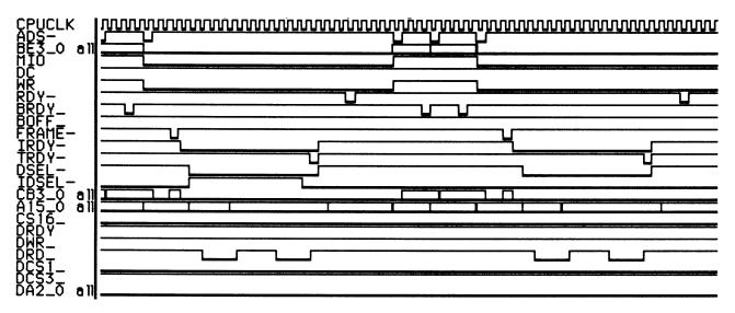
Figure 6-7 32-Bit I/O Write
