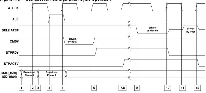
Figure A-5 Compact ISA Configuration Cycle Operation
