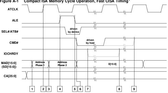
Figure A-1 Compact ISA Memory Cycle Operation, Fast CISA Timing<sup>1</sup>
