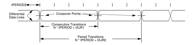
Figure 6-5 Differential to EOP Transition Skew and EOP Width
