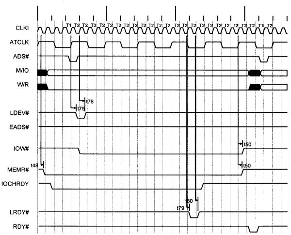
Figure 6-19 DMA Write Cycle
