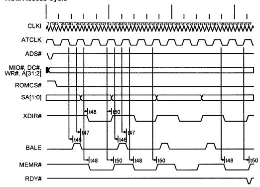
Figure 6-23 Keyboard Controller Access Cycle
