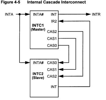
**Note:** INTA will be active when the CPU initiates an interrupt acknowledge cycle.
