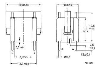
Fig. 1 Line driver transformer AT4043/89.
