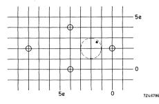
Fig. 2 Hole pattern for mounting on a printed-wiring board. Grid hole diameter = 1,3  $\pm$  0,1 mm; e = 2,54 mm (0,1 in).
