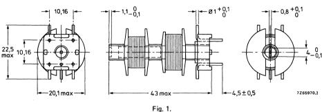
The coil has five pins for mounting on a printed-wiring board. It can be adjusted at the top by means of a trimming key.
