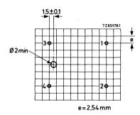
Hole pattern for mounting on a printed-wiring board; hole diameter  $1,3 \pm 0,1$  mm.
