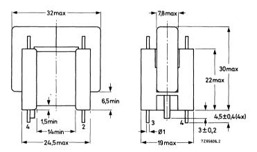
Fig. 1 Line driver transformer AT4043/83.
