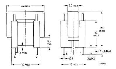
Fig. 1 Line driver transformer AT4043/64.
