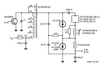
Fig. 4a Diode modulator with split tuning.
