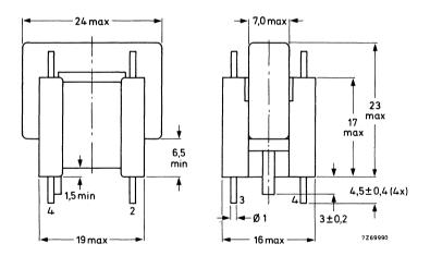
Fig. 1 Line driver transformer AT4043/59.
