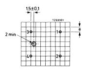
Fig. 2 Hole pattern for mounting on a printedwiring board (component side). Hole diameter 1,3 + 0,1 mm. e = 2,54 mm (0,1 in).
