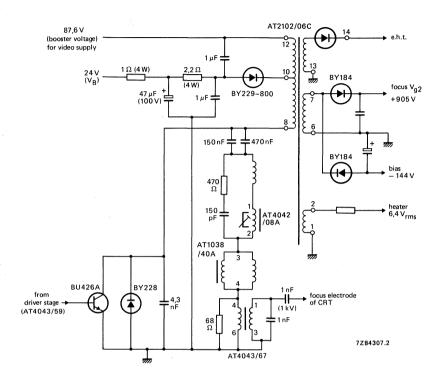
Fig. 3 Application circuit.
