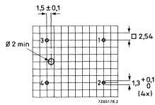
Fig. 2 Hole pattern for mounting on a printedwiring board (component side). Hole diameter 1,3 + 0,1 mm; e = 2,54 mm (0,1 in).
