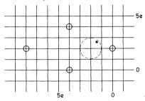
Fig. 2 Hole pattern for mounting on a printed-wiring board. Grid hole diameter = 1,3  $\pm$  0,1 mm;  $^{7246786}$  e = 2.54 mm.
