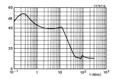
Fig. 4 Insertion loss measured in the 60  $\Omega$  circuit of Fig. 5.
