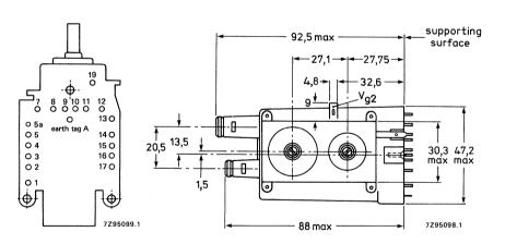
Fig. 1 Line output transformer AT2077/81.
