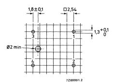
Fig. 2 Hole pattern for mounting on a printedwiring board (component side).
