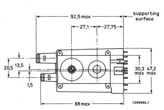
Fig. 1 Line output transformer AT2077/82.
