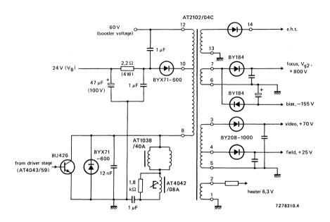
Fig. 3 Application circuit.
