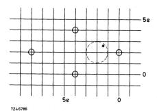
Fig. 2 Hole pattern for mounting on a printedwiring board; e = 2,54 mm.
