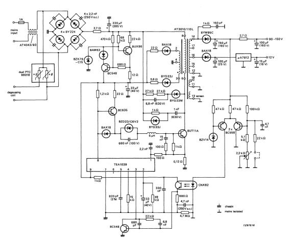
Fig. 5 Application circuit; 90 - 264 V mains input, 70 W output power.
