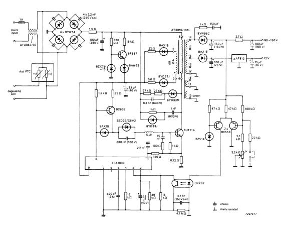
Fig. 4 Application circuit; 220/240 V mains input, 120 W output power.
