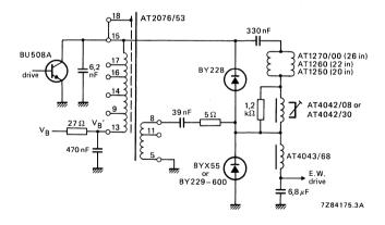
Fig. 4b Diode modulator with tap on transformer.
