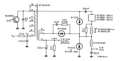
Fig. 4c Three-diode modulator circuit.
