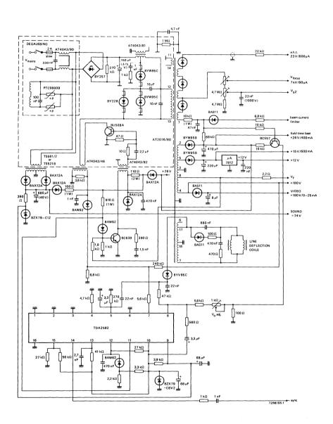
Fig. 3 Application circuit.
