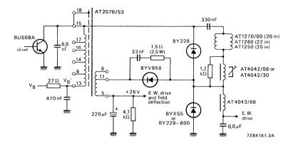
Fig. 4c Three-diode modulator circuit.
