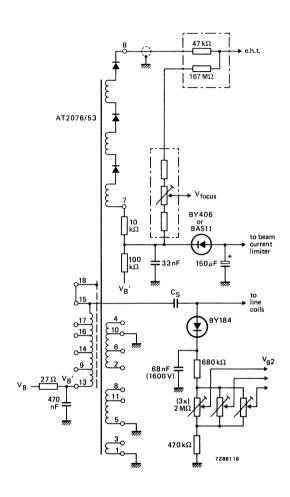
Fig. 3 Circuit diagram of transformer, and e.h.t., focus voltage and  $\mathrm{V}_{g2}$  circuits.
