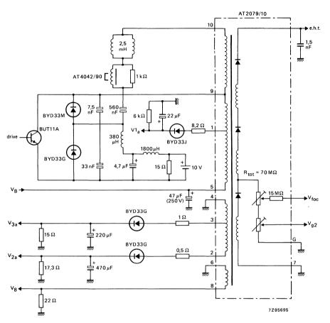
Fig. 3 Application circuit with diode modulator.
