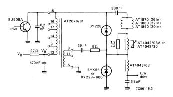
Fig. 4b Diode modulator with tap on transformer.
