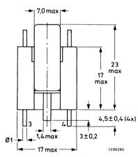
Fig. 2 Hole pattern for mounting on a printed-wiring board (component side); e = 2,54 mm; hole diameter is 1,3 + 0,1 mm. The windings may be interchanged because the coil is symmetrical.
