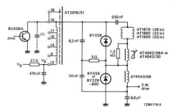
Fig. 4a Diode modulator with split tuning.
