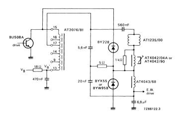
Fig. 5a Diode modulator,  $V_B' = 150 \text{ V}$ .
