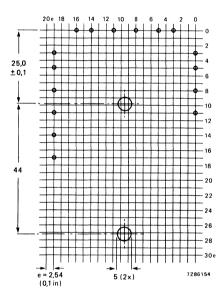
Fig. 2 Hole pattern for mounting on a printed-wiring board (solder side). Grid hole diameter 1,3 ± 0,1 mm.
