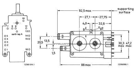
Fig. 1 Line output transformer AT2077/80.
