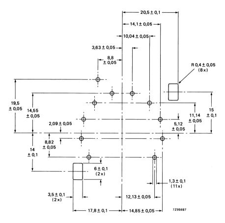
Fig. 2 Mounting hole pattern (solder side).
