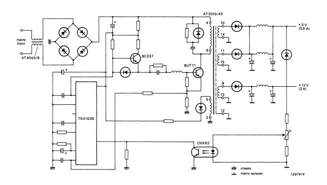
Fig. 4 Application circuit.
