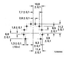
Fig. 2 Mounting hole pattern.
