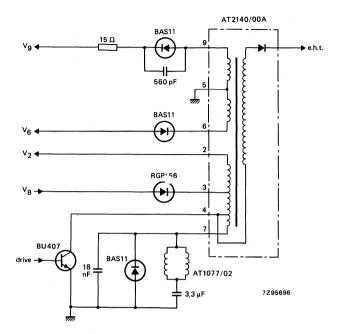
Fig. 3 Application circuit.
