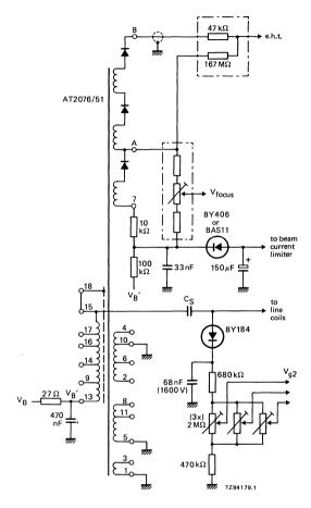
Fig. 3 Circuit diagram of transformer, and e.h.t., focus voltage and  $\mathrm{V}_{g2}$  circuits.
