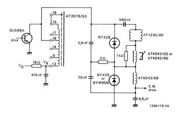
Fig. 5b Diode modulator,  $V_B = 134,3 \text{ V}$ .
