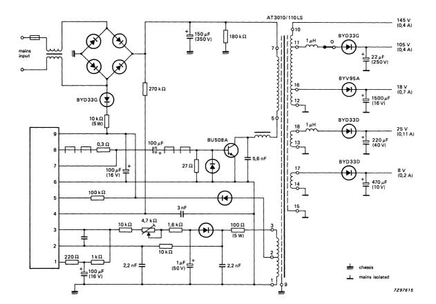
Fig. 4 Application circuit, with IC TDA4600.
