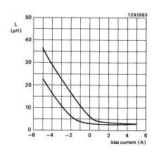
Fig. 4 Inductance as a function of bias current.
