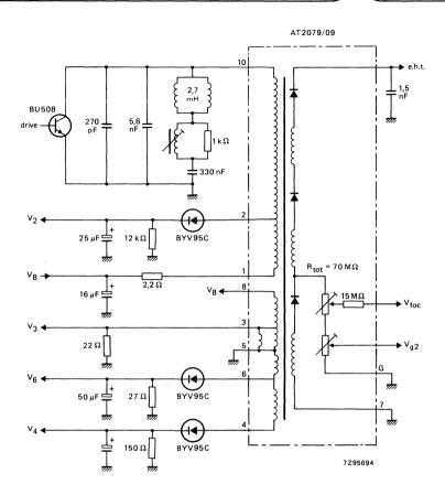
Fig. 3 Application circuit.
