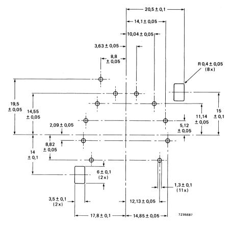
Fig. 2 Mounting hole pattern (solder side).
