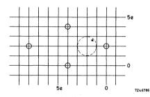
Fig. 2 Hole pattern for mounting on a printedwiring board (e = 2,54 mm (0,1 in); grid hole diameter 1,3 ± 0,1 mm.
