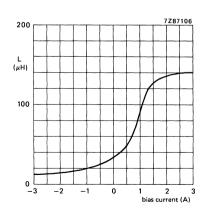
Fig. 4 Inductance as a function of bias current.
