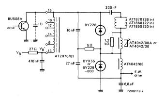
Fig. 4a Diode modulator with split tuning.
