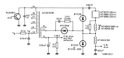
Fig. 4c Three-diode modulator circuit.
