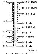
Fig. 3 Circuit diagram.
