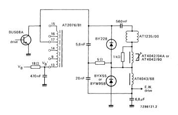
Fig. 5b Diode modulator,  $V_{B'} = 130 V$ .
