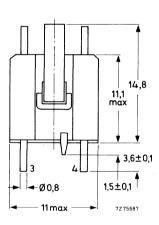
Fig. 1 Line driver transformer AT4043/56.
