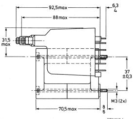
Fig. 1 Line output transformer AT2076/84.
