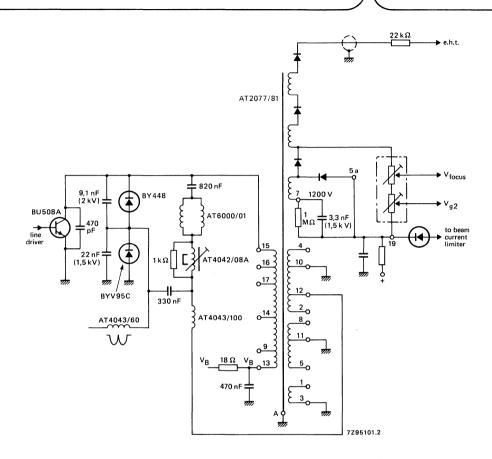
Fig. 5 Application circuit.
