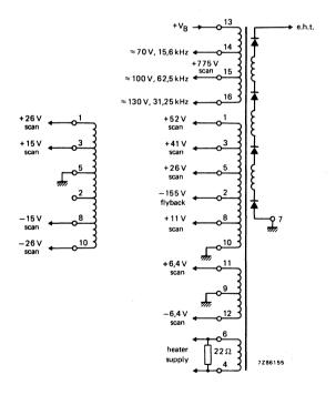
Fig. 6 Application circuit.
