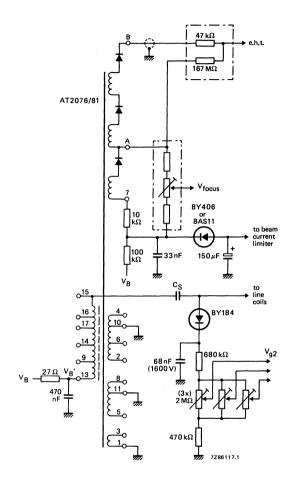
Fig. 3 Circuit diagram of transformer, and e.h.t., focus voltage and  $\rm V_{g2}$  circuits.
