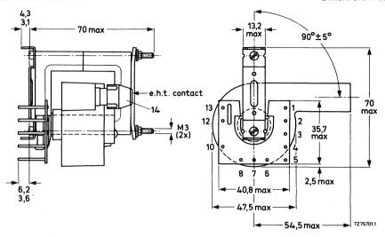
Fig. 1a Line output transformer AT2102/04C.
