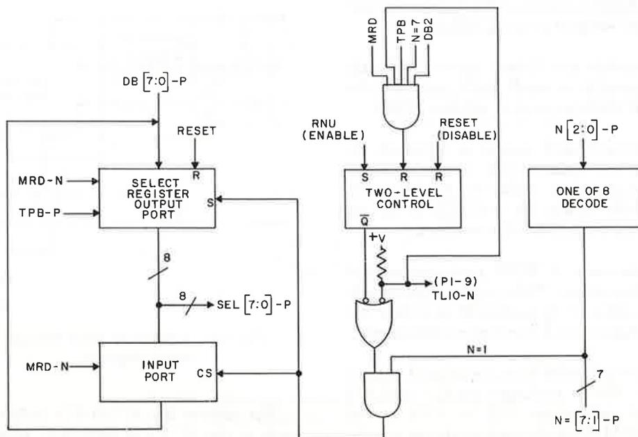
Fig. 10 - I/O Decode Module CDP18S509 block diagram.
