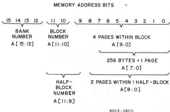
Fig. 17 - Memory address bit assignments.
