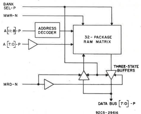
Fig. 12 – 4-Kilobyte RAM Module CDP18S205 block diagram.
