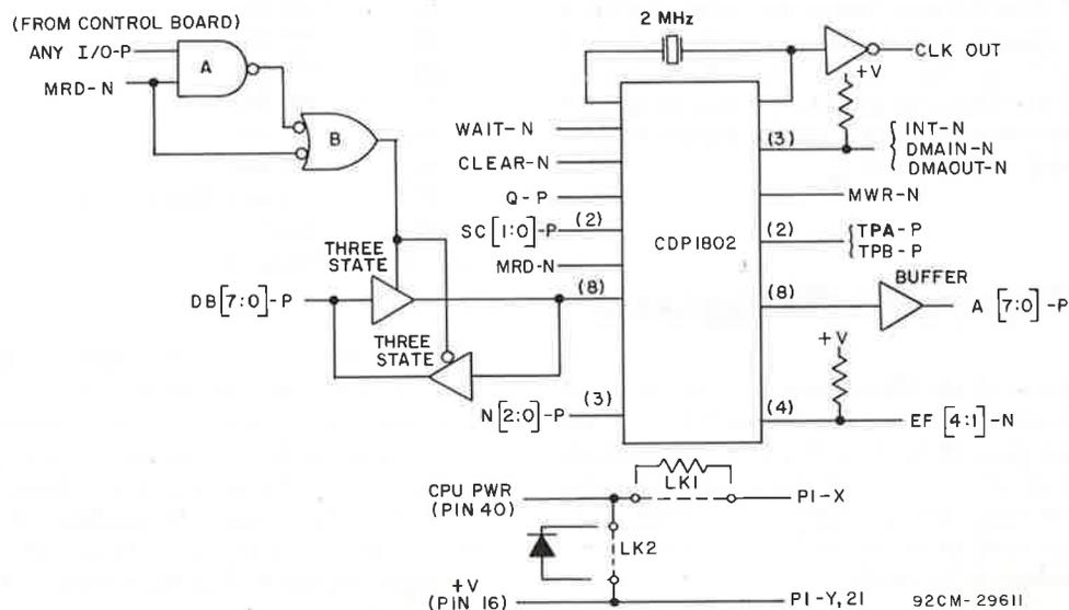
Fig. 7 - CPU Module CDP18S102 block diagram.
