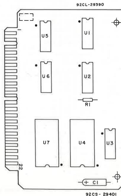
Fig. D8 - I/O decode module CDP18S509 layout diagram.
