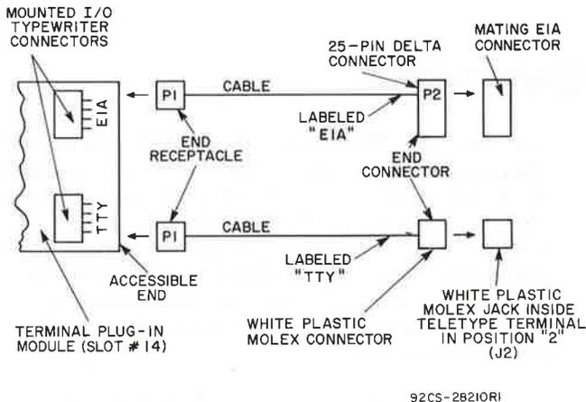
Fig. 1 - Cable connection for I/O data terminals.
