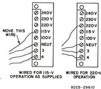
Fig. 11 - Conversion for different operating voltages.
