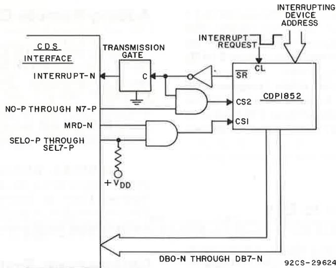
Fig. 22 - General-purpose circuit for vectored interrupts.
