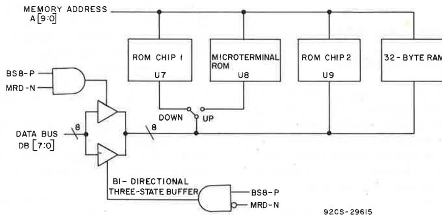
Fig. 11 – ROM/RAM Module CDP18S401 block diagram.
