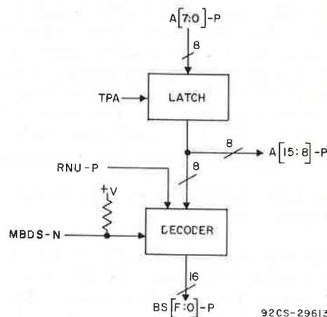
Fig. 9 — Address Latch and Bank Select Module
