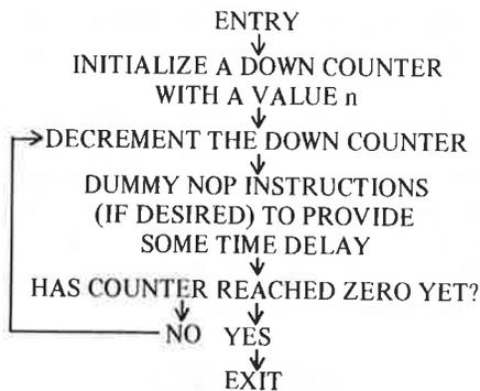
This flow chart, of course, is a much more understandable version of the program. The time from ENTRY to EXIT is approximately  $n_{16}$  times the time for one pass through the loop.
