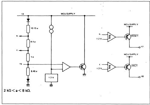
Note : Reset and Halt outputs, which are open collector outputs, require external resistors to zero volt.
