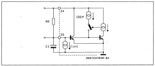
At "Off-hook", with only DC voltage applied to the line terminals, C1 fixes the timing of the line current profile at : \_\_\_\_\_ 150mA max for a time shorter than 400msec T-charge of 240msec (typ) is obtained with  $C1 = 220\mu F$ .
