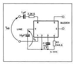
Figure 3 : Application Compatible with LS1240 (single ended output).
