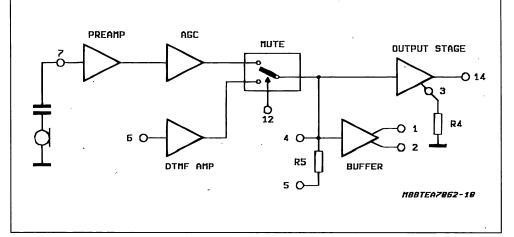
2.1 A.G.C. IN TRANSMISSION. The transmission gain between Microphone Input (pin 7) and Vline (pin 14) is internally decreased of 6dB when the line current varies from ILL to ILS with a constant AC load of  $600\Omega$ .
