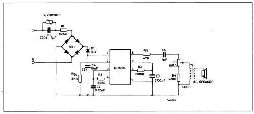
Figure 11 : ML8204 Test Circuit (power supply transient).
