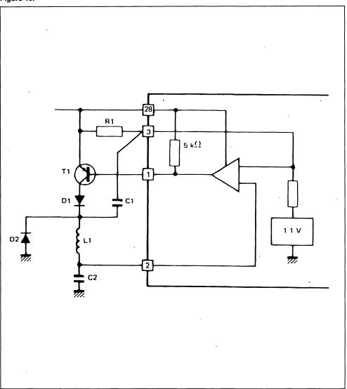
Transistor T1 is switched either ON/OFF via pin 1 in accordance with the result of a comparison between an internal reference voltage and the I.C. supply voltage (pin 2). When transistor T1 is off, the diode
