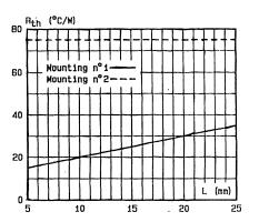
Fig.2 - Thermal resistance versus lead length.
