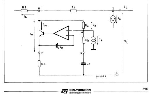
It is important to note that the DC voltage at pin 5 is proportional to the line current ( $V_5 = V_7 + V_B = (I_L - I_0) R3 + V_B$ ).
