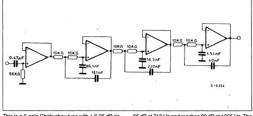
This is a 6-pole Chebychev type with  $\pm$  0.25 dB ripple in the passband. A decoupling stage is used to avoid the influence of the input impedance on the filter's characteristics. The attenuation is about
