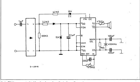
If pin EIN is connected to  $V_{\text{DD}}$  the ringer is activated by frequencies upper than 20 Hz.
