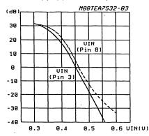
Figure 3 : Power Available on Loudspeaker versus V<sub>LS</sub> Typical Curve.
