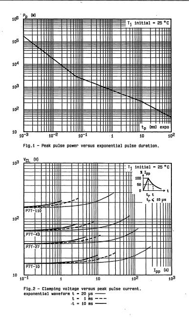
Note : The curves of the figure 2 are specified for a junction temperature of 25 °C before surge. The given results may be extrapolated for other junction temperatures by using the following formula :  $\Delta V$  (BR) =  $\alpha T (V (BR)) X [T_j - 25] X V (BR)$  For intermediate voltages, extrapolate the given results.
