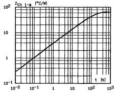
Fig.6 - Transient thermal impedance junction-ambient for mounting  $n^{\circ}2$  versus pulse duration (L = 10 mm).
