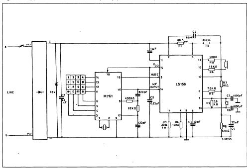
Figure 8 : Application Circuit with Multifrequency (EUROPE II std.).
