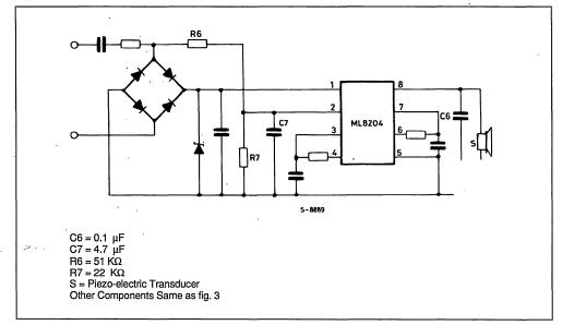
Figure 16 : ML8204/5 Circuit to eliminate Tail-off.
