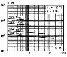
Fig.8b - Capacitance versus reverse applied voltage for bidirectional types (typical values). D88P6KEP6
