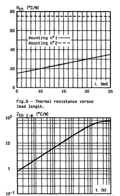
Fig.6 - Transient thermal impedance junction-ambient for mounting n°2 versus pulse duration (L = 10 mm).
