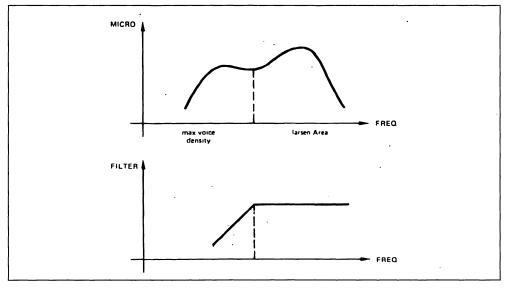
To extract the larsen component, the microphone signal is first filtered by a second order filter (formed
