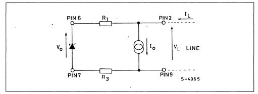
Figure 6 : Circuit Configuration of the Shunt Regulator.
