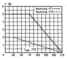
Fig.4 - Power dissipation versus ambient temperature.
