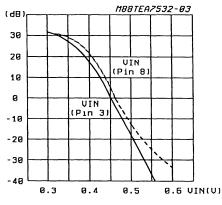
Figure 2 :Loudspeaker Gain Versus Voltage on Pin (3) - (8) and Versus R<sub>2</sub>.
