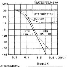
$R_2 = 10 \text{ K} \Rightarrow \text{ATT} = 20 \text{ dB}$  $R_2 = 3 \text{ K} \Rightarrow \text{ATT} \approx 10 \text{ dB}$
