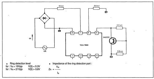
Figure 4 : Ring Detection Distortion.
