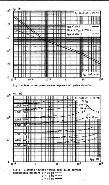
Note : The curves of the figure 2 are specified for a junction temperature of 25 °C before surge. The given results may be extrapolated for other junction temperatures by using the following formula :  $\Delta V$  (BA) =  $\alpha$  T (V (BA)) X [Tj - 25] X V (BA) For intermediate voltages, extrapolate the given results.
