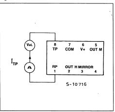
OUTL output will sink output current when the OUTH output is connected to the mirror input and when ringing is detected (see application diagram figure 11 and 12). The device does not have to depend upon power derived from the Tip-Ring inputs to become operational. Connecting an external voltage source to V+ will also allow the device to operate in what is described as "Stand Alone Applications".
