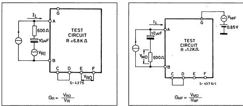
**ELECTRICAL CHARACTERISTICS** (refer to the test circuits, S1 and S2 in (a),  $T_{amb} = -25$  to + 50 °C, f = 200 to 3400 Hz, unless otherwise specified)
