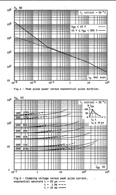
Note: The curves of the figure 2 are specified for a junction temperature of 25 °C before surge. The given results may be extrapolated for other junction temperatures by using the following formula:  $\Delta V$  (BA) =  $\alpha \tau$  (V (BA)) X [T<sub>j</sub> - 25] X V (BA) For intermediate voltages, extrapolate the given results.
