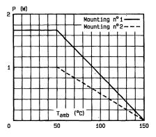
Fig.4 — Power dissipation versus ambient temperature.
