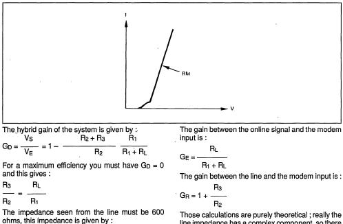
Those calculations are purely theoretical; really the line impedance has a complex component, so there will be little changes in the value of R<sub>1</sub>, R<sub>2</sub>, R<sub>3</sub> to adapt the hybrid system.
