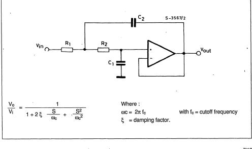
Three parameters are needed to characterize the frequency and phase response of a 2<sup>nd</sup> order active filter : the gain  $(G_v)$ , the damping factor  $(\xi)$  or the Qfactor (Q =  $(2\xi)^{-1}$ ), and the cutoff frequency (fc). The higher order responses are obtained with a se-
