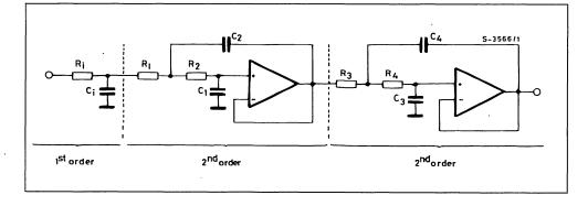
Figure 15: 5<sup>th</sup> Order Low Pass Filter (Butterworth) with Unity Gain Configuration.
