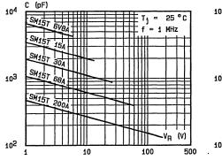
Fig.8a - Capacitance versus reverse applied voltage for unidirectional types (typical values).
