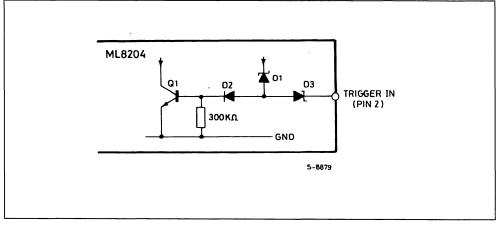
Figure 5a : Enabling Oscillation of the ML8204 for Supply Voltages less than V<sub>si</sub>.
