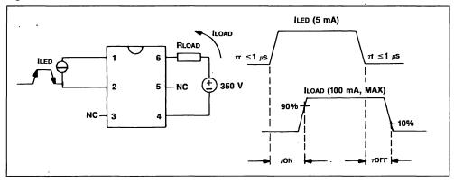
Figure 4 : TON/TOFF Test Circuit and Waveform.
