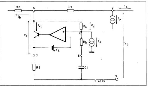
The difference  $l_L - l_o$  flows through the shunt regulator being  $l_b$  negligible.
