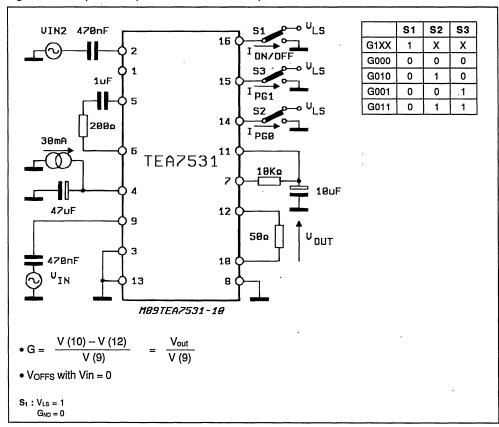
Figure 7 : Loudspeaker Amplifier : Gain/Distortion/Output Offset.
