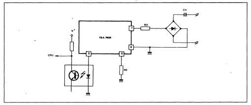
The ringing signal coming from the line is rectified by the diode bridge ; the circuit compares the peak amplitude of the signal to a predeterminated detection level fixed by Rs. On the output transistor of the optocoupling device a logic signal is generated which frequency is twice the frequency of the ringing signal.
