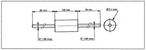
Cooling method : by conduction (method A) Marking : type number Weight : 0.9 g
