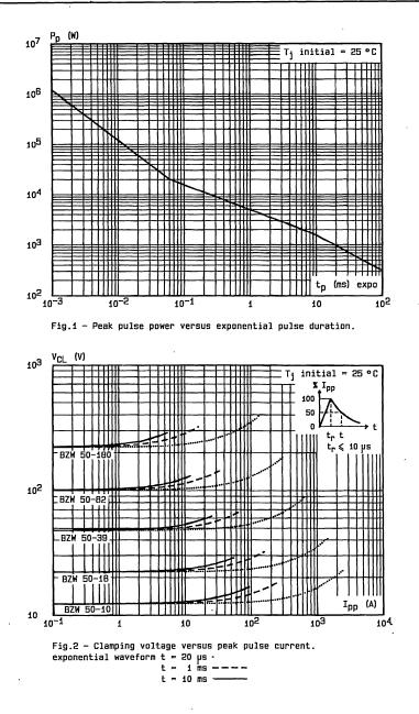
Note: The curves of the figure 2 are specified for a junction temperature of 25 °C before surge. The given results may be extrapolated for other junction temperatures by using the following formula:  $\Delta V$  (BA) =  $\alpha$  T (V (BA)) X [T<sub>j</sub> - 25] X V (BA) For intermediate voltages, extrapolate the given results.
