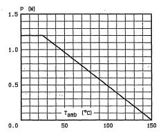
Fig.4 - Power dissipation versus ambient temperature.
