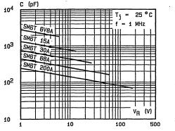
Fig.8a - Capacitance versus reverse applied voltage for unidirectional types (typical values).
