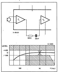
For the version originally developed for electrodynamic/magnetic microphones it is also possible to use electret microphones as shown in fig. 20.
