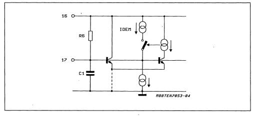
At "Off-hook", with only DC voltage applied to the line terminals, C1 fixes the timing of the line current profile at :
