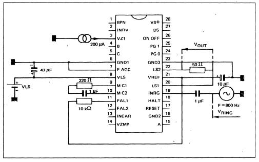
Figure 3 : Test Loudspeaker Amplifier - Gain - Distortion - ILS.
