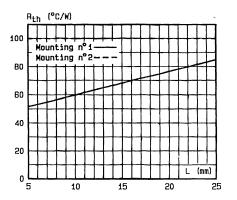
Fig.2 - Thermal resistance versus lead length.
