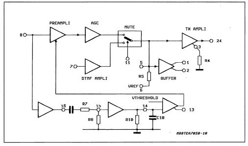
2.1. A.G.C. IN TRANSMISSION. The transmission gain between Microphone Input (pin 8) and Vline (pin 24) is internally decreased of 6dB when the line current varies from 27mA to 42mA with a constant AC load of 6000hms.
