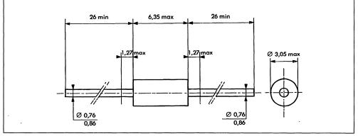
Cooling method : by conduction (method A) Marking : type number Weight : 0.4 g
