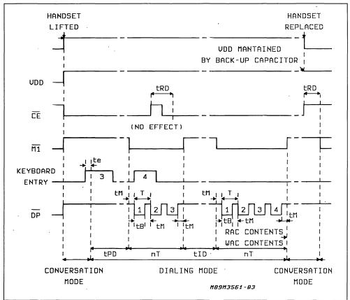
(1) Oscillator off. All registers except WAC reset. Keyboard input inhibited. Number stored in RAM until VDD >= 1V.
