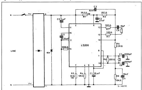
Figure 12 : Application Circuit without Multifrequency.
