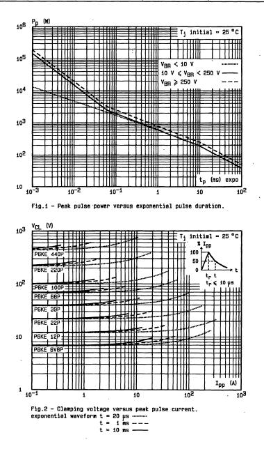
Note : The curves of the figure 2 are specified for a junction temperature of 25 °C before surge. The given results may be extrapolated for other junction temperatures by using the following formula :  $\Delta V$  (BR) =  $\alpha$  T (V (BR)) X (T<sub>j</sub> = 25) X V (BR) For intermediate voltages, extrapolate the given results.
