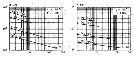
Fig.8a - Capacitance versus reverse applied voltage for unidirectional types (typical values).
