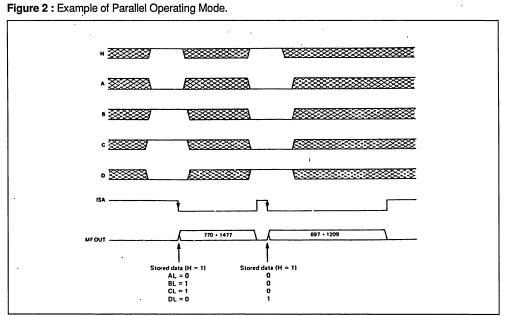
Note : If the circuit operates permanently in parallel mode, then the H input may be left floating (internally pulled-up to V\*) or tied to logic 1. With ISA at logic 0, H,A,B,C, and D inputs cannot modify the generated DTMF pair.
