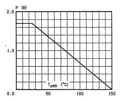
Fig.4 - Power dissipation versus ambient temperature.
