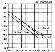
Figure 9 : Normalized On-resistance vs. Temperature.
