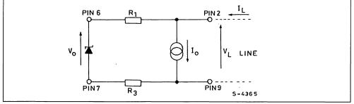
A fixed amount Io of the total available current IL is drained for the proper operation of the circuit.
