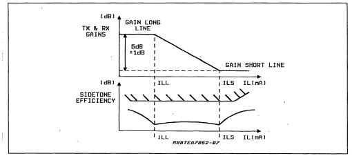
4.1 PROGRAMMABLE CONTROLS. AGC and sidetone attack and disonnect points (or currents) are programmable externally through two independents pins, I-start (pin 19) and I-slope (pin 13).
