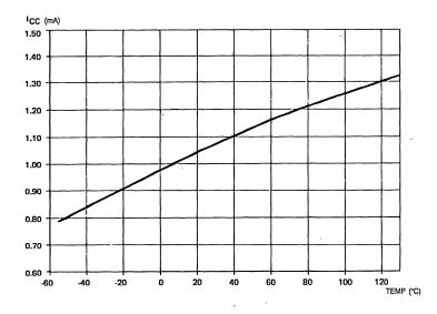
SUPPLY CURRENT VS. AMBIENT TEMPERATURE
