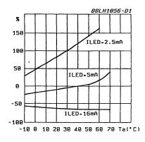
Figure 7 : Normalized Turn-off Time vs. Temperature.
