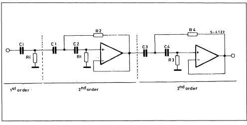
Figure 17 : Multiple Feedback 8-pole Bandpass Filter.
