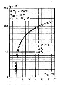
Fig.7 - Peak forward ourrent versus peak forward voltage drop (typical values for unidirectional types).
