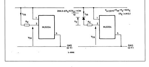
Oscillation of the ML8204 may be inhibited for voltages in the range  $V_{si} < Vs \leq V_{s(max)}$  by sinking the current from D<sub>1</sub>, starving Q<sub>1</sub> of base current. This is achieved by either a) grounding pin 2 (fig. 6a), or b) applying a voltage  $V_{\rm INH}$  via a resistor R<sub>1</sub> to pin 2 (fig. 6b) to ensure that :
