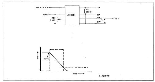
Figure 8 : Current Limiting Characteristics.
