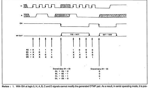
es: 1. With ISA at logic 0, H, A, B, C and D signals cannot modify the generated D I M- pair. As a result, in serial operating mode, it is possible to enter AS, BS, CS and DS data while another DTMF pair is being generated.
