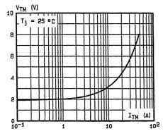
Fig.5 - On-state voltage versus on-state current (typical values).
