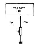
Rlp In MW =  $\frac{7.8}{\text{lp}\mu\text{A}}$ For Rlp = 390K to 1% DG =  $-2\text{dB} \pm 0.4\text{dB}$
