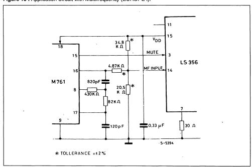
Figure 10 : Application Circuit with Multifrequency (EUROPE I).
