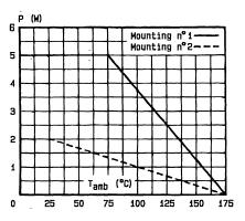
Fig.4 - Power dissipation versus ambient temperature.
