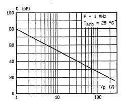
Fig.4 - Junction capacitance versus reverse applied voltage.
