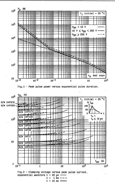
Note: The curves of the figure 2 are specified for a junction temperature of 25 °C before surge. The given results may be extrapolated for other junction temperatures by using the following formula:  $\Delta V$  (BR) =  $\alpha T$  (V (BR)) X [Tj - 25] X V (BR) For intermediate voltages, extrapolate the given results.
