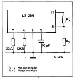
In addition to the above mentioned applications, different values for the external components can be used in order to satisfy different requirements.
