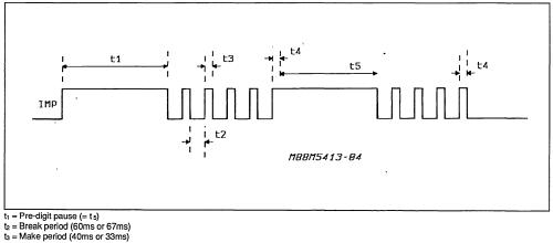
$t_4 = Post-digit make (= t_3)$  $t_5 = Inter-digit pause (500 or 800ms)$
