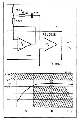
Figure 21 : Typical Receive Gain.
