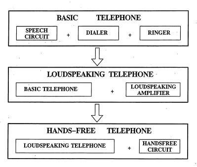
MODULAR APPROACH. The SGS-THOMSON telephone product range includes a basic, telephone kit for each national standard plus add-on function ICs that turn a basic phone into a feature phone.
