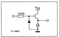
The following equivalent circuit should be applied during filter design :
