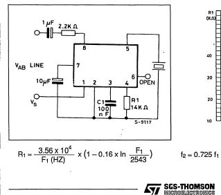
Figure 2 : Typical Application with Balanced Output.
