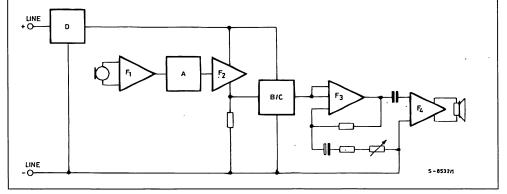
In this case an extra 20 dB amplification is added to the receiving part. A potentiometer provides the possibility of adjusting the gain to the required level.
