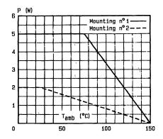
Fig.4 - Power dissipation versus ambient temperature.
