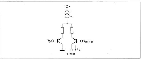
b) When gains have to be related to the voltage at the line terminals of the telephone set, it is necessary to obtain  $V_G$  from a resistive divider directly connected to the end of the line.
