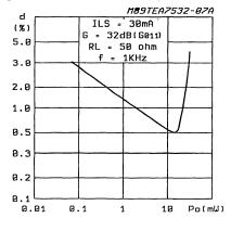
Figure 5 : Distortion Versus Output Power.
