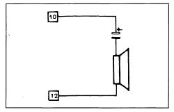
Two loudspeaker connection methods are possible, using the amplifier in either "H" mode or "B" mode.
