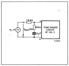
Figure 8 : Test Circuit which does not Activate the Output Signal Generator (see also frequency specification).
