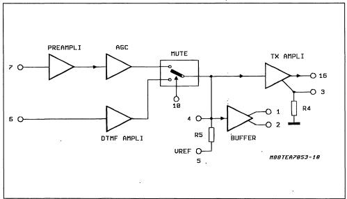
2.1. A.G.C. IN TRANSMISSION. The transmission gain between Microphone Input (pin 7) and Vline (pin 16) is internally decreased of 6dB when the line current varies from 27mA to 42mA with a constant AC load of 600ohms.
