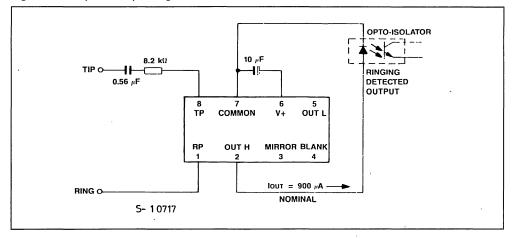
Figure 11 : Typical Application for Opto-isolator Drive.
