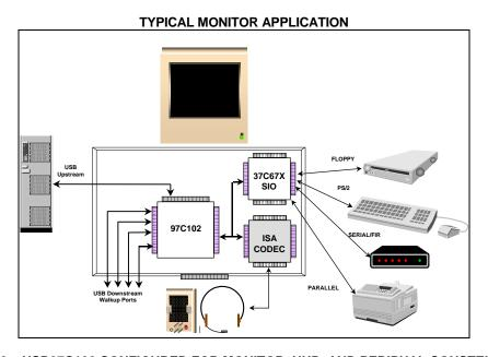
FIGURE 3 – USB97C102 CONFIGURED FOR MONITOR, HUB, AND PERIPHAL CONSTELLATION
