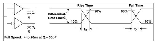
FIGURE 10 - DATA SIGNAL RISE AND FALL TIME
