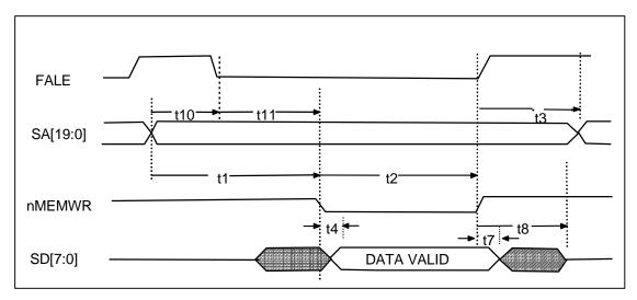
FIGURE 22 - 8051 FLASH MEMORY WRITE TIMING
