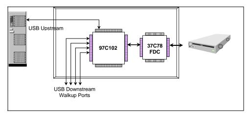
FIGURE 4 – USB97C102 CONFIGURED FOR FLOPPY DRIVE APPLICATION AND WALKUP PORTS
