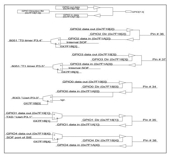
FIGURE 6 - GPIO MUXING BLOCK DIAGRAM
