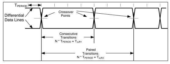
**FIGURE 12 - DIFFERENTIAL DATA JITTER**
