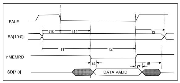
FIGURE 21 - 8051 FLASH MEMORY READ TIMING
