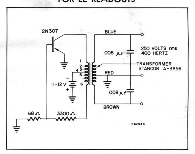
operates from a nominal 12 volt dc source and provides an output of 250 volts RMS, 400 hertz. It has a load rating of 25 ma with a 20% power factor.
