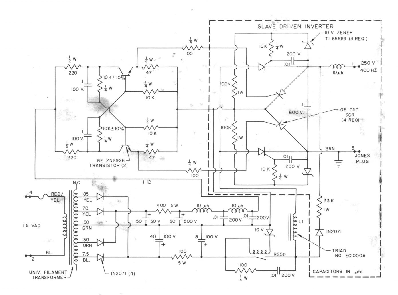
This Sylvania design meets the power requirements for the majority of EL display applications. The unit is made with standard, off-the-shelf components and readily adapts to modular construction. It operates from a 115 Vac, 60 hertz source and has a load rating of 65 ma with a 20% power factor. The design provides essential regulation to assure uniform brightness of the display regardless of the number of EL panels illuminated at any given time within the rating of the supply.
