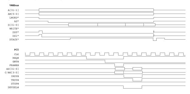
Figure 34: Coupled Read Cycle - Universe II as VME Slave
