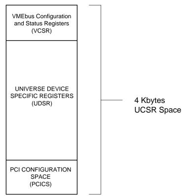
Figure 10: Universe II Control and Status Register Space
