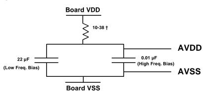
For both schemes, it is recommended that the components involved be tied as close as possible to the associated analog pins.
