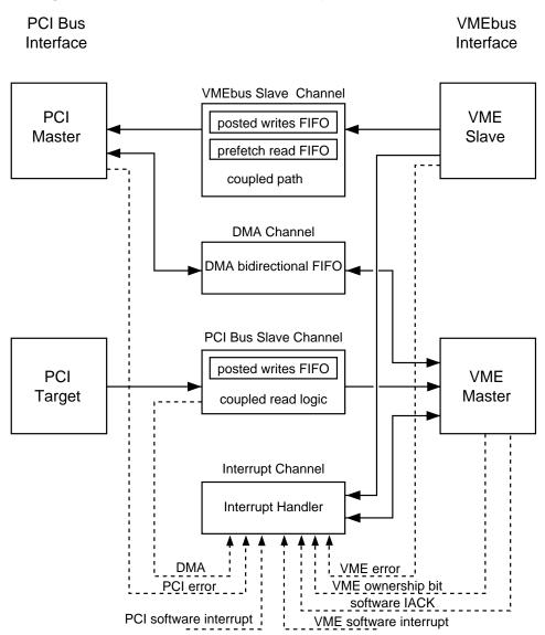
Figure 19: Sources of Internal Interrupts
