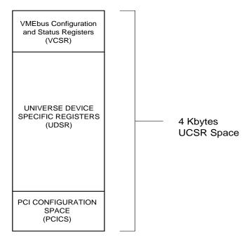
Figure 23: UCSR Access Mechanisms
