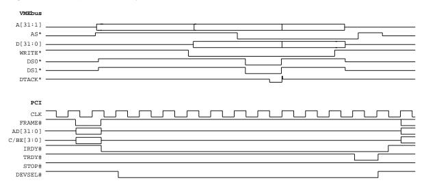
Figure 31: Coupled Write Cycle - Universe II as VME Master
