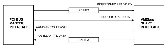
Incoming cycles from the VMEbus can have data widths of 8-bit, 16-bit, 32-bit, and 64-bit. Although the PCI bus supports only two port sizes (32-bit and 64-bit), the byte lanes on the PCI bus can be individually enabled, which allows each type of VMEbus transaction to be directly mapped to the PCI data bus.
