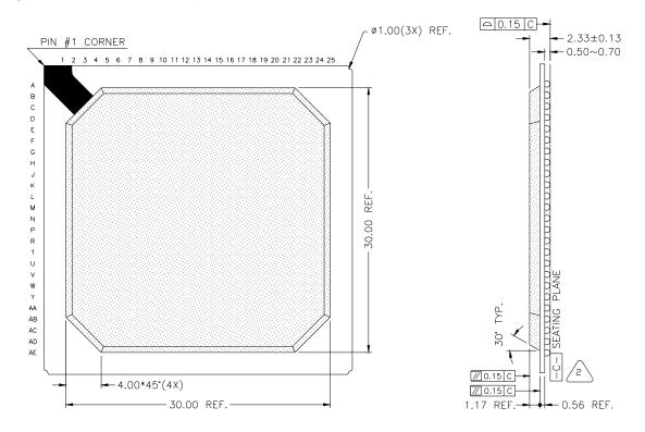
Figure 25: 313 PBGA - Top and Side View
