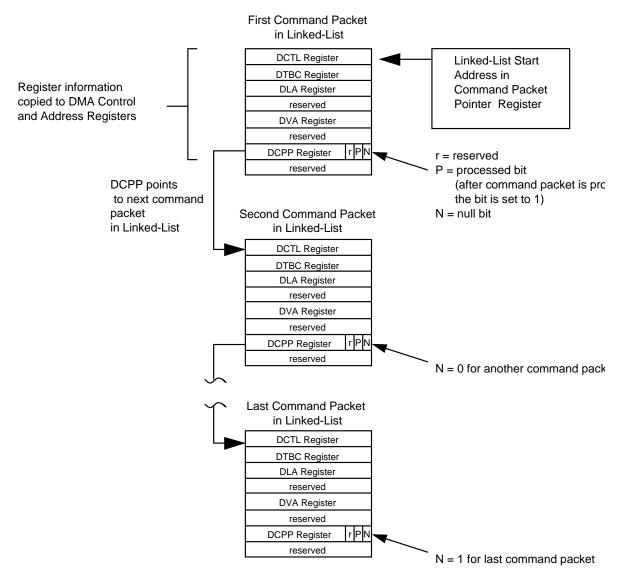
The NULL bit indicates the termination of the entire linked list. If the NULL bit is set to 0, the DMA processes the next command packet pointed to by the command packet pointer. If the NULL bit is set to 1 then the address in the command packet pointer is considered invalid and the DMA stops at the completion of the transfer described by the current command packet.
