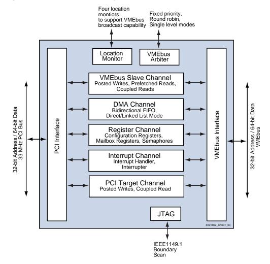
Figure 1: Universe II Block Diagram
