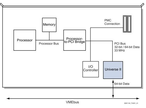
Figure 2: Universe II In Single Board Computer Application
