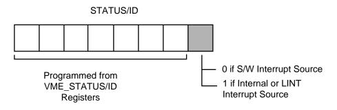
Once the Universe II has provided the STATUS/ID to an interrupt handler during a software initiated VMEbus interrupt, it generates an internal interrupt, SW\_IACK. If enabled, this interrupt feeds back to the PCI bus (through one of the LINT\_ pins) to signal a process that the interrupt started through software has been completed.
