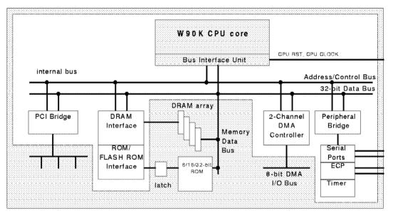
Figure 1.1 shows the system diagram of W90210F.
