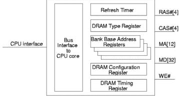
Figure 8.1 DRAM controller block diagram
