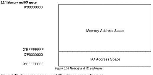
Figure 5.16 shows the memory and I/O address space allocation.Total memory address space available is (4 GB-256 MB). Total addressable I/O space is 256 MB.Program address for I/O:FxxxxxxW90210F CPU core output address:0xxxxxx
