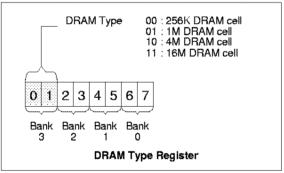
Figure 8.2 DRAM Type register programming
