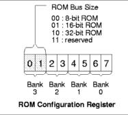
Figure 8.4 ROM configuration register programming
