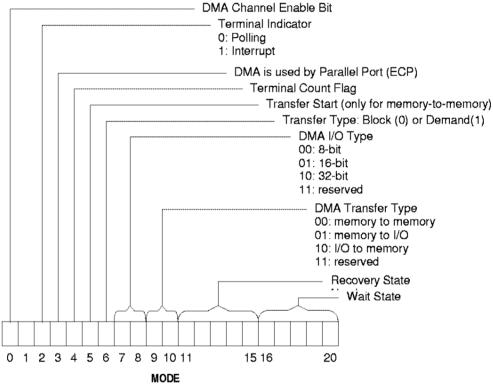
Figure 8.6 Programming DMA controller MODE register
