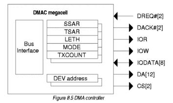
In programming the megacell registers, the register address is defined by the BASE register plus the offset value.
