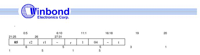
**Purpose:** To multiply two unsign 32-bit word of GR[r1] and GR[r2], then add accumulate register {HI, LO} with the multiplied result.
