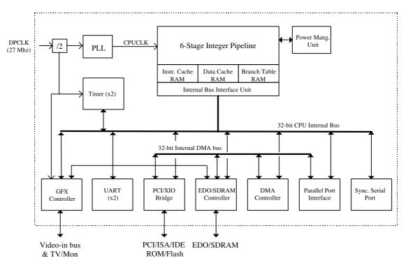
Fig 1-1 : W90221 Internal Block Diagram
