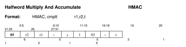
**Purpose:** To multiply two signed 16-bit halfword of GR[r1] register and GR[r2] register, then accumulate {HI, LO} register with the multiplied result.
