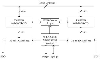
Fig 5.1.6-1 SSI Block Diagram
