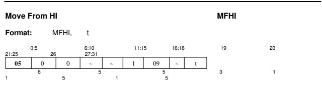
Purpose: To move the high-order 32-bits of the accumulator HI into a general register GR[t].
