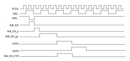
Fig5.12.1 Timer register write command when the osilattor frequence is slower the cpu frequency
