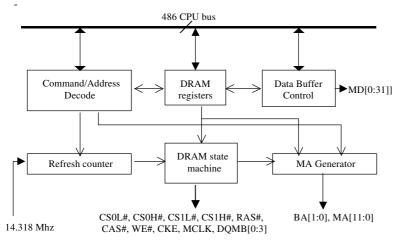
Fig 5.4-1 MEMC Block Diagram
