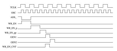
Fig5.12.1 Timer register write commandwhen the osilattor frequence is faster the cpu frequency
