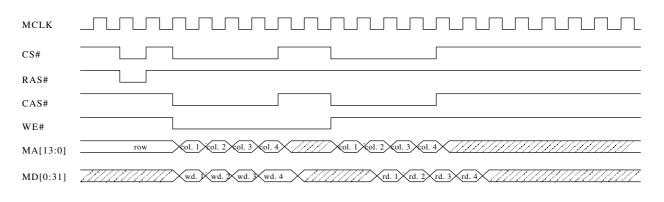
Fig 5.4.4 Fastest SDRAM memory write/read cycle (32 bits)
