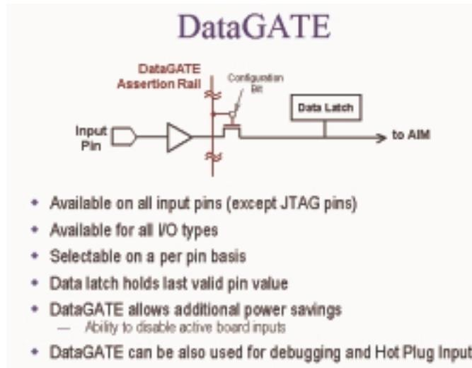
FIGURE 2-34: DATA GATE FUNCTION IN COOLRUNNER-II CPLDs
