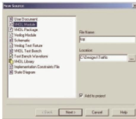
FIGURE 4-25: NEW SOURCE WINDOW SHOWING VHDL MODULE
