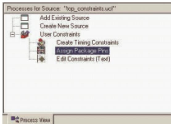
FIGURE 5-3: ASSIGN PACKAGE PINS IN PACE TOOL
