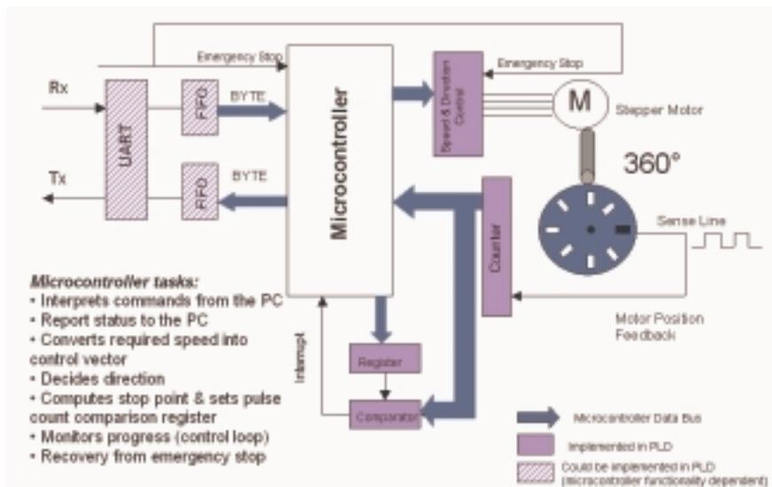
FIGURE 7-7: PARTITIONED DESIGN: MICROCONTROLLER AND CPLD
