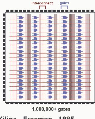
FIGURE 1-4: FPGA ARCHITECTURE
