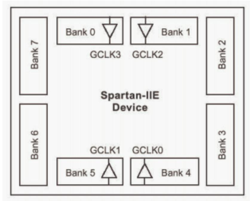
FIGURE 2-11: SPARTAN-IIIE BANKING OF I/O STANDARDS
