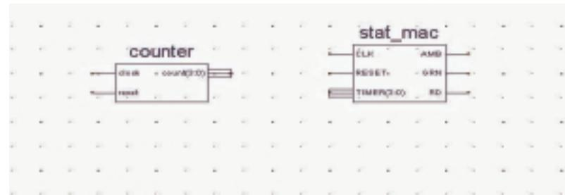
FIGURE 4-34: CLOSE-UP OF COUNTER AND STATE MACHINE SYMBOLS
