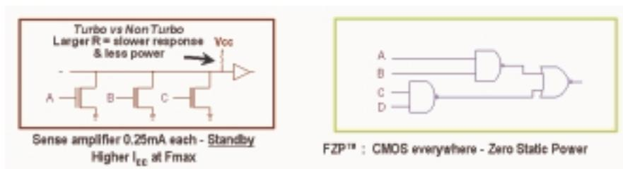
FIGURE 2-21: SENSE AMPLIFIER VS. CMOS CPLDs
