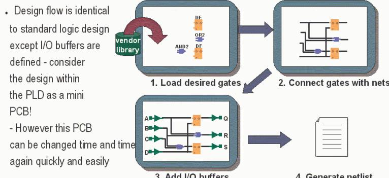
FIGURE 1-7: PLD DESIGN FLOW
