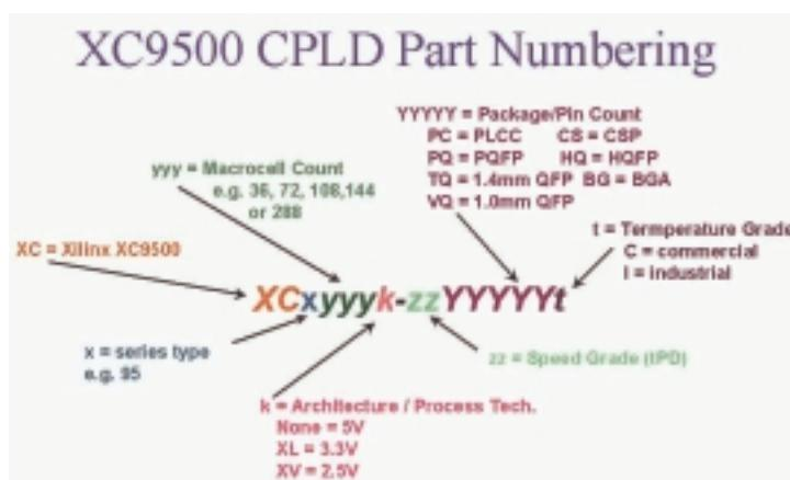
FIGURE 2-20: XC9500 PART NUMBERING SYSTEM
