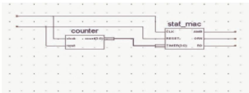
FIGURE 4-35: COUNTER AND STATE MACHINE SYMBOLS WITH WIRE
