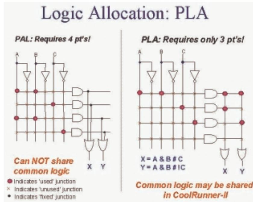
FIGURE 2-31: LOGIC ALLOCATION – TYPICAL PAL vs. PLA
