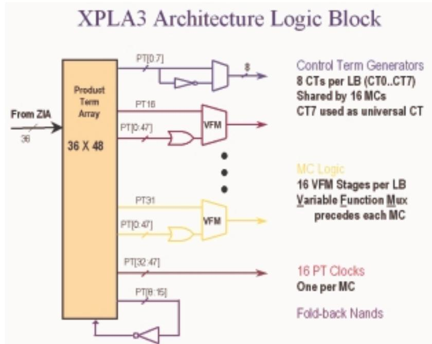
FIGURE 2-24: COOLRUNNER XPLA3 LOGIC BLOCK
