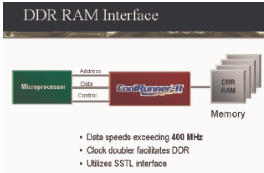
FIGURE 2-39: DDR RAM INTERFACE EXAMPLE
