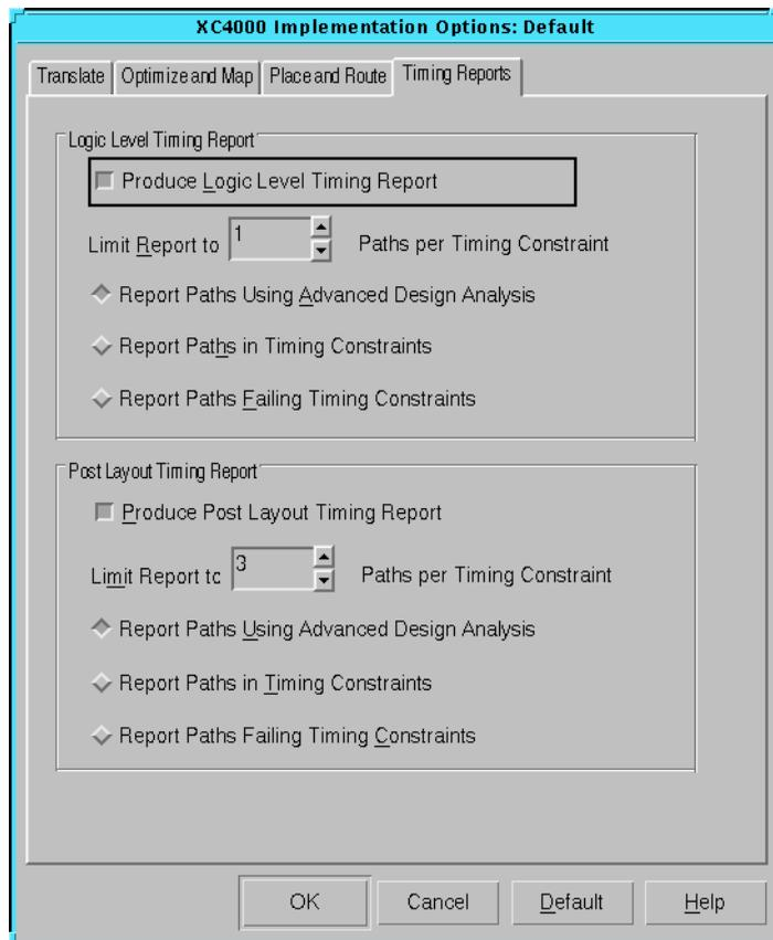
**Figure 4-11** Setting the Produce Logic Level Timing Report Option
