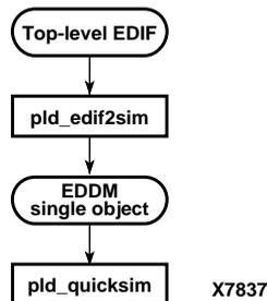
**Figure 3-15** EDIF Functional Simulation Flow
