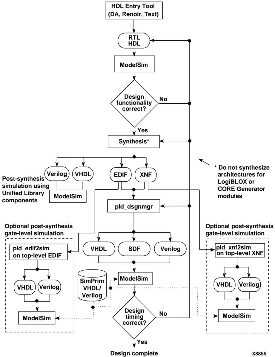
Figure 7-5 Pure VHDL/Verilog Design Flow
