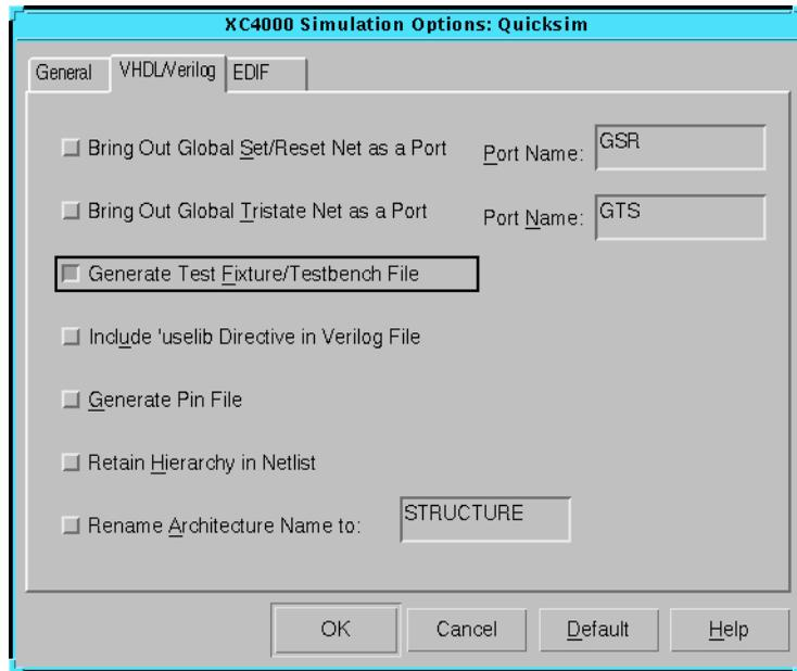
**Figure 5-12 VHDL/Verilog Pane of Simulation Options Dialog Box**
