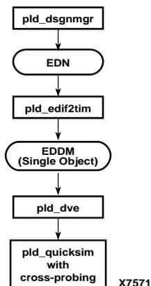
Figure 3-25 Timing Simulation for Schematics
