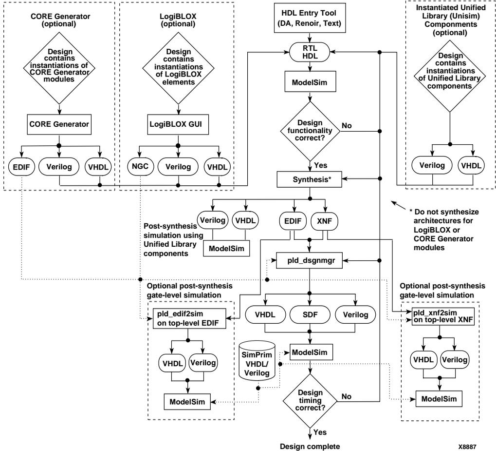
Figure 1-5 HDL (Verilog/VHDL) Design Entry and Synthesis
