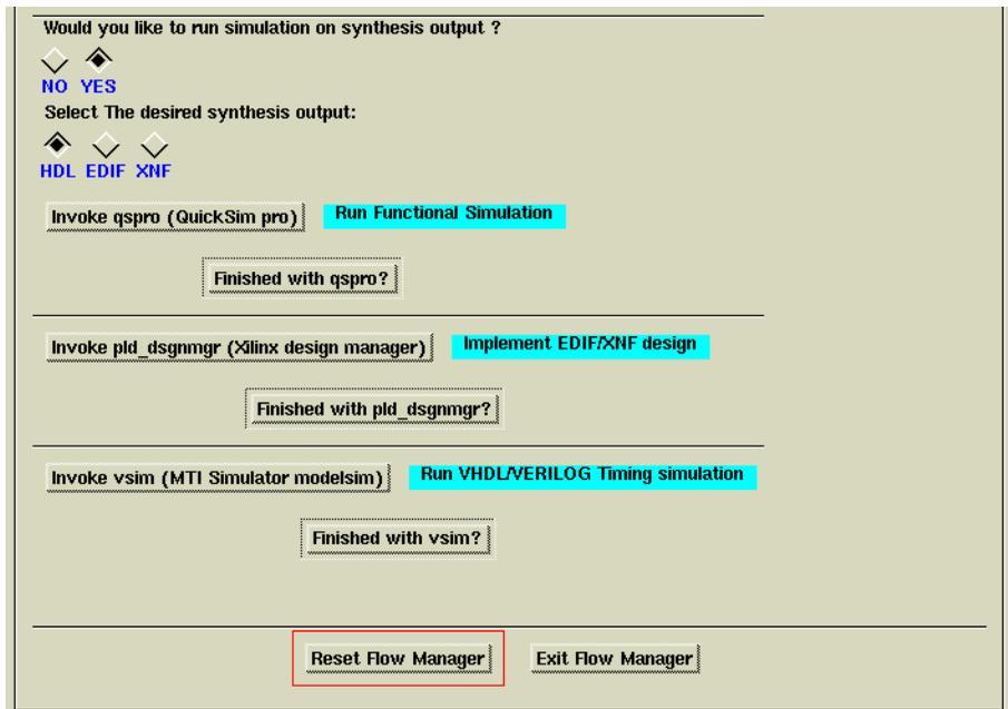
Figure 7-13 Run Simulation on HDL Synthesis Output
