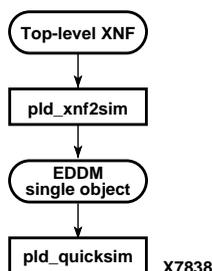
Figure 3-13 XNF Functional Simulation Flow
