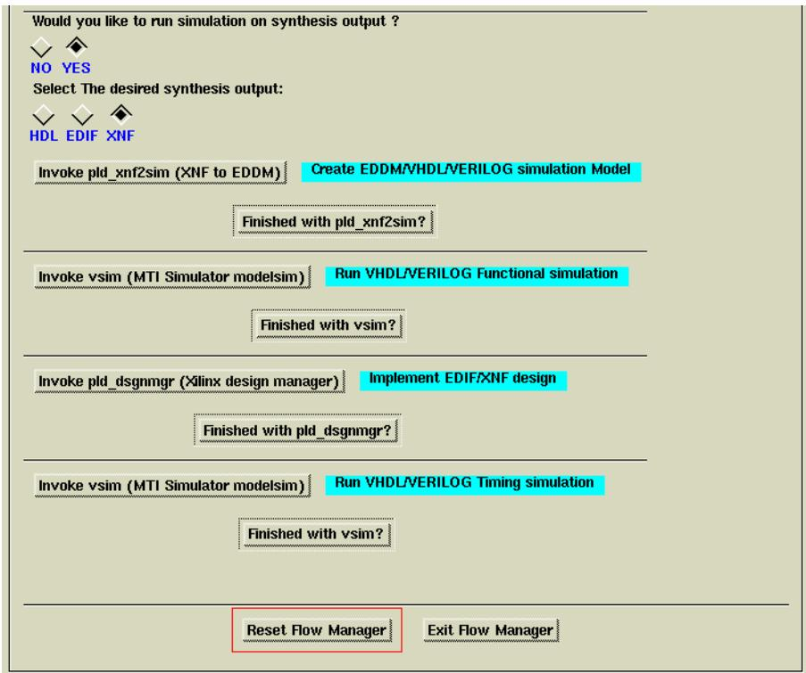
Figure 7-15 Run Simulation on XNF Synthesis Output
