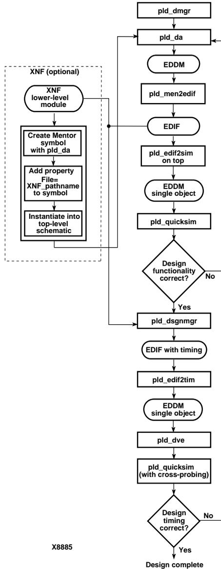
Figure 1-4 Schematic Design Entry with XNF Module
