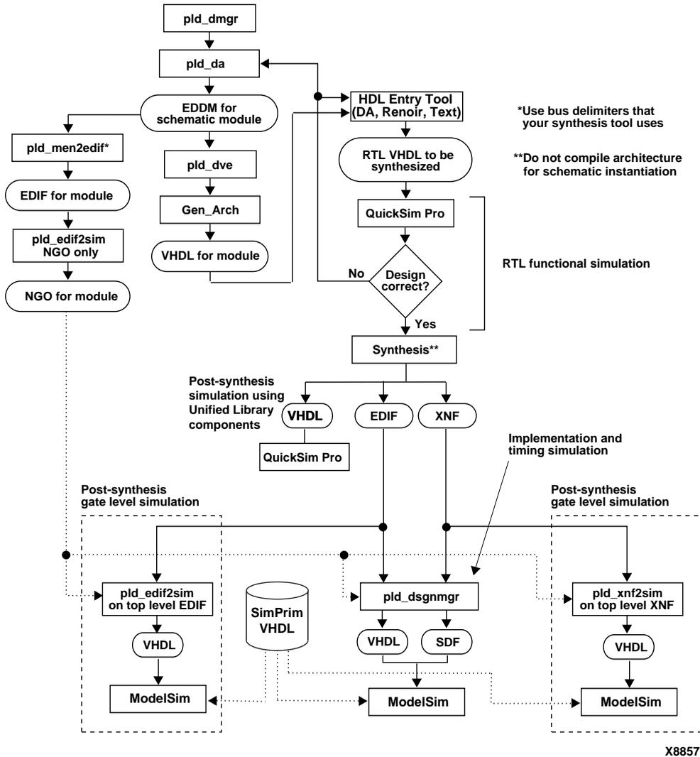
Figure 7-10 Mixed Designs with HDL on Top Design Flow
