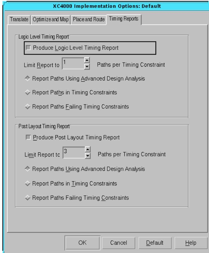
**Figure 3-23** Setting the Produce Logic Level Timing Report Option
