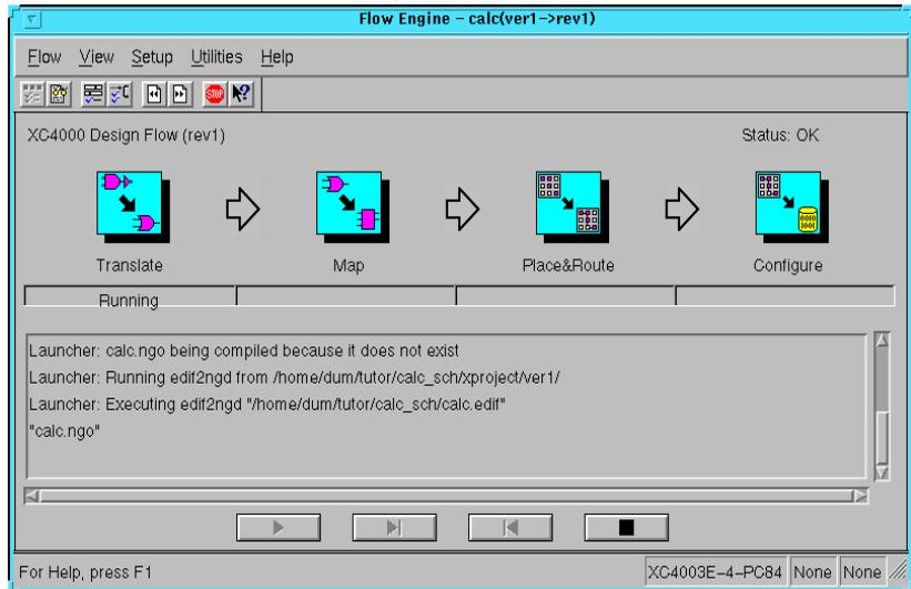
**Figure 5-14 The Xilinx Flow Engine**
