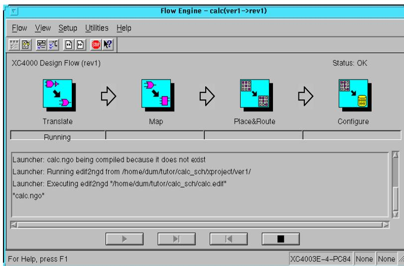
**Figure 4-12 The Xilinx Flow Engine**
