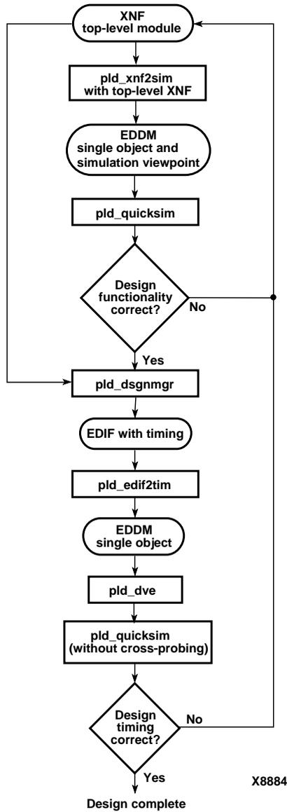
Figure 1-3 Design Entry with XNF Top-Level Module
