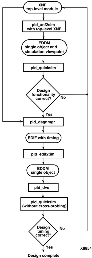
Figure 7-3 Pure XNF Design Flow
