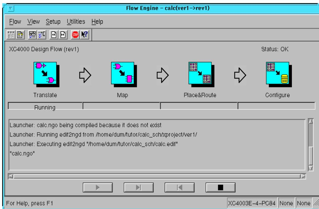
**Figure 3-24 The Xilinx Flow Engine**
