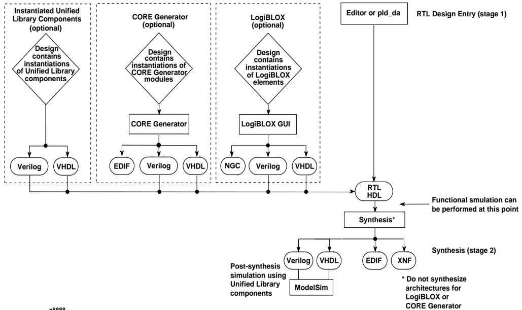
**Figure 4-2 HDL (Verilog/VHDL) Design Entry and Synthesis**
