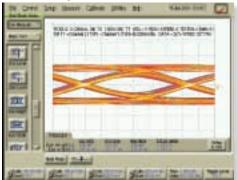
Figure 5 -Received signals after 50 inches FR-4 PC board material with no pre-emphasis and with 30% pre-emphasis in the Rocket I/O MGT.
