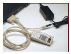
Parallel Cable IV connected to external power supply
