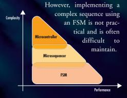
Figure 1 - Performance versus functional complexity Microcontrollers are commonly used to implement complex protocols. However, they require substantial resources (memory, cost, pins, ...), which can be difficult to justify in real-life situations. On the other hand, software implementations allow designers to cope with mounting logic complexity. They are easy and quick to implement and easier to maintain.
