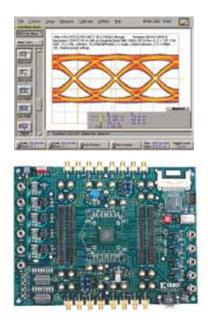
Figure 3 - RocketIO characterization using ML320 hardware platform: eye diagram at receiver shows 3.125 Gbps on 44-inch FR4, two connectors with 33% pre-emphasis.
