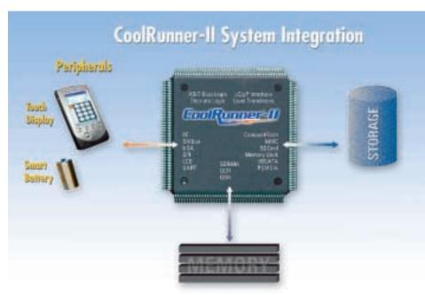
Figure 2 - Multiple functions in a single CPLD
