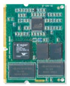
Figure 4 - Virtex XC2V1000 implemented on Hitachi SH4 µEngine
