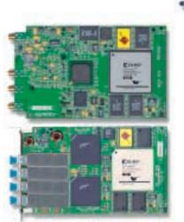
Figure 2 - WILDSTAR II for VME with 1.5 GHz A/D and Fibre Channel 2 I/O cards
