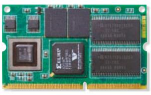
Figure 3 - Hitachi SH3 µEngine with Virtex XCV100
