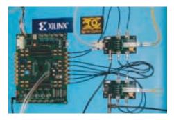
Figure 1 - Four RocketIO channels at 2.488 Gbps with Ignis Optics' four IGP-2000 OC-48 SFP optical transceivers
