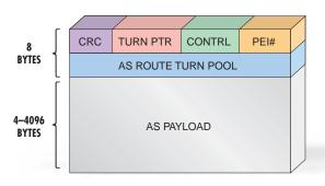
Figure 2 – AS transaction layer packet
