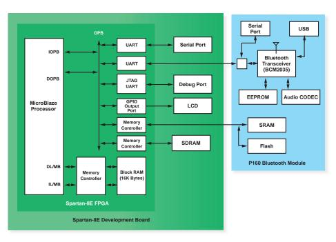
Figure 4 – Typical MicroBlaze-based system
