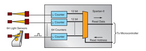
Figure 5 – Light sensors collect data for processing.
