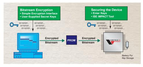
Figure 3 – Design security in Virtex-II Pro FPGAs using Triple DES encryption/decryption
