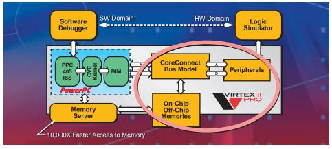
Figure 2 – The Seamless Co-Verification Environment connects hardware and software verification environments for Virtex-II Pro FPGAs.
