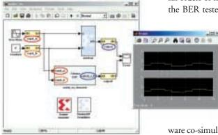
Figure 6 – Co-simulation block parameterized with port names that match the original model.
