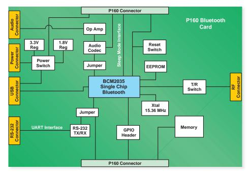
Figure 3 – P160 Bluetooth Module functional diagram
