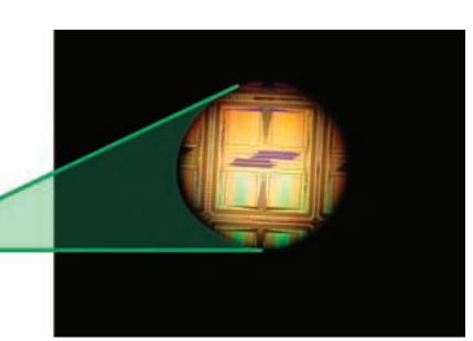
them, as well as charge pumping. In addition, four or five layers of metal (Figure 2) rule out direct exposure of top die to laser/electrical tampering.
