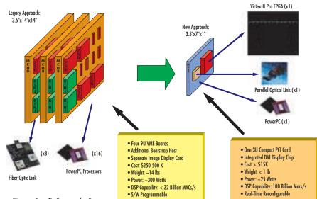
Figure 2 – Before and after Virtex-II Pro implementation
