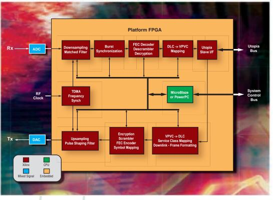
Figure 1 – Access-point transceiver for ETSI-compliant BRAN PHY layer
