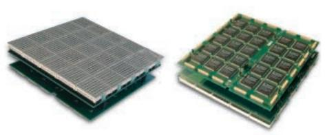
Figure 3 – Front and back view of 25 FPGAs assembled on a BioWall panel
