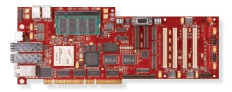
Figure 1 – Avnet-designed Virtex-II Pro XC2VP20 development board
