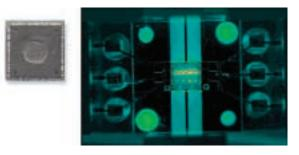
Figure 1 - An attacker can extract nonvolatile device die from a chip package and find security bits using thermal imaging.
