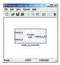
Figure 5 – Co-simulation library – cosim\_ex\_hwcosim\_lib – created by the post-generation script.
