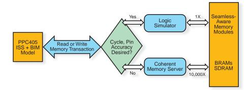
Figure 3 – The Seamless coherent memory server accelerates co-simulation with faster access to memory.
