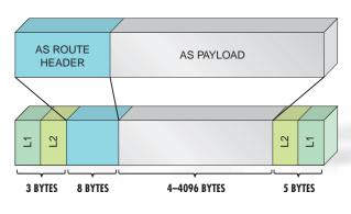
Figure 3 – AS transaction layer frame
