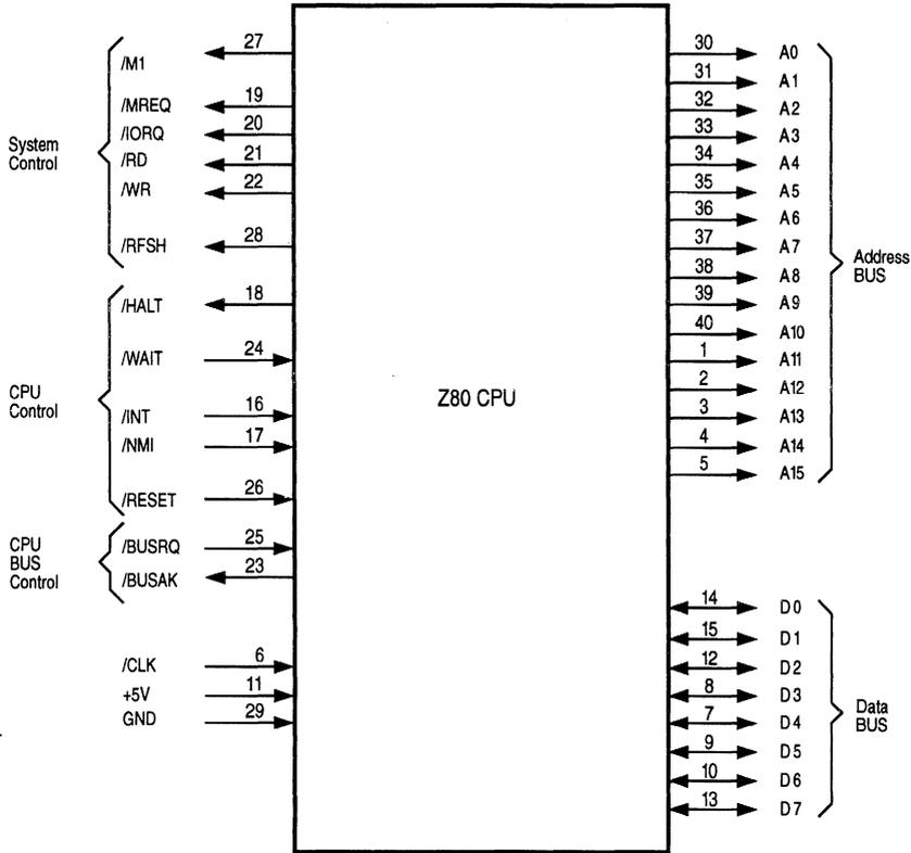
Figure 2.1 Z80 Pin Configuration
