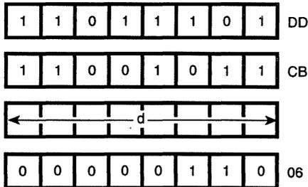
**Description:** The contents of the memory address specified by the sum of the contents of the Index Register IX and a two's complement displacement integer d, are rotated left 1-bit position. The content of bit 7 is copied into the Carry flag and also, into bit 0. Bit 0 is the least significant bit.
