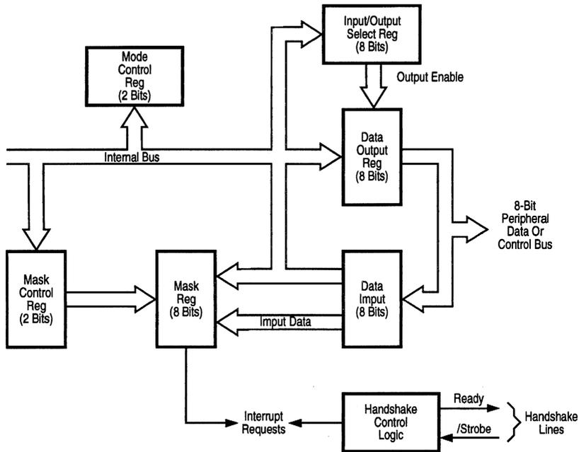
Figure 2-2. Port I/O Block Diagram
