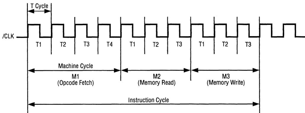
Figure 3-1. Basic CPU Timing Example
