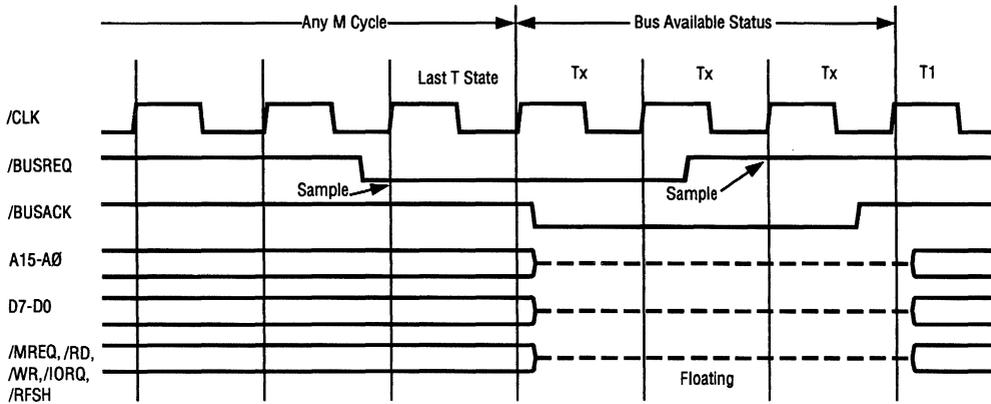
Figure 3-5. Bus Request/Acknowledge Cycle
