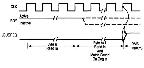
**Figure 8-10. Bus Release on Match (Burst and Continuous Modes)**
