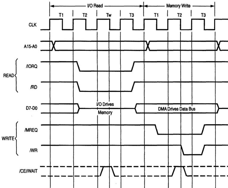
Figure 8-4. Sequential I/O-to-Memory Transfer, Standard Timing (Searching Is Optional)
