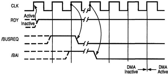
**Figure 8-7. Bus Request and Acceptance Timing**
