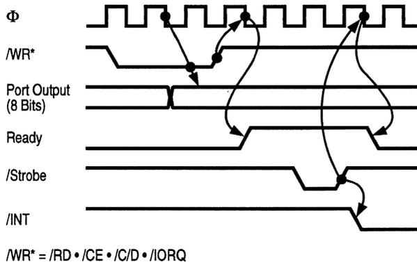
Figure 5-1. Mode 0 (Output) Timing
