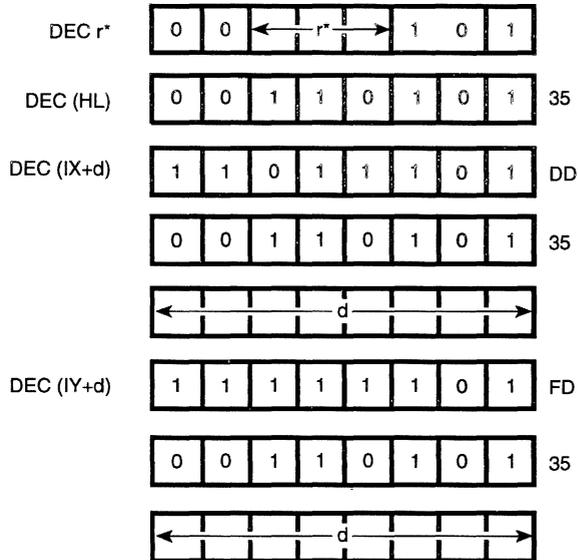
\*r identifies registers B, C, D, E, H, L, or A assembled as follows in the object code field above:
