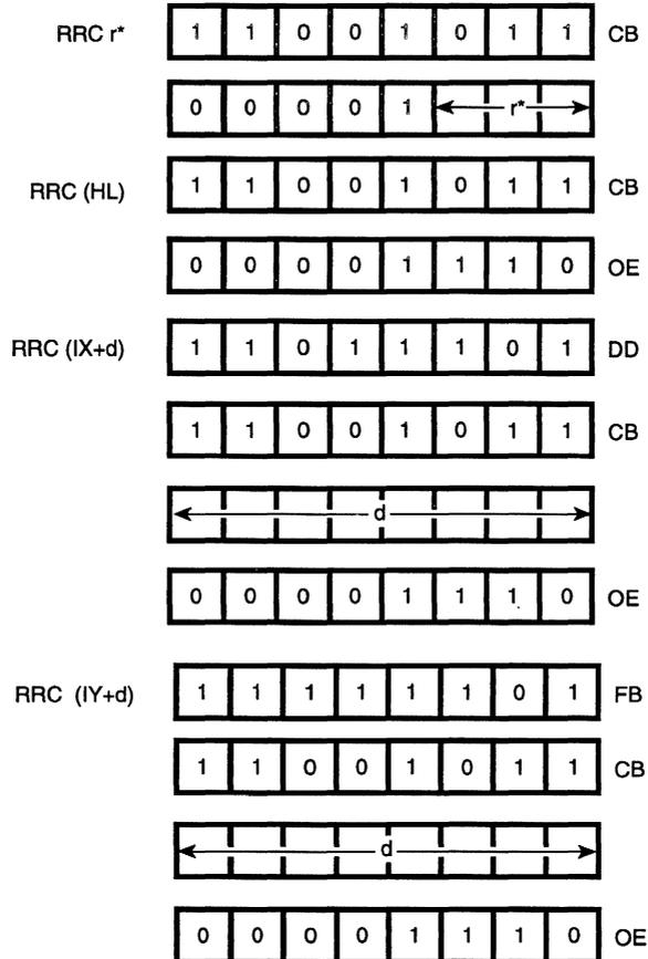
\*r identifies registers B, C, D, E, H, L, or A specified as follows in the assembled object code above:
