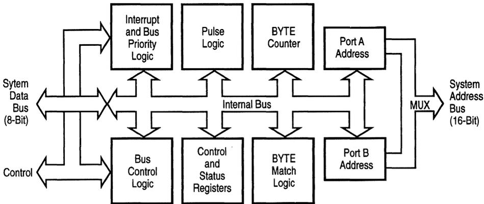
Figure 4-1. Z80 DMA Block Diagram
