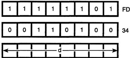
**Description:** The contents of the Index Register IY (register pair IY) are added to a two's complement displacement integer *d* to point to an address in memory. The contents of this address are then incremented.
