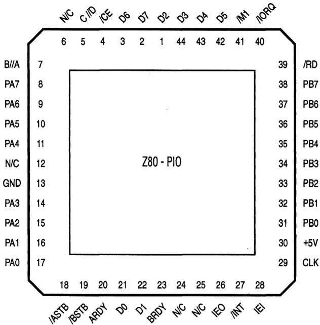
Figure 3-2. PIO 44-Pin PLCC Pin Assignments
