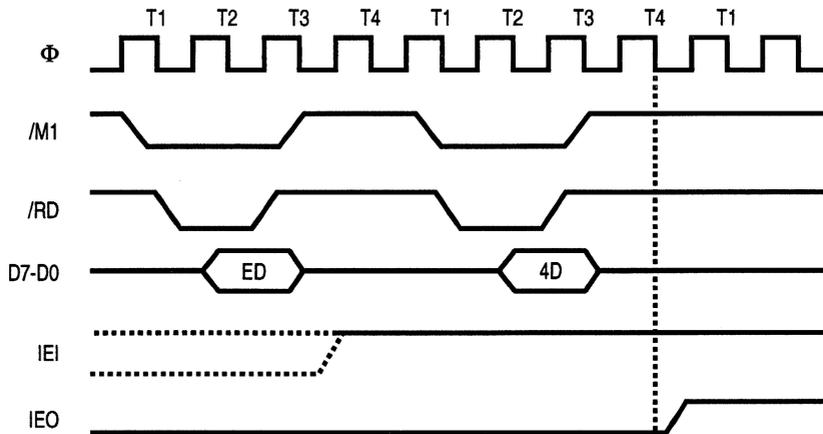
Figure 9-4. Return From Interrupt Cycle Timing
