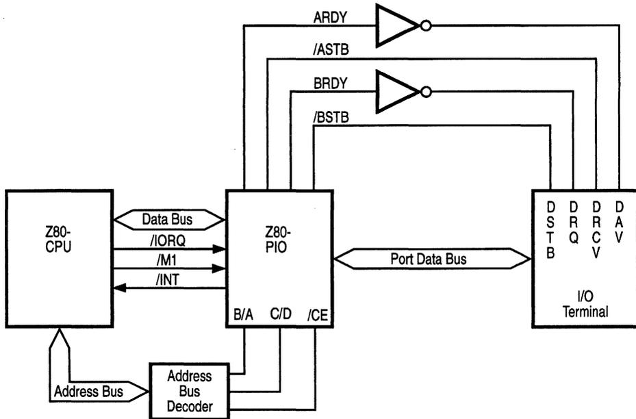
Figure 7-2. Example of I/O Interface
