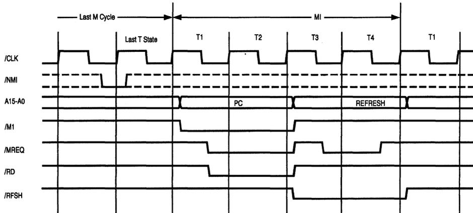
Figure 3-7. Non-Maskable Interrupt Request Operation
