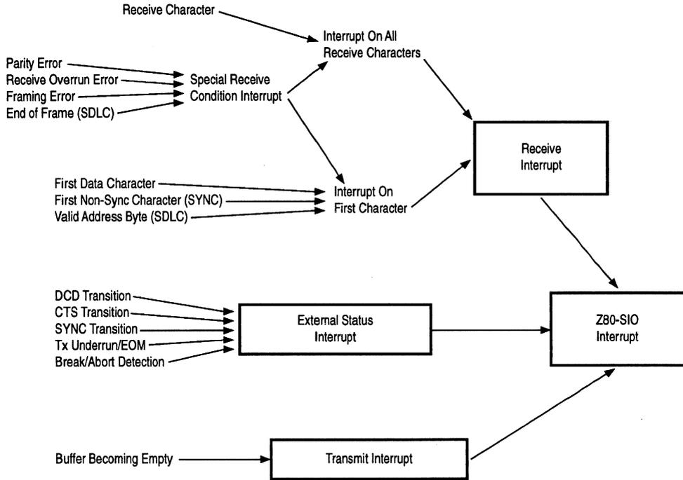
Figure 3-2. Interrupt Structure
