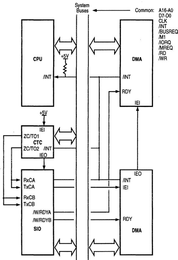
Figure 6-8. Z80 DMA-SIO Environment
