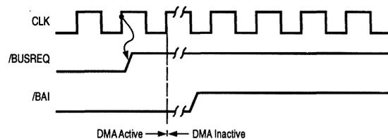
**Figure 8-8. Bus Release in Byte Mode**
