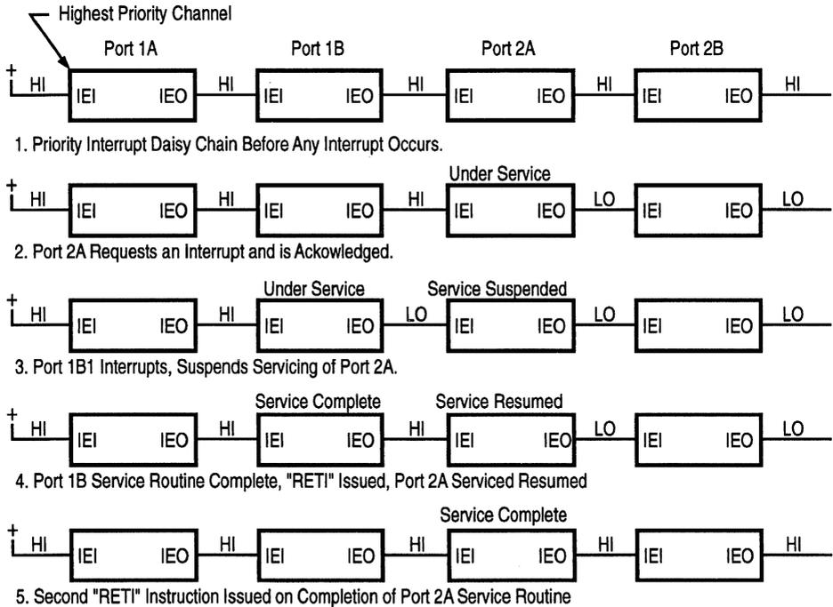
Figure 6-3. Daisy-Chain Interrupt Servicing
