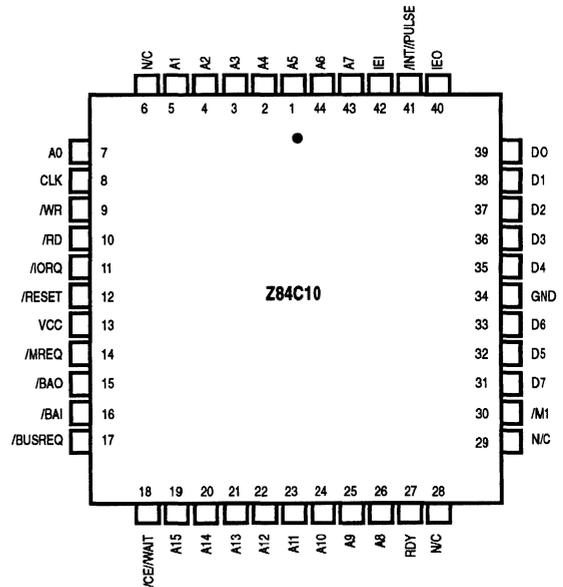
Figure 3-4. 44-Pin PLCC Pin Assignments (Z84C10 CMOS)
