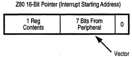
**Figure 2-5. Z80 16-Bit Pointer (Interrupt Starting Address)**
