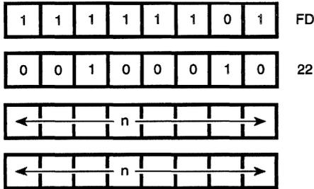
**Description:** The low order byte in Index Register IY is loaded into memory address (nn); the upper order byte is loaded into memory location (nn+1). The first n operand after the opcode is the low order byte of nn.
