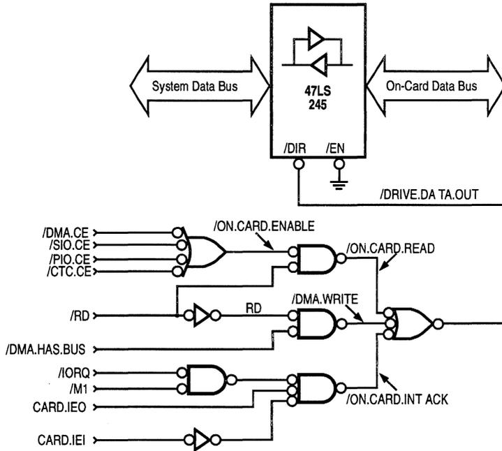
Figure 6-7. Data Bus Buffer Control Example
