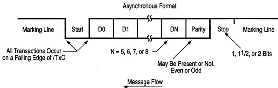
Figure 4-1. Asynchronous Message Format
