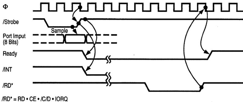
Figure 5-2. Mode 1 (Input) Timing
