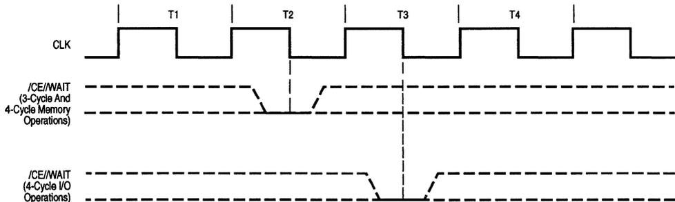
Figure 8-16. /WAIT Line Sampling in Variable-Cycle Timing
