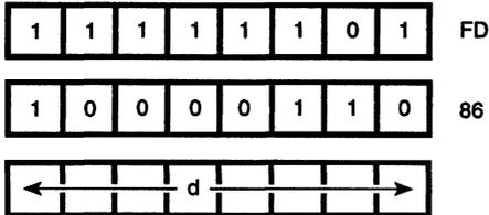
**Description:** The contents of the Index Register (register pair IY) is added to a two's complement displacement *d* to point to an address in memory. The contents of this address is then added to the contents of the Accumulator, and the result is stored in the Accumulator.
