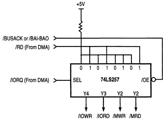
**Figure 6-4. Simultaneous Transfer Multiplexer**
