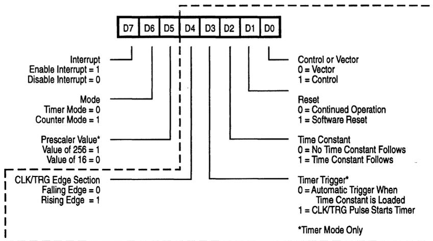
Figure 5-1. Channel Control Register
