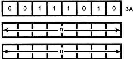
**Description:** The contents of the memory location specified by the operands nn are loaded into the Accumulator. The first n operand after the opcode is the low order byte of a 2-byte memory address.
