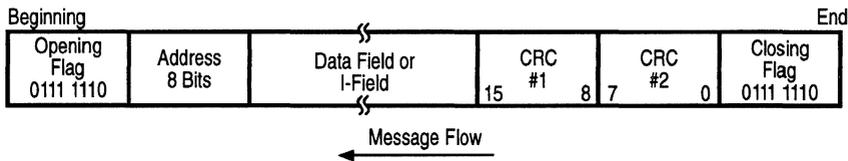
**Figure 6-1. Transmit/Receive SDLC/HDLC Message Format**
