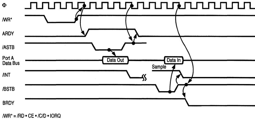
Figure 5-3. Port A, Mode 2 (Bidirectional) Timing
