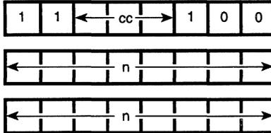
Note: The first of the two n operands in the assembled object code above is the least significant byte of the 2-byte memory address.
