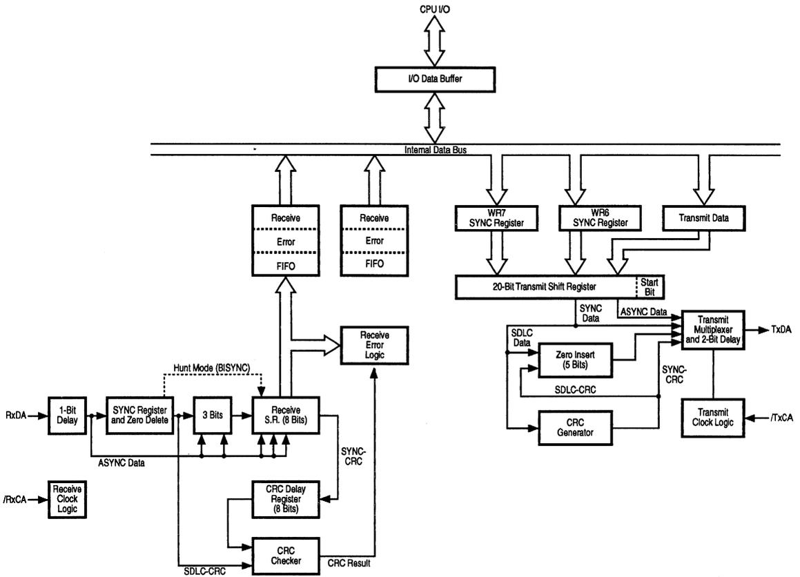
Figure 3-1. Transmit and Receive Data Path
