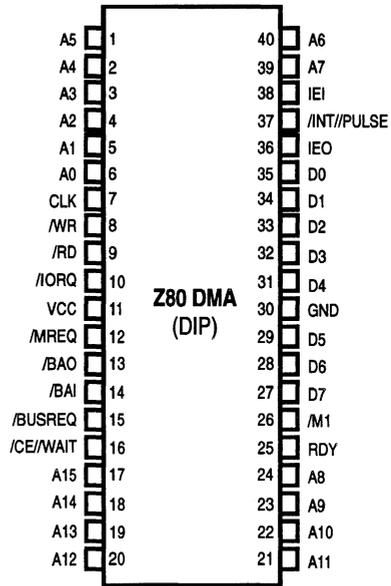
Figure 3-2. 40-Pin DIP Pin Assignments
