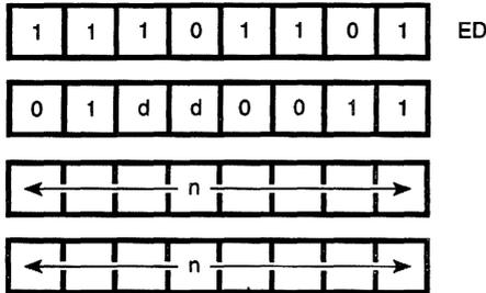
**Description:** The low order byte of register pair dd is loaded into memory address (nn); the upper byte is loaded into memory address (nn+1). Register pair dd defines either BC, DE, HL, or SP, assembled as follows in the object code:
