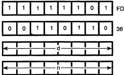
**Description:** Integer n is loaded into the memory location specified by the contents of the Index Register summed with the two's complement displacement integer d.
