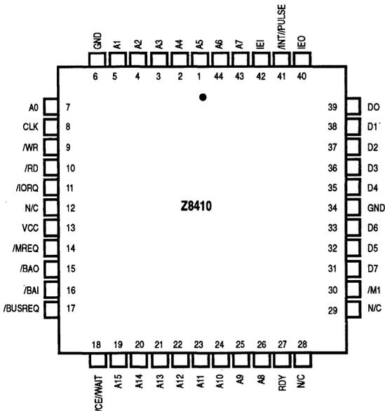
Figure 3-3. 44-Pin PLCC Pin Assignments (Z8410 NMOS)
