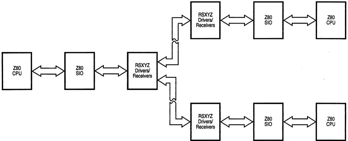
**Figure 8-1. Synchronous/Asynchronous Processor-to-Processor Communication (Direct Wire to Two Remote Locations)**
