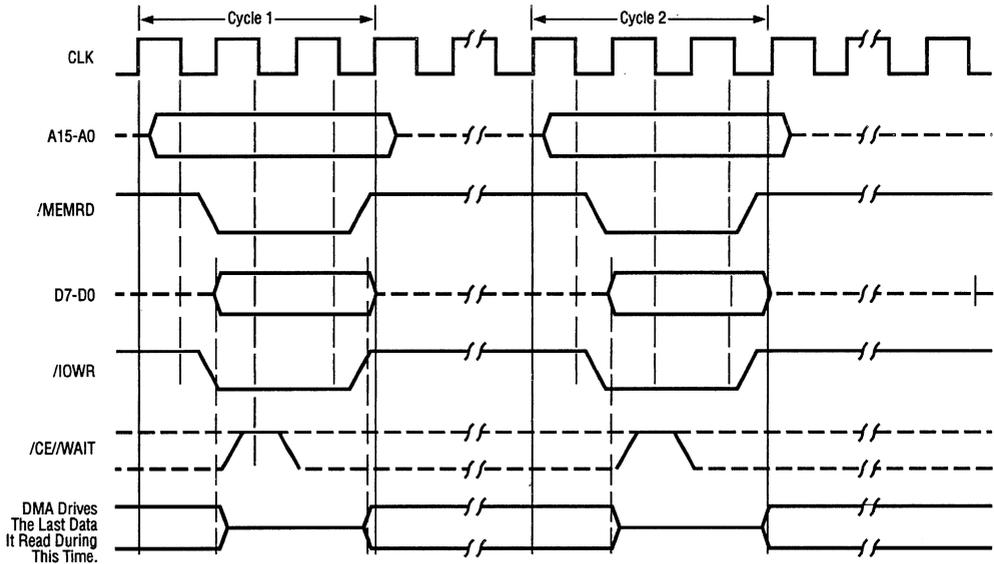
Figure 8-6. Simultaneous Memory-to-I/O Transfer (Byte Mode)
