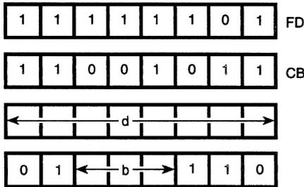
**Description:** This instruction tests bit b in the memory location specified by the content of register pair IY combined with the two's complement displacement d and sets the Z flag accordingly. Operand b is specified as follows in the assembled object code.
