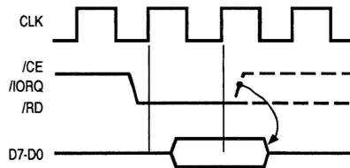
Figure 8-2. CPU-to-DMA Read Cycle Requirements
