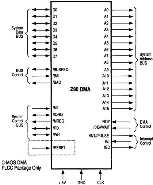
Figure 3-1. Pin Functions
