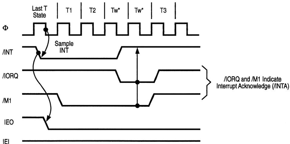
Figure 6-1. Interrupt Acknowledge Timing
