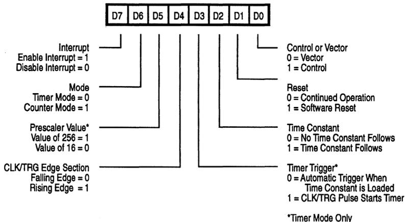
Figure 2-3. Channel Control Register
