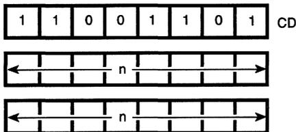
Note: The first of the two n operands in the assembled object code above is the least significant byte of a 2-byte memory address.
