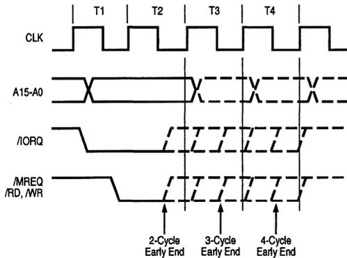
Figure 8-15. Variable-Cycle and Edge Timing
