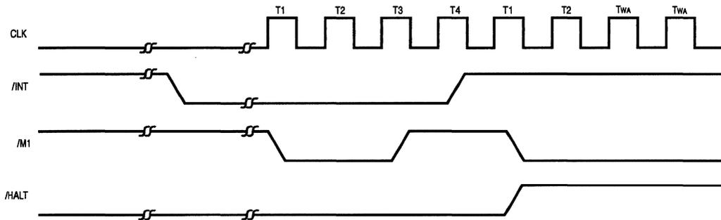
Figure 3-12. Power-Down Release Cycle No. 3
