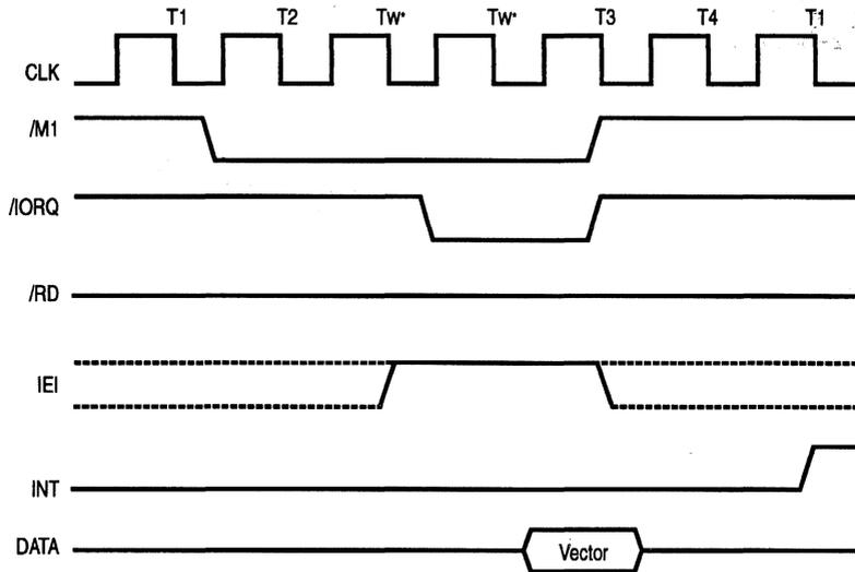
Figure 7-1. Interrupt Acknowledge Cycle
