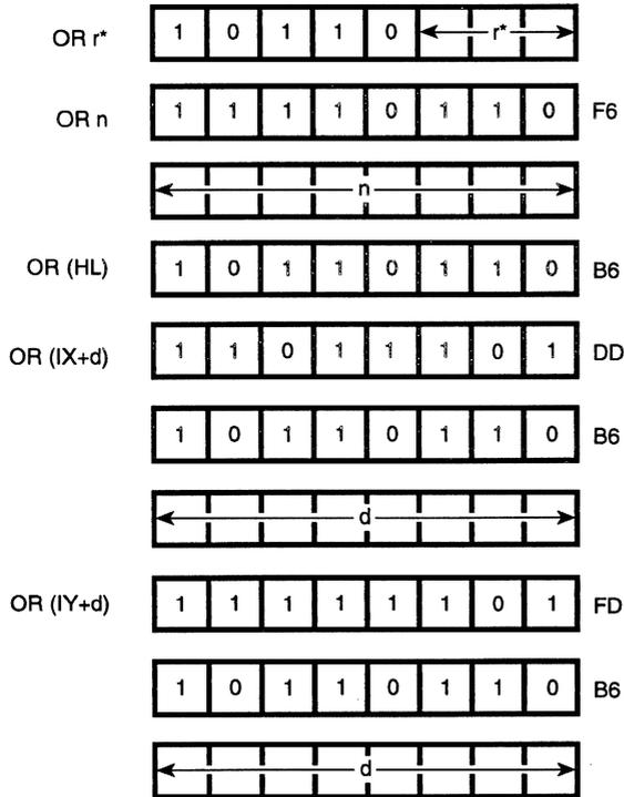
\*r identifies registers B, C-, D, E, H, L, or A specified as follows in the assembled object code field above:
