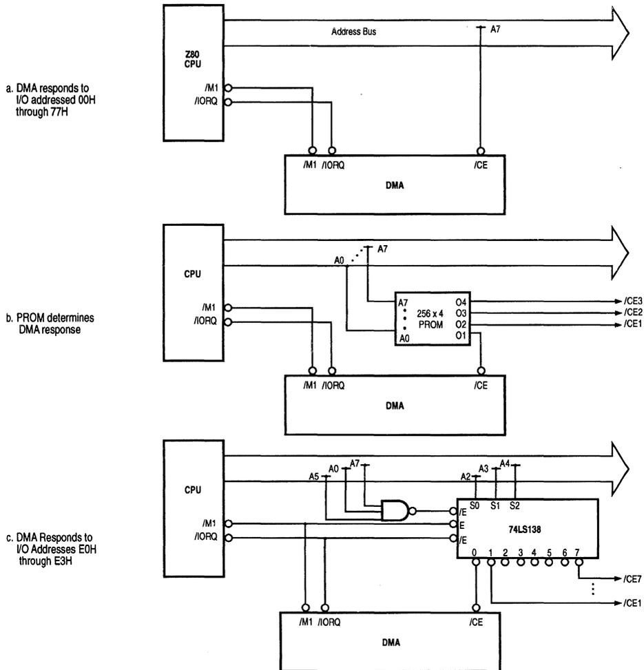
Figure 6-2. Chip Enable Decoding with Z80 CPU
