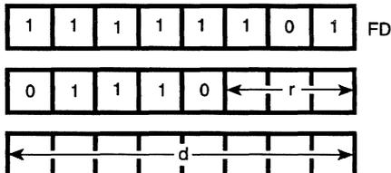
**Description:** The contents of register r are loaded into the memory address specified by the sum of the contents of the Index Register IY and d, a two's complement displacement integer. The symbol r is specified according to the following table.
