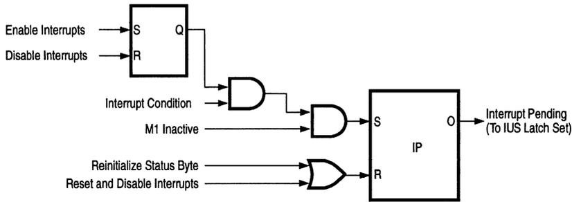
\*NOTE: Interrupt conditions can include end-or-block, byte match or active RDY line, depending on programming.
