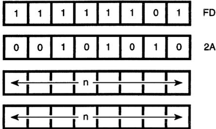
**Description:** The contents of address (nn) are loaded into the low order portion of Index Register IY, and the contents of the next highest memory address (nn+1) are loaded into the high order portion of IY. The first n operand after the opcode is the low order byte of nn.
