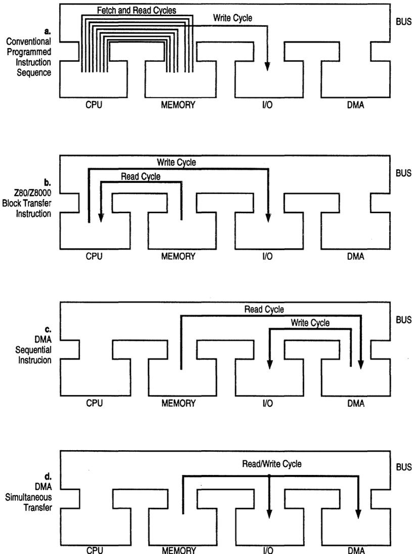
Figure 1-2. Conceptual Comparison of Various I/O Transfer Methods
