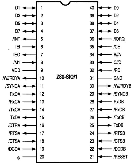
Figure 2-3. Z80-SIO/1 Pin Functions
