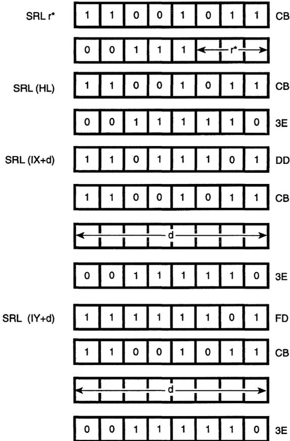
\*r identifies registers B, C, D, E, H, L, or A specified as follows in the assembled object code fields above:
