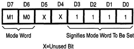
Bits D7 and D6 from the binary code for the desired mode according to the following table:
