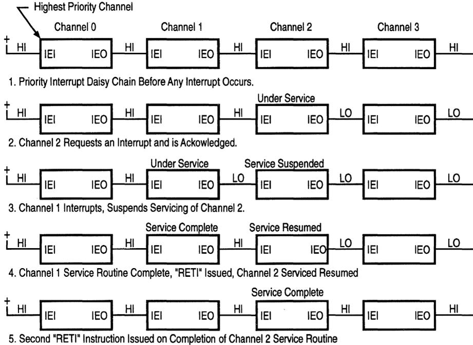
Figure 7-3. Daisy-Chain Interrupt Servicing
