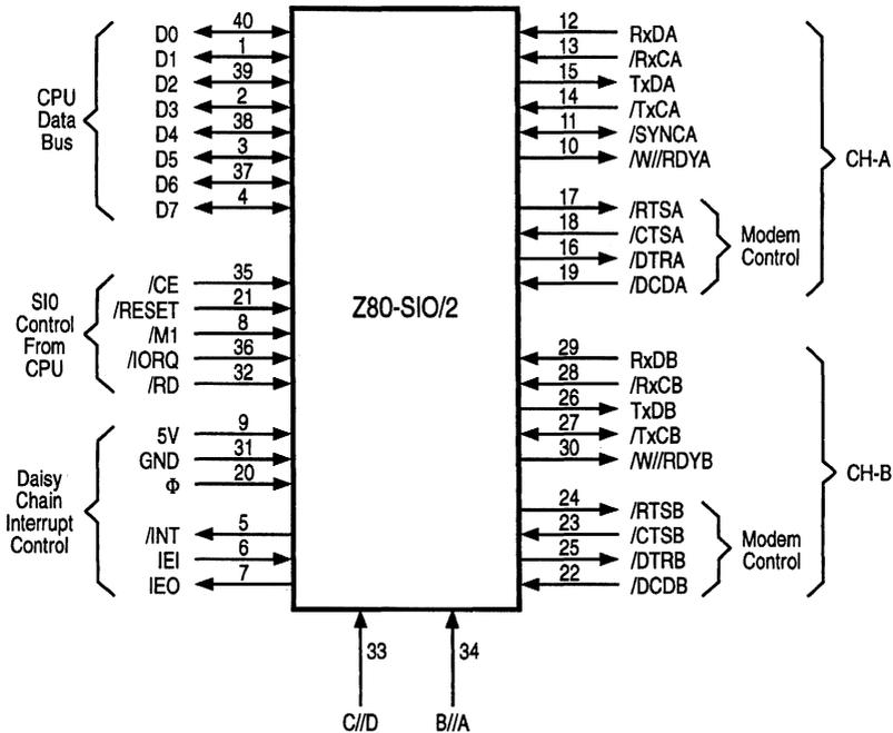
Figure 2-6. Z80-ZIO/2 Pin Assignments
