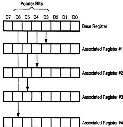
Figure 5-1. Method of Write-Register Pointing
