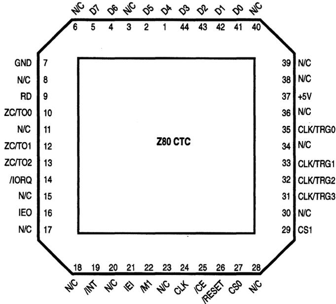
Figure 3-3. 44-pin Chip Carrier Pin Assignments
