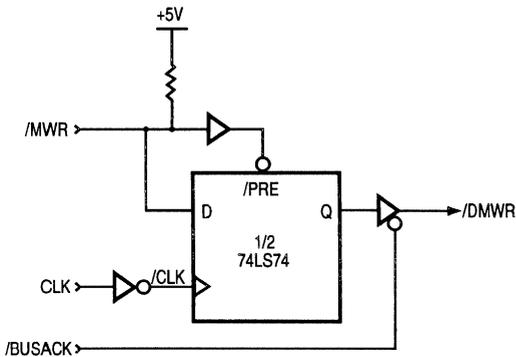
Figure 6-6. Delaying the Leading Edge of /MWR
