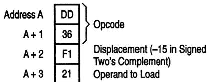
Notice that with any indexed addressing the displacement always follows directly after the opcode.
