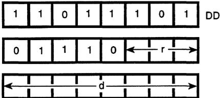
**Description:** The contents of register r are loaded into the memory address specified by the contents of Index Register IX summed with d, a two's complement displacement integer. The symbol r identifies register A, B, C, D, E, H, or L, assembled as follows in the object code:
