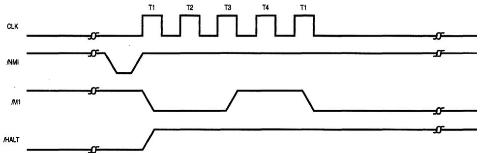
**Figure 3-10. Power-Down Release Cycle No. 1**
