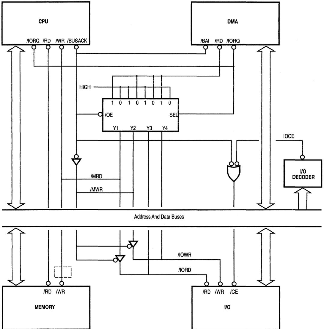
Figure 6-5. Simultaneous Transfer
