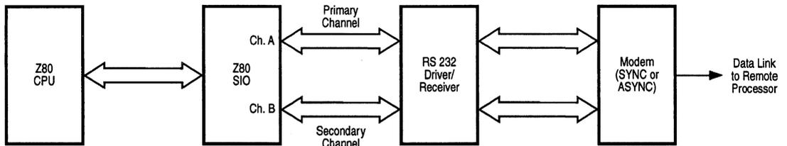
**Figure 8-2. Synchronous/Asynchronous Processor-to-Processor Communication (Using Telephone Line)**
