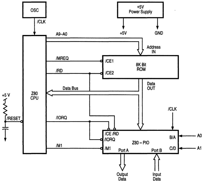
Figure 7-1. Minimum Z80 Computer System
