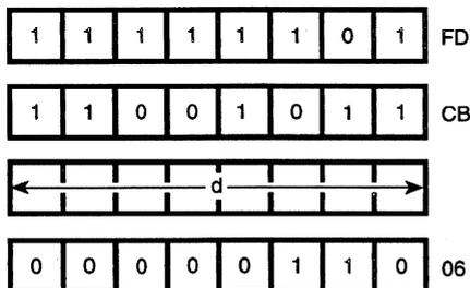
**Description:** The contents of the memory address specified by the sum of the contents of the Index Register IY and a two's complement displacement integer d are rotated left 1-bit position. The content of bit 7 is copied into the Carry flag and also into bit 0. Bit 0 is the least significant bit.
