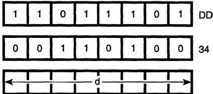
**Description:** The contents of the Index Register IX (register pair IX) are added to a two's complement displacement integer *d* to point to an address in memory. The contents of this address are then incremented.
