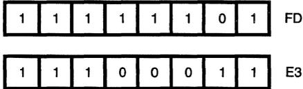
**Description:** The low order byte in Index Register IY is exchanged with the contents of the memory address specified by the contents of register pair SP (Stack Pointer), and the high order byte of IY is exchanged with the next highest memory address (SP+1).
