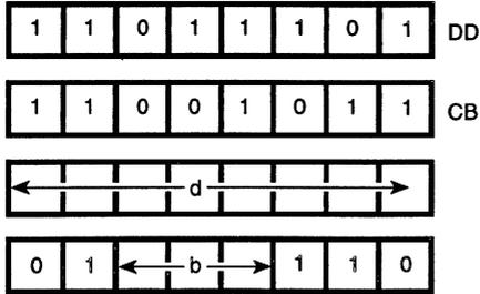
**Description:** This instruction tests bit b in the memory location specified by the contents of register pair IX combined with the two's complement displacement d and sets the Z flag accordingly. Operand b is specified as follows in the assembled object code.
