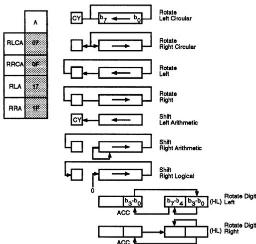
Figure 4-9. Rotates and Shifts
