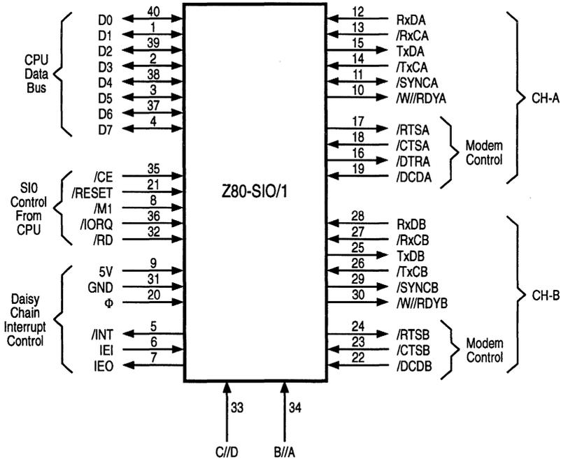
Figure 2-4. Z80-ZIO/1 Pin Assignments
