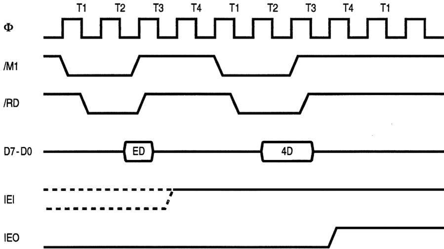
Figure 6-2. Return From Interrupt Cycle
