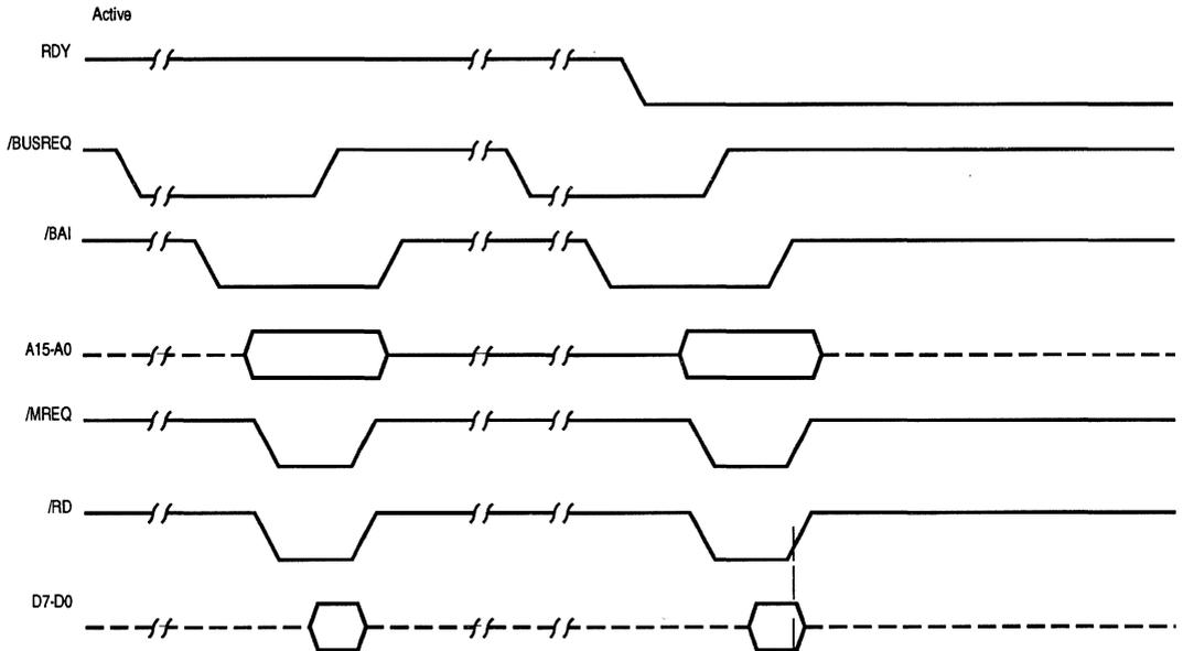
**Figure 8-12. RDY Line in Byte Mode**
