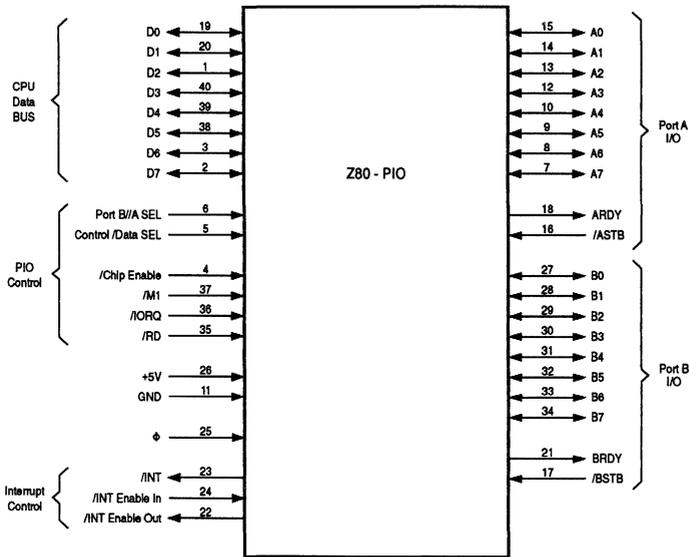
Figure 3-1. PIO Pin Functions
