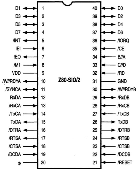
Figure 2-5. Z80-SIO/2 Pin Functions
