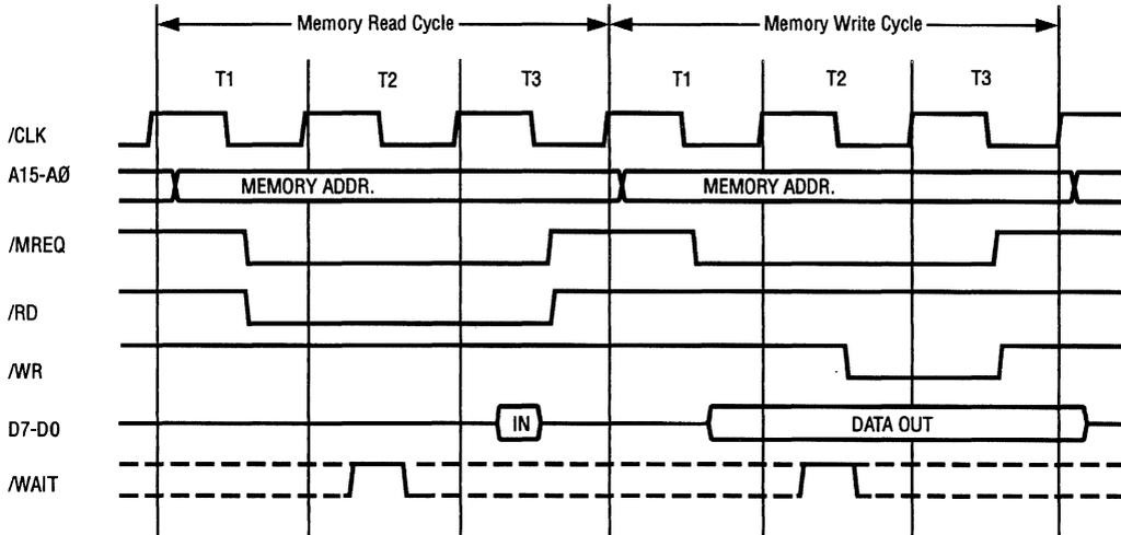
Figure 3-3. Memory Read or Write Cycle
