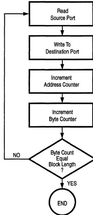
**Figure 1-1. Typical CPU I/O Sequence**
