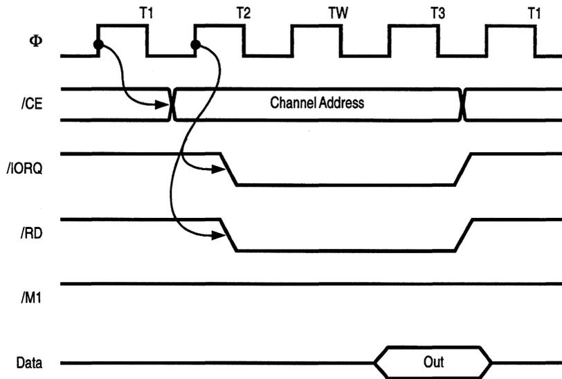
Figure 9-1. Read Cycle Timing
