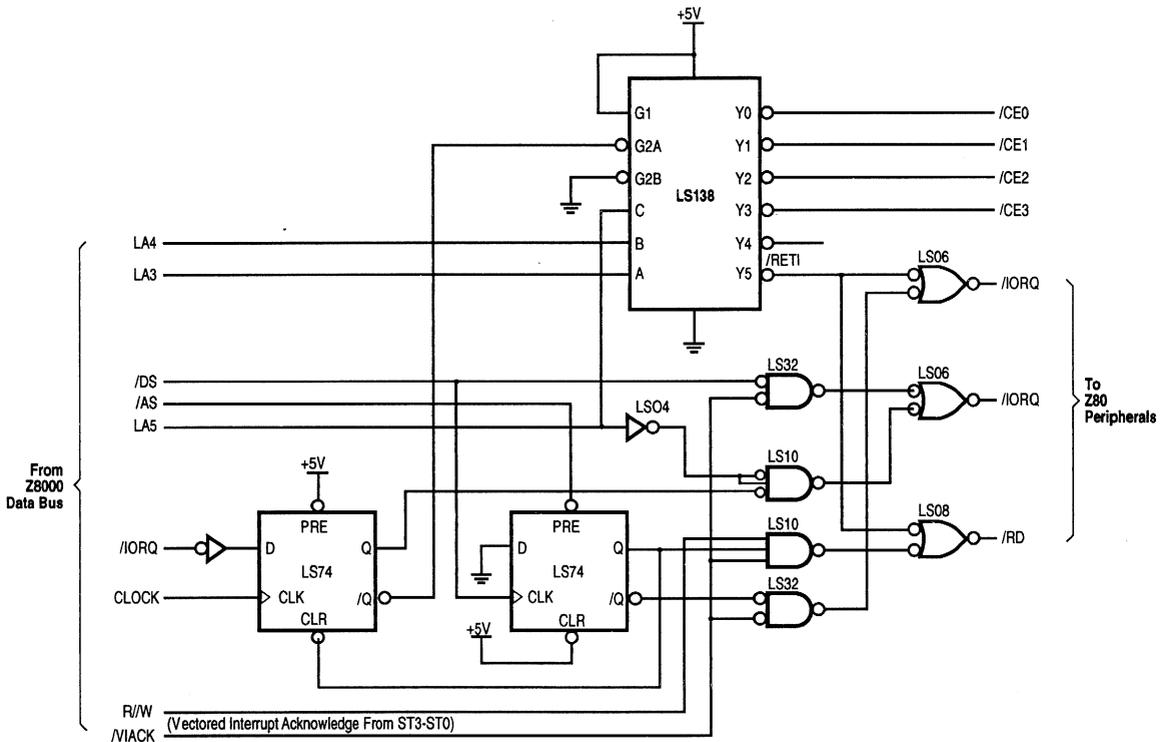
Figure 6-10. Z8000/Z80 Peripheral Interface
