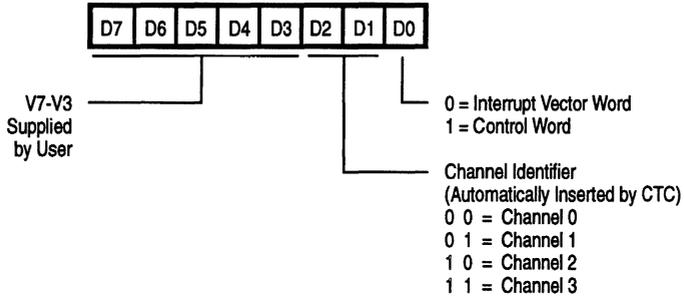
Figure 5-4. Interrupt Vector Register
