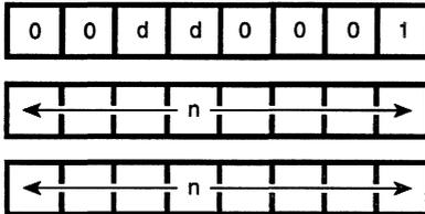
**Description:** The 2-byte integer nn is loaded into the dd register pair, where dd defines the BC, DE, HL, or SP register pairs, assembled as follows in the object code:
