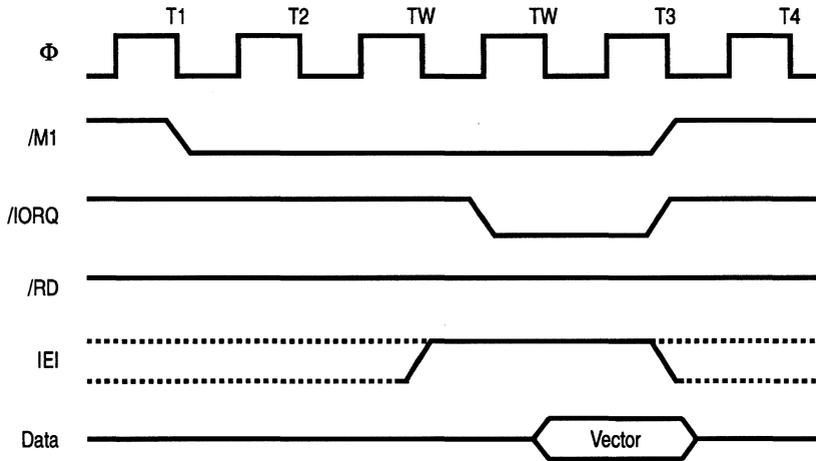
Figure 9-3. Interrupt Acknowledge Cycle Timing
