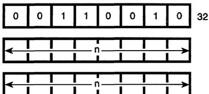
**Description:** The contents of the Accumulator are loaded into the memory address specified by the operand nn. The first n operand after the opcode is the low order byte of nn.
