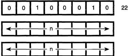
**Description:** The contents of the low order portion of register pair HL (register L) are loaded into memory address (nn), and the contents of the high order portion of HL (register H) are loaded into the next highest memory address (nn+1). The first n operand after the opcode is the low order byte of nn.
