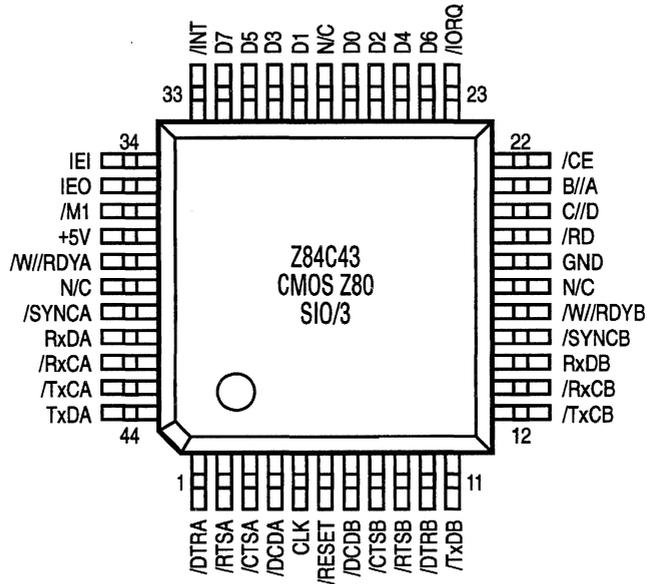
Figure 2-7. Z80-SIO/3 Pin Assignments
