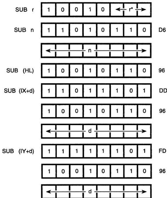
\*r identifies registers B, C, D, E, H, L, or A assembled as follows in the object code field above:
