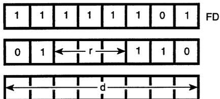
**Description:** The operand (IY+d) (the contents of the Index Register IY summed with a two's complement displacement integer (d) is loaded into register r, where r identifies register A, B, C, D, E, H, or L, assembled as follows in the object code:
