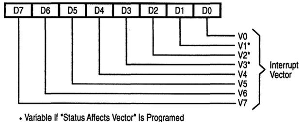
Figure 7-11. Read Register 2 (Channel B Only)
