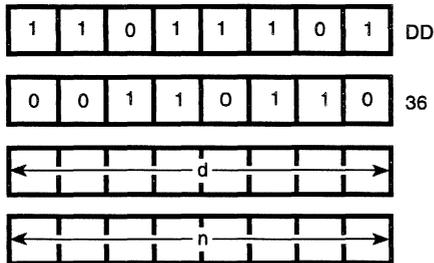
**Description:** The n operand is loaded into the memory address specified by the sum of the Index Register IX and the two's complement displacement operand d.
