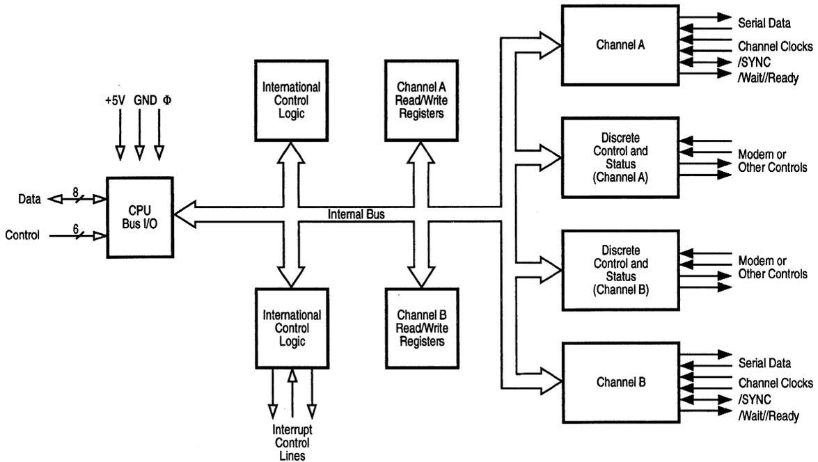
Figure 1-1. Z80-SIO Block Diagram
