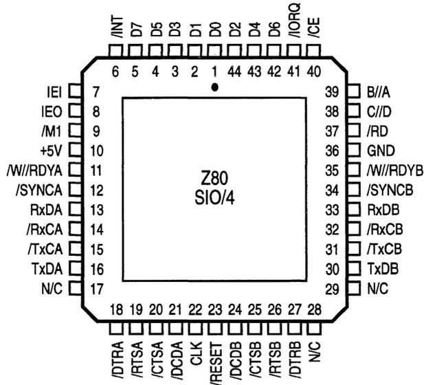
Figure 2-8. Z80-ZIO/4 Pin Assignments
