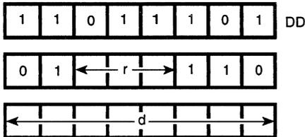
**Description:** The operand (IX+d), (the contents of the Index Register IX summed with a two's complement displacement integer d) is loaded into register r, where r identifies register A, B, C, D, E, H, or L, assembled as follows in the object code:
