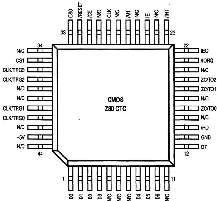
Figure 3-4. 44-pin Quad Flat Pack Pin Assignments
