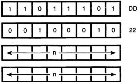
**Description:** The low order byte in Index Register IX is loaded into memory address (nn); the upper order byte is loaded into the next highest address (nn+1). The first n operand after the opcode is the low order byte of nn.
