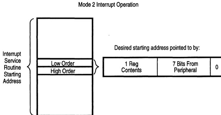
Figure 5-3. Mode 2 Interrupt Operation
