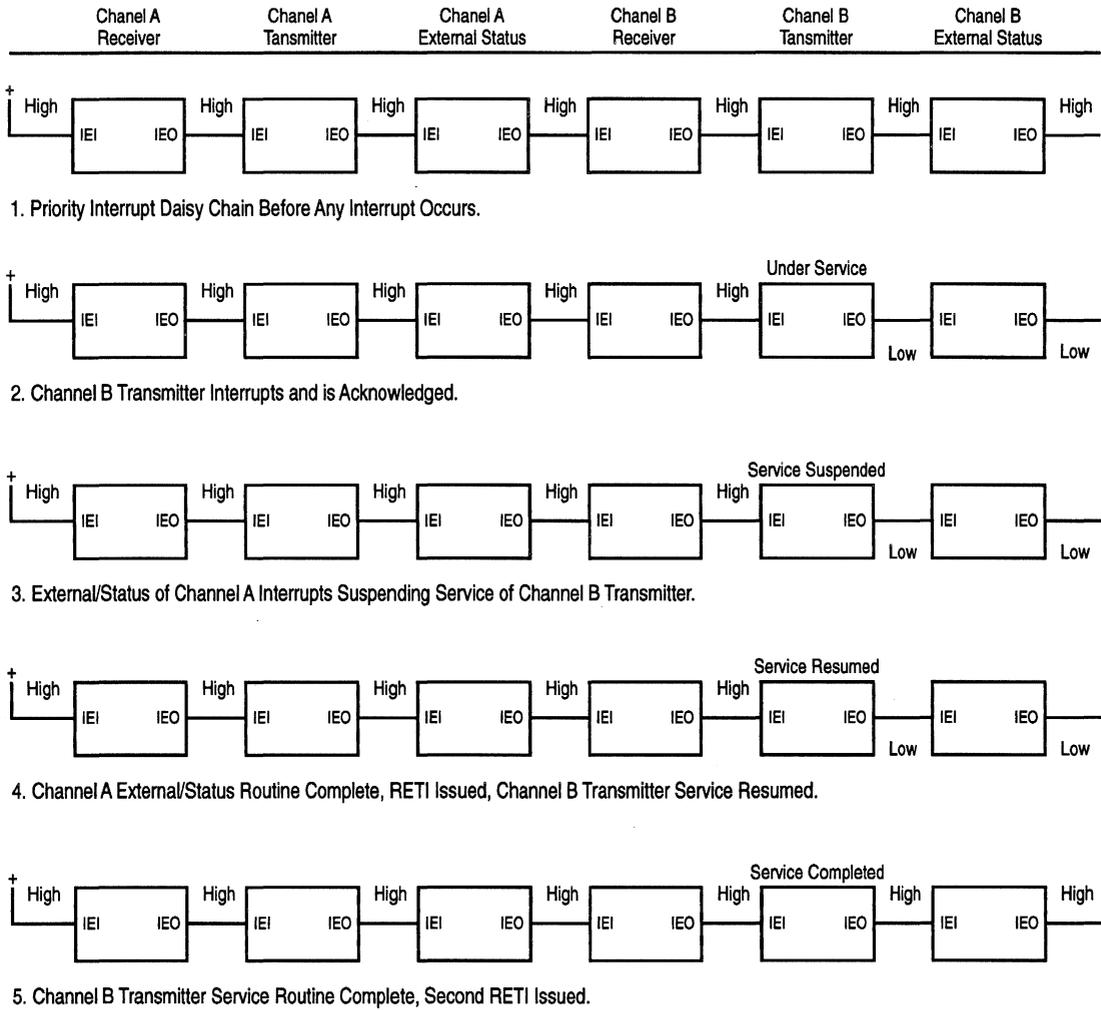
**Figure 9-5. Typical Interrupt Service**
