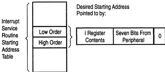
The first byte in the table is the least significant (low order) portion of the address. The programmer must obviously fill this table in with the desired addresses before any interrupts are to be accepted.
