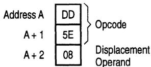
The two extended addressing instructions are also three byte instructions. For example, the instruction to load the accumulator with the operand in memory location 6F32H would be written:
