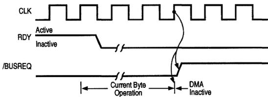
**Figure 8-11. Bus Release on Not Ready (Burst Mode)**
