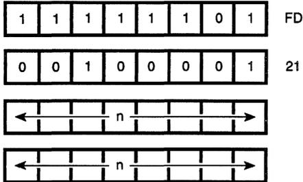
**Description:** Integer nn is loaded into the Index Register IY. The first n operand after the opcode is the low order byte.
