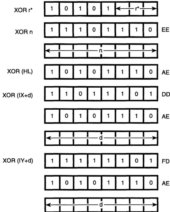
\*r identifies registers B, C, D, E, H, L, or A specified as follows in the assembled object code field above:
