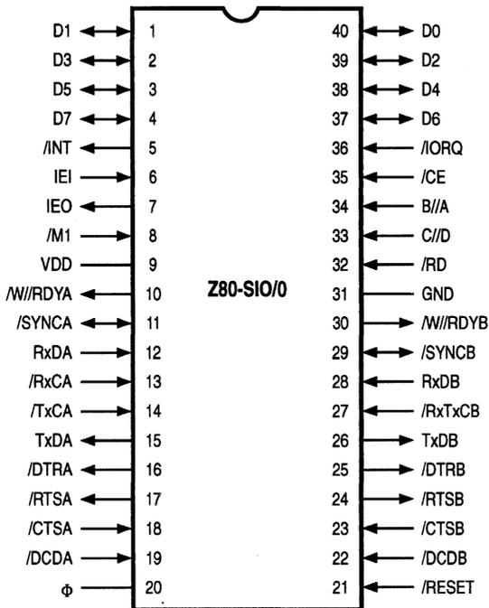
Figure 2-1. Z80-SIO/0 Pin Functions
