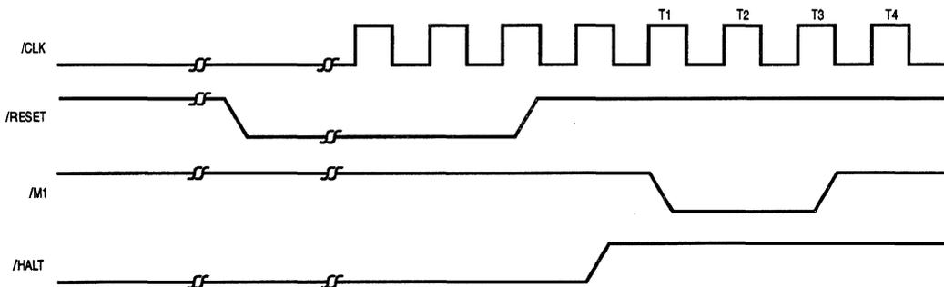
Figure 3-11. Power-Down Release Cycle No. 2
