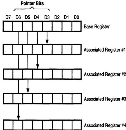
**Figure 5-1. Method of Write-Register Pointing**
