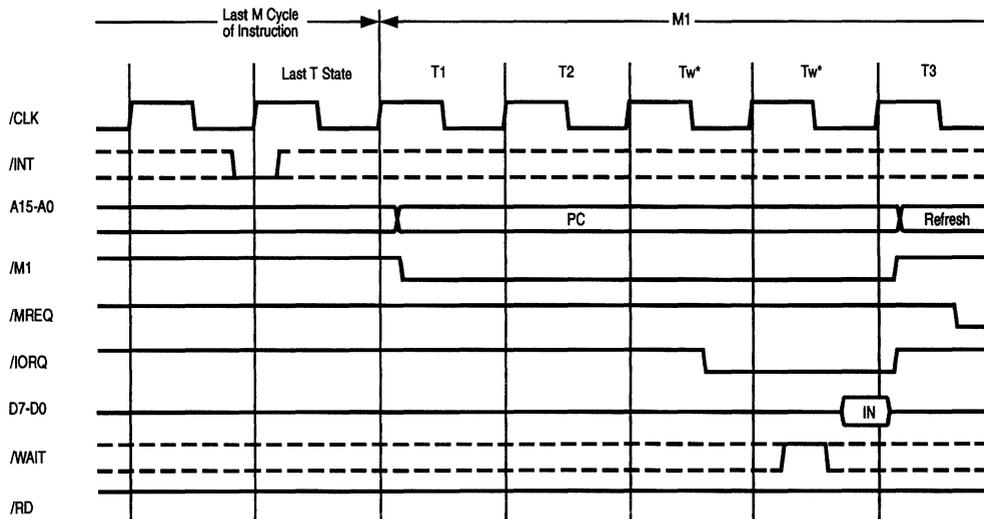
Figure 3-6. Interrupt Request/Acknowledge Cycle
