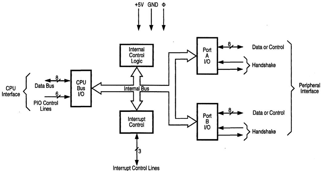
Figure 2-1. PIO Block Diagram
