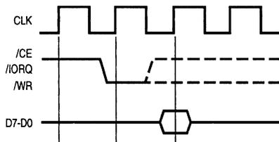
Figure 8-1. CPU-to-DMA Write Cycle Requirements
