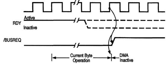
**Figure 8-9. Bus Release on End-of-Block (Burst and Continuous Modes)**
