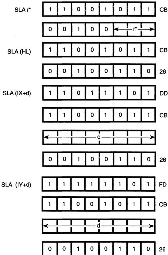
r identifies registers B, C, D, E, H, L, or A specified as follows in the assembled object code field above:
