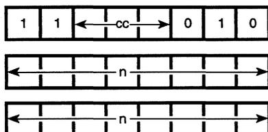
**Note:** The first n operand in this assembled object code is the low order byte of a 2-byte memory address.
