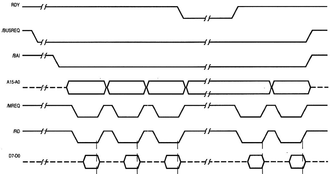
Figure 8-14. RDY Line in Continuous Mode
