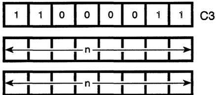
Note: The first operand in this assembled object code is the low order byte of a two-byte address.
