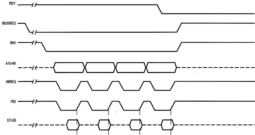
Figure 8-13. RDY Line in Burst Mode
