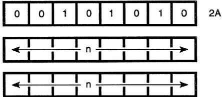
**Description:** The contents of memory address (nn) are loaded into the low order portion of register pair HL (register L), and the contents of the next highest memory address (nn+1) are loaded into the high order portion of HL (register H). The first n operand after the opcode is the low order byte of nn.
