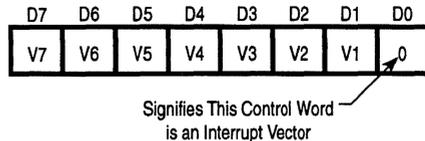
D0 is used in this case as a flag bit which when Low, causes V7 through V1 to be loaded into the vector register. At interrupt acknowledge time, the vector of the interrupting port will appear on the Z80 data bus exactly as shown in the format above.
