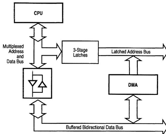
**Figure 6-9. Connecting DMA to Demultiplexed Address/Data Buses**
