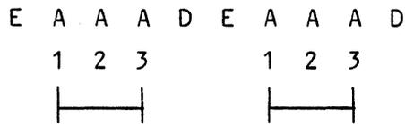
Count begins on the first occurrence of the event to be counted (ALTERNATE resource) after the ENABLE sequence is recognized. The counter stops after the first Disable sequence. The counter is reset to 1 on the first occurrence of the event to be counted in the next interval (ENABLE sequence recognized). The previous count is lost if it is not stored in Trace Memory (see HP command).
