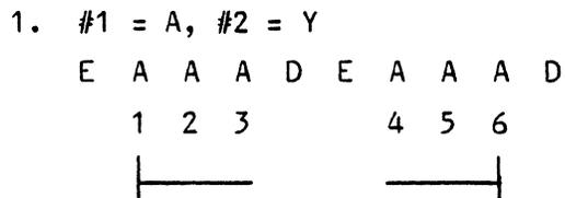
In example 1, the count begins on the first occurrence of the event to be counted (ALTERNATE resource) after the ENABLE sequence is recognized. The counter pauses after the first DISABLE sequence is recognized. The counter resumes after the next ENABLE sequence and stops after the subsequent DISABLE sequence.
