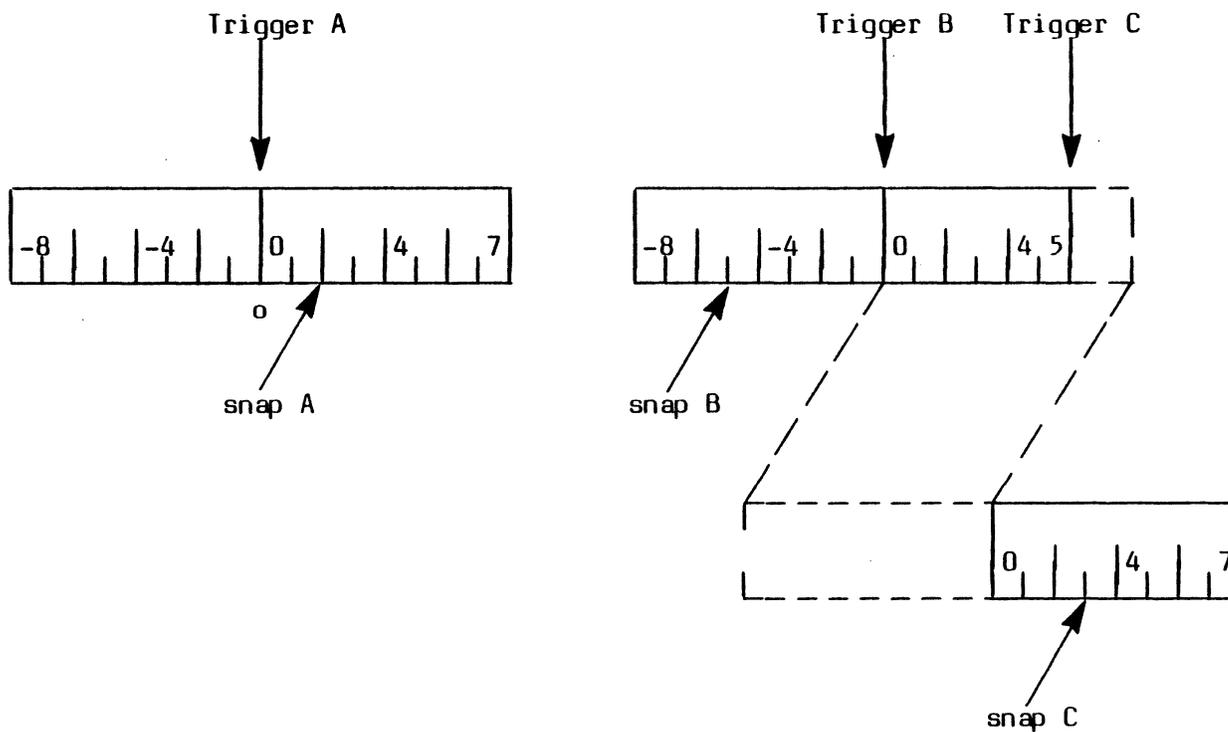
**Figure 4-4. Triggers Occurring During a Cycle Delay**
