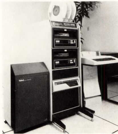
The low-profile Line 2 Power Conditioner from Topaz protects minicomputers from noise and sags, and doubles as a distribution unit.
