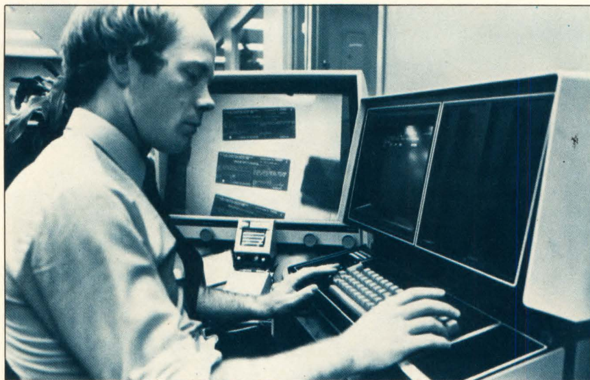
The Bank of California chose a computer-assisted retrieval (CAR) system from 3M. CAR systems, which can stand alone or operate online, search for documents via computer terminal. The most sophisticated models retrieve digitized images stored in the central computer and reproduce them on a terminal's display screen like the one at records management specialist Don Smythe's left in photo below.
