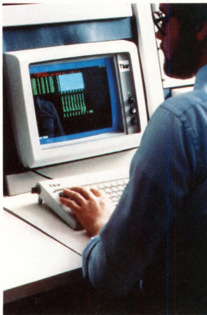
T-bar's Virtual Matrix Switch allows an operator to monitor and test communications lines in both directions from a central location.
