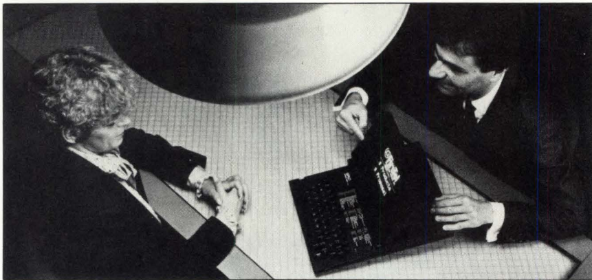
Data General's new battery-operated briefcase portable (9.1 pounds) operates software written for the MS-DOS, CPM-86, and Xenix operating systems. With 256 Kbytes of memory and two disk drives, the portable costs $4,095. The liquid-crystal display is 80 columns by 25 lines.
