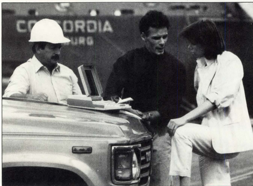
Grid Systems' Compass is one of the few lap-top portables with a full-size screen. Thanks to its internal luminescence, the flat panel display is easily viewable in spite of any external light source.
