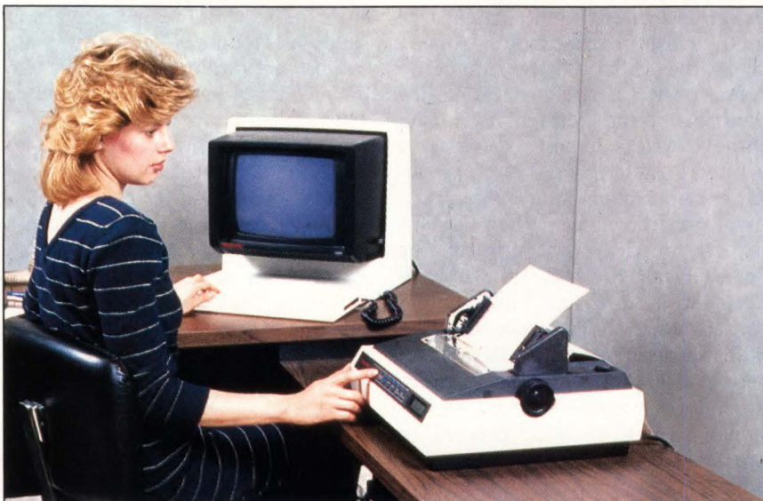
AT&T Teletype's 5310B dot-matrix printing terminal prints up to six copies of a document at 200 characters per second.
