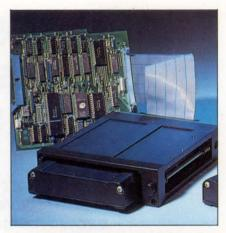
Ruggedized nonvolatile CMOS RAM data storage systems such as these from Targa Electronics Systems meet the three important criteria for use in harsh environments: reliability, cost and speed.
