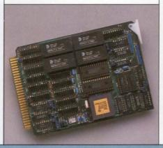
Two modes of operation are possible with the DSP: stand-alone or slave. In the stand-alone mode, the board doesn't generate bus requests or require bus acknowledgements to execute I/O operations. This mode accommodates full I/O interrupt handling. In a multiprocessor configuration using the device as a slave, communication takes place through the dual-port memory, letting only one processor assume the task of handling interrupts.
