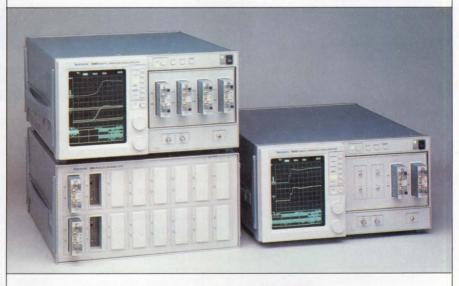
with 16 continually updated automatic time and amplitude measurements. Mean and standard deviation statistics are provided for all measurements.
