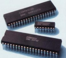
oscillator, this highly integrated IC contains all the logic necessary to control a tokenpassing ARCNET interface across standard coax, twisted pair or fiber optic cable. The COM90C62's high level of integration allows inclusion of a LAN interface directly on a PC mother board.
