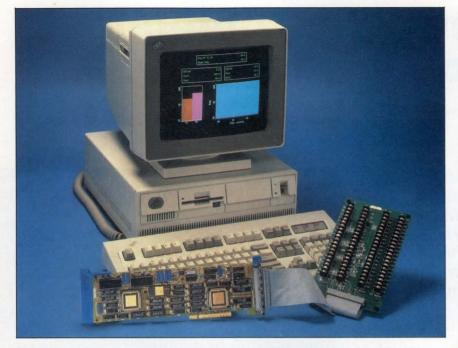
Micro Channel board makers face such difficulties as limited real estate, limited power allocation and rigorous mechanical demands. These difficulties have ironically driven some vendors to ambitious efforts, as in this Micro Channel board from Data Translation that simultaneously manages analog input, analog output and digital I/O operations.
