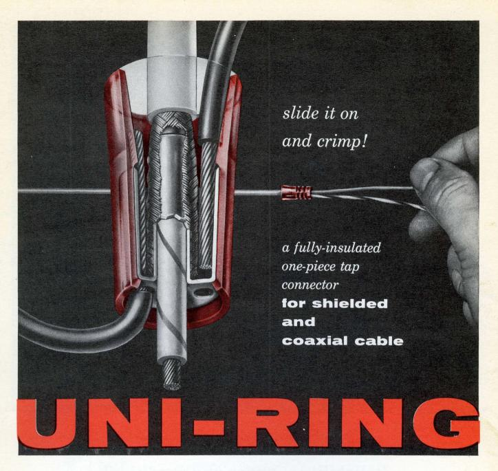
UNI-RING offers a tremendous saving in installation time over any previous method of tapping or terminating shielded or coaxial cable. As the inner ring slides under the shielded braid, the tap wire is held between the braid and the outer ring. Single or multiple taps, from either the front or back of the connector, can be accommodated ... A single crimp, using the same basic HYTOOLS used for installing HYRINGS, completes the uniform, secure, and insulated assembly.
