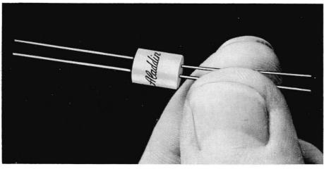
At left is a pulse transformer, .285 inches in diameter, and .350 inches long, held between thumb and forefinger. The core is ferrite; the two or more windings are made of size 48 wire. Many largescale electronic data processing machines contain 1500 or more pulse transformers. This one is made by Aladdin Industries, Nashville, Tenn. (Figure 20)
