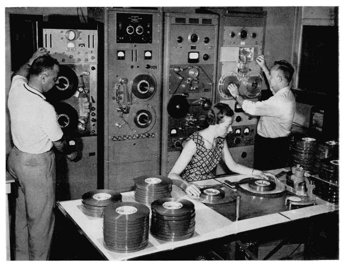
Here, a battery of automatic machines at Audio Devices, Inc., N.Y., makes 100% inspection of magnetic tape intended for use on computers, data processors, instrumentation recorders, etc. Several million pulses are recorded on each reel of tape; if even a single pulse fails to reproduce properly for a tape under test, the machine automatically stops and signals the operator, and the reel is rejected for computer use. (Figure 3)
