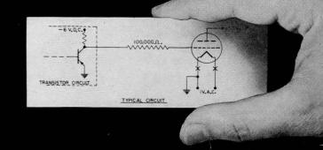
Heater voltage is only 1 volt, 30 ma, AC or DC. The anode will draw only 0.5 ma from a 50 volt DC supply during the zero-bias "on" condition. A 3.0 volt DC voltage is sufficient to cut-off plate current and light. Write for data sheet to Semiconductor and Special Purpose Tube Division, Amperex Electronic Corp., 230 Duffy Avenue, Hicksville, L.I., N.Y.
