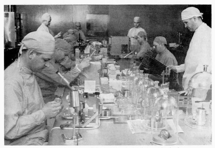
Men at Sperry Gyroscope producing inertial navigation devices under dust-free conditions.
