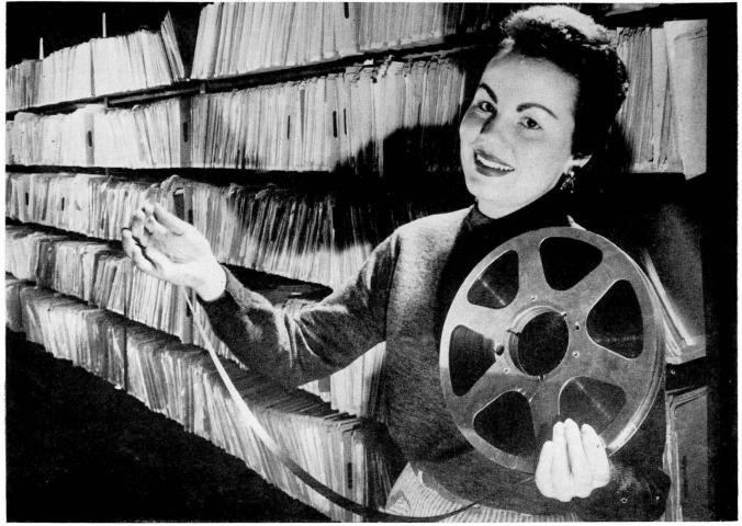
This single reel of magnetic tape holds as much information as ten of the file shelves. This reel of magnetic tape contains 2400 feet of magnetic tape and stores information at the rate of 125 characters to the inch. The scene is the Army Ordnance Tank-Automotive Command in Detroit, and the equipment is RCA's Bizmac. (Figure 1)
