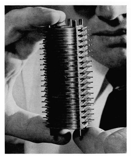
At left is an assembly of 18 magnetic heads, for reading from or recording on magnetic tape three inches wide; the device will handle 60,000 decimal digits per second. This is part of the Datamatic 1000 Electronic Dataprocessing System, made by Datamatic Corp., Newton, Mass. (Figure 17)
