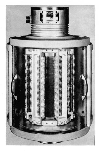
This magnetic drum (at left) is 5 inches in diameter and 12 inches long; it can turn at speeds up to 12,000 revolutions per minute, permits 240 magnetic read/record heads, and can store as many as 625,000 binary digits of information. This is the Type 512A drum made by the Bryant Gage and Spindle Division, Springfield, Vt. (Figure 12)
