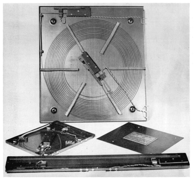
Here is a delay line of the magnetostriction type, stable under changing temperatures. Such a delay line will provide up to 1/200 of a second delay for separate pulses as fast as one million a second. It is made by Ferranti Electric, Inc., Hempstead, N.Y. (Figure 19)
