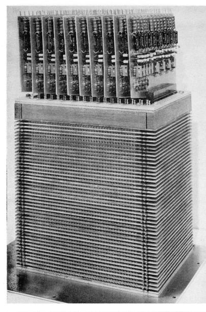
At left is a unit of the core memory stack of the Univac II, of Remington Rand Univac. It consists of about 44 core memory planes, and has a capacity of 24,000 characters. Any register in this memory will supply the information it holds within a few millionths of a second after the call for the information. (Figure 8)
