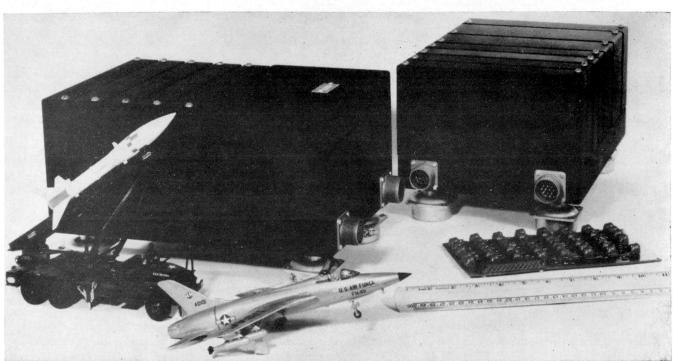
This complete digital computer above, although not much larger than the plastic models of aircraft and missiles shown, processes enough information to make a modern fighter-bomber nearly automatic. The computer is GEVIC, General Electric Variable Increment Computer; it was designed and developed by GE Light Military Electronics Department, Utica, N.Y. One of the circuit modules is also shown. (Figure 2)
