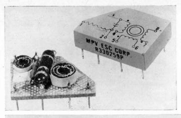
At left is a magnetic shift register, one bit per core, information rate 5000 kilocycle, size 2/10 of a cubic inch, made by ESC Corp., Palisades Park, N.J. (Figure 20)
