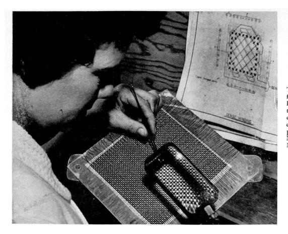
The operator is sewing fine strands of insulated copper wire through tiny magnetic cores, in order to make computer memory planes, at RCA's plant, Needham Heights, Mass. (Figure 11)
