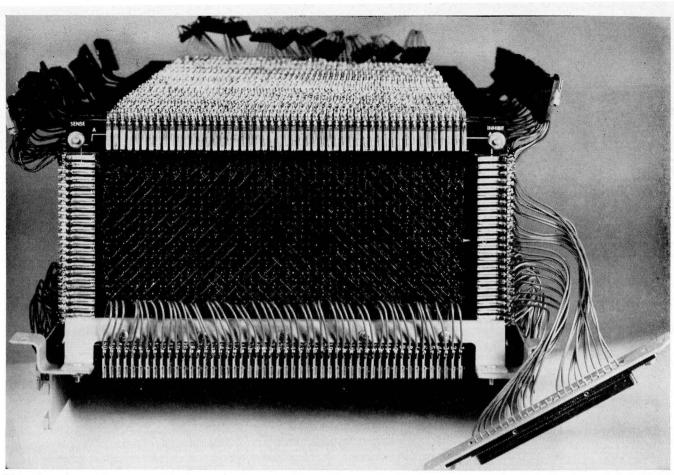
Here is a magnetic core quick-access memory used in a Burroughs 220 computer. In front is the first plane of 1000 tiny doughnut shaped cores. Behind it are 43 more just like it. The memory is entered in parallel by impulsing the same core position in each one of the 44 planes; access time is 10 microseconds. The memory is made by the ElectroData Division of Burroughs Corp., Pasadena, Calif. (Figure 6)
