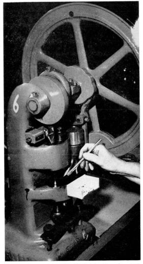
This press squeezes out tiny rings of ferrite powder, which after heating and testing will become ferrite cores for computer memory frames. The place is the RCA plant, Needham Heights, Mass. (Figure 14)
