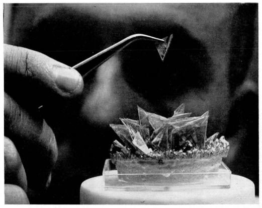
These synthetic crystals are the basic material for an experimental logical device for an electronic business machine. They were crystallized in the research laboratories of the National Cash Register Company, Dayton, Ohio. (Figure 19)
