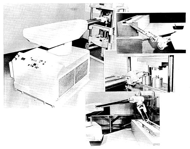
— Shown here in a simulated factory activity, Unimate, the new "teachable" robot, by Consolidated Controls Corporation, picks billets from a feed chute, puts them through a two-stage forging operation and delivers the finished parts to a conveyer.
