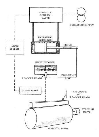
As used in Unimate, the magnetic memory drum has a capacity of 16,000 bits of information. These are recorded in 200 rows around the circumference, each row consisting of 80 bits parallel to the drum axis. The 200 rows correspond to the number of distinct movements which Unimate can "remember". The 80 parallel bits per row represent the number necessary to control all of the functions which may be needed for Unimate to make a movement and to actuate auxiliary machinery.
