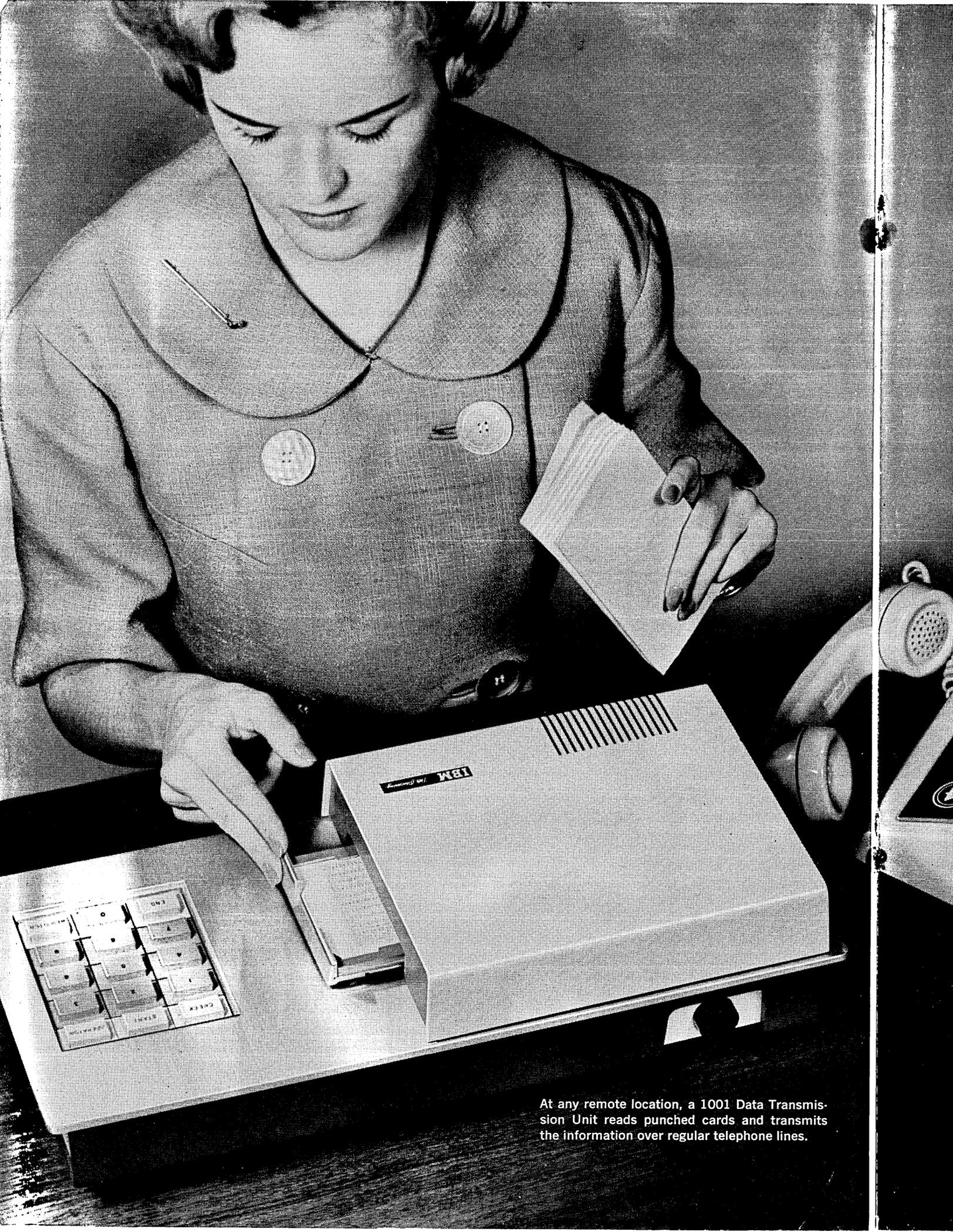
At any remote location, a 1001 Data Transmission Unit reads punched cards and transmits the information over regular telephone lines.
