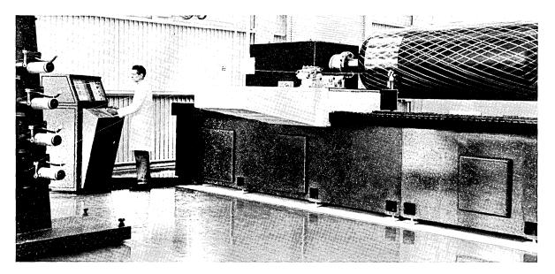
"Director Control System" -- Thompson-Ramo-Wooldridge Inc., Michigan City, Ind. has developed for the Rohr Aircraft Corp., Riverside, Calif., a numerical control system for winding missile fuel tanks with fiber glass. The machine makes light, strong, rocket-engine cases for the larger and more advanced ballistic missiles. The shapes and winding patterns are determined by a computer, which in turn programs the machine to produce them.
