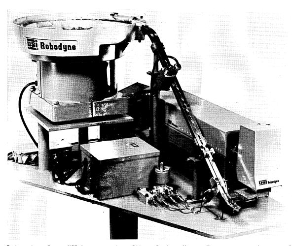
U.S. Industries, Inc., USI Robodyne Div., Silver Spring, Md. -- The segmented vibratory feeding bowl supplies small components to the waiting jaws of an automated TransfeRobot 200. The segmented bowl is so constructed that one small piece can be detached and another inserted to make the bowl ready for a different assembly task.
