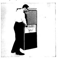
The 910 is the first random access, buffered input/output digital computer to be priced below \$90,000. Although designed primarily for systems use, its high speed, working flexibility, and excellent performance allow it to be used as an extremely low cost general purpose machine. The 910 operates directly, without special coupling, with all types of input/output devices, including magnetic tape units, A-D converters, automatic typewriters and line printers.
