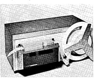
There are very few moving parts in the Facit PE 1000. Tape can be inserted and secured in a couple of seconds. If an incorrectly punched character stops the reader, the character is immediately visible. The error can be flagged because the reader can be stopped after every character. The Facit PE 1000 is convertible for 4, 6, 7 or 8-track punched tape. A simple hand motion performs the changeover.
