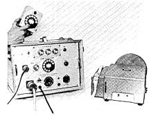
can be converted to cards for machine sorting and/or computer operation. The company recommends the Friden #1294-021 tape punch unit. The recorder can be modified to use other tape punch units. The recorder is useful for analyzing performance of processing or manufacturing units, small research and development projects, semi-works or pilot plant operation, and for study of manufacturing systems.
