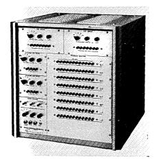
The Digital Program Generator is designed for high-speed test of memory cores, twistors, and thin film devices. It also may be used independently for development of computer circuits and logic as well as for a high-speed clock or for word generation. (For more information, circle 79 on the Readers Service Card.)
