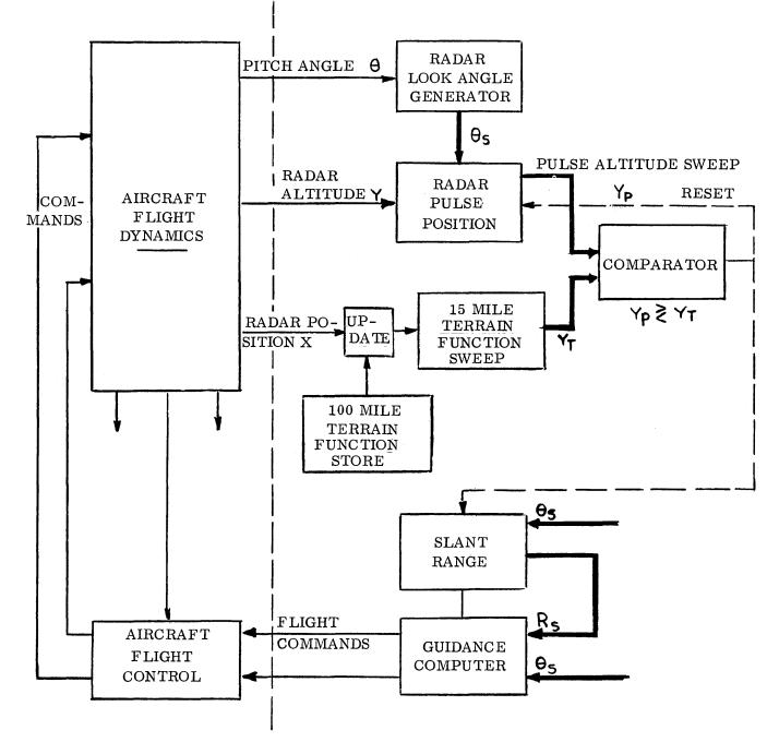
Figure 5. Block Diagram
