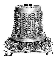
These memory drums, designated series 1200, are 13" in diameter, with heights from 11.375" to 21.875". Drum speeds range from 900 to 12,000 rpm. They are supplied with from 55 to 540 tracks. Storage capacities range from 50,000 to 3,500,000 bits.
