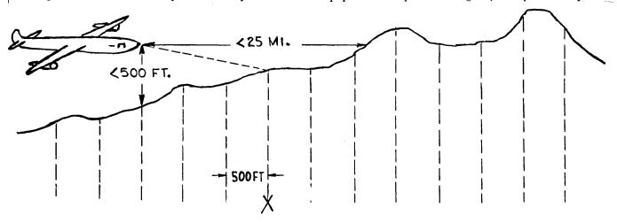
Figure 4. Terrain Avoidance Guidance
