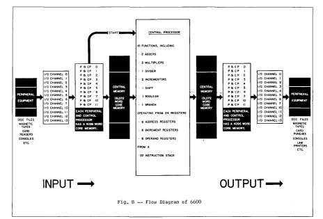
Each processor has a 12-bit, 4096 word memory (not a part of central memory) and an 18-bit adder. The repertoire of instructions allows each processor access to central memory and the central processor, and features flexible I/O and logical operations, plus 18-bit add and subtract capability. Indirect addressing is also provided.
