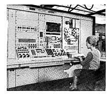
The new computer will enable scientists and engineers to solve a growing class of design and simulation problems beyond the scope of conventional separate analog and digital equipment. It is particularly suited to 'real time' problem solving and simulation in major aerospace and industrial process control applications.
