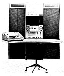
An extensive programming system is available for the new PDP-7 and includes a FORTRAN operating system, FORTRAN compiler and library, symbolic assembler and relocating linking loader, on-line symbolic debugging program, symbolic tape editor, and arithmetic utility, and maintenance routines. (For more information, circle 30 on the Readers Service Card.)
