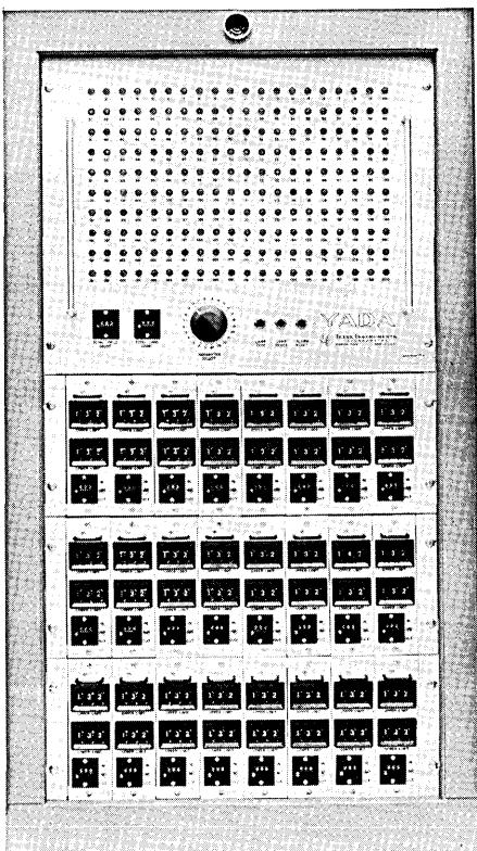
YADA, MODEL 858 / Texas Instruments, Inc. — Yield and Distribution Analyzer (YADA) Model 858 for punched card data analyzing quickly summarizes data which pass within preset limits compared against preset upper and lower values. A yield counter totals the units passing; a device counter totals units compared. The 858 analyzes three or four digit parameters and will read and compare 72 columns of an 80 column IBM card simultaneously. (For more information, circle 62 on the Readers Service Card.)
