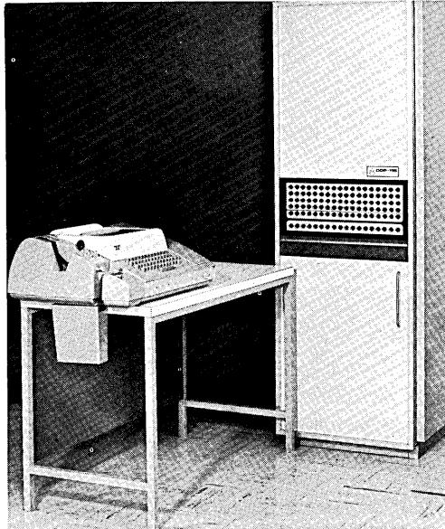
DDP-116 / Computer Control Company, Inc. — This low cost, 16-bit digital computer has indexing, multi-level indirect addressing and priority interrupt. It performs up to 294,000 computations per second. Basic memory cycle is 1.7 microseconds; add time is 3.4 microseconds; and the memory is expandable up to 32,768 words. The DDP-116 is designed for both open-shop scientific applications and real-time data processing. (For more information, circle 49 on the Readers Service Card.)
