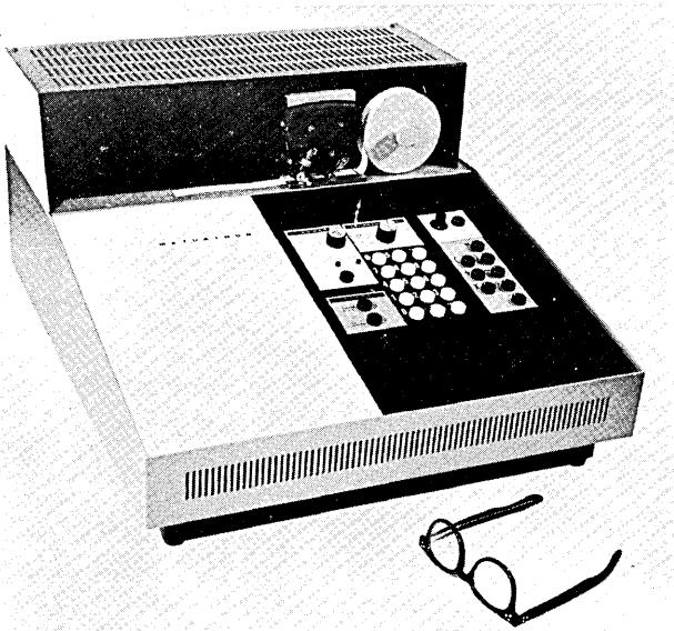
MATHATRON / Mathatronics, Inc. — This desk-top computer/calculator includes a ten-key direct input keyboard, storage registers, ferrite-core program memory storage, solid-state computer logic, and printed output. Extra storage registers, program memory storage, constants and special pre-wired programs may be added to suit individual computing needs. (For more information, circle 53 on the Readers Service Card.)
