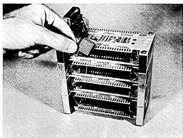
This one-inch square ferrite sheet, perforated with 256 tiny holes, is part of the Call Store temporary memory. The ferrite around each hole acts as a "core" and stores one bit of information. Three wires are threaded through the holes and a conductor is plated onto the sheet. The assembly is used to write information into and read it out of the memory. Sheets are stacked in a module and four modules make up a Call Store, each holding 196,608 bits of erasable information.
