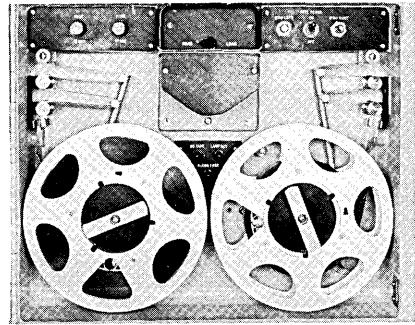
**500RM TAPE READER / Photocircuits Corporation** — The reader utilizes a printed motor direct capstan drive for tape transport, completely eliminating pinch rollers, brakes and clutches. The 500RM will read at speeds up to 500 characters per second and will Wind/Search at 1000 characters per second. The device will accommodate 5, 6, 7 or 8 level tape and has 8 inch reels. Optional polarities for input and output are available. (For more information, circle 98 on the Readers Service Card.)
