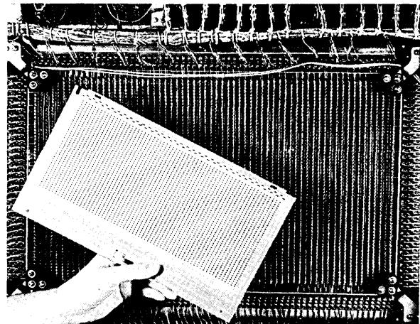
Information ESS No. 1 needs, in order to switch calls and perform other services, is stored on this aluminum card which is inserted between folds of stacked twistor memory planes. A card contains 2816 vicalloy spots arranged in a 64 x 44 array. There are 128 cards in a twistor module and 16 modules in a Program Store. From two to six Program Stores form the semipermanent memory in an electronic central office.
