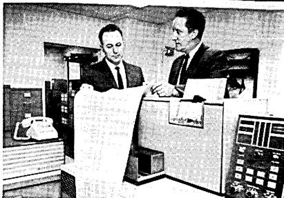
— After calling the firm's computer center, using the Bell System Data-Phone data set at left (top), a clerk inserts punched cards into a Honeywell transmission unit for relay over phone lines directly to the computer which runs a credit check on them. Within hours the originating office receives back information (bottom) on persons identified as having a record of credit delinquency.
