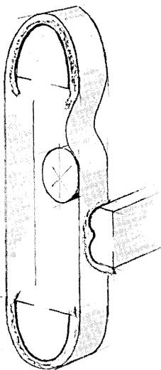
tape loops float over stationary bearings on cushions of air... "fly" past write/read head without making physical contact. Years of trouble-free operation are assured.
