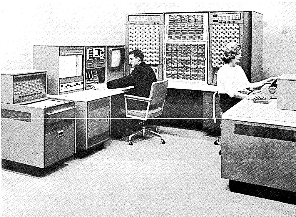
EAI 8800 ANALOG COMPUTER / Electronic Associates, Inc. — This analog/hybrid computer has high-performance analog and digital computing components, a stored-program input/output computer and a complete complement of readout and other peripheral devices. The digital input/output computer automates analog problem preparation, setup and checkout procedures; and provides digital control and monitoring — including hard copy documentation. (For more information, circle 61 on the Readers Service Card.)
