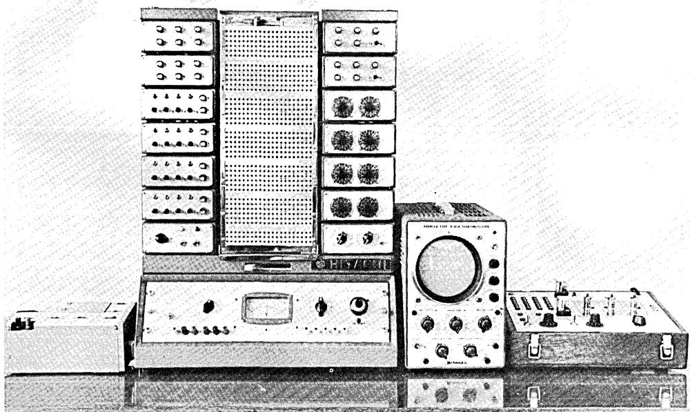
**SERIES WAC-3030 ANALOG COMPUTER /** Hatachi — The desk-top  $\pm 50$  volt Analog Computers, Series WAC-3030 are designed for educational use but can be used on a variety of other applications. Configurations are available with 4 to 24 amplifiers. The picture illustrates the 24-amplifier computer Model WAC-3030-42, with pen writing, single channel recorder; oscilloscope; and linear computing element demonstrator. (For more information, circle 60 on the Readers Service Card.)
