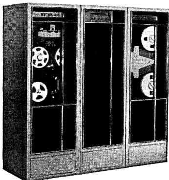
A typical DSI-1000 Data Conversion System. This unit is bi-directional paper tape / magnetic tape.
