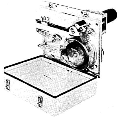
The new tape reader, unusually good for repetitive program playing in general usage, operates unidirectionally at 15 ips (150 cps) stop on sprocket hole and at 100 cps stepping character to character. It uses .003-inch-thick, 1-inch-wide mylar tape. All components of the reader are modular construction. The reader uses no lenses and has a throwaway light source. No electrical adjustments are necessary. (For more information, circle 56 on the Readers Service Card.)
