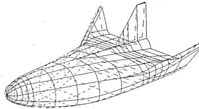
— Three-dimensional perspective drawing of re-entry vehicle was drawn by a computer in Boeing's Aero-Space Division. Exact replica of shape can be carved in aluminum by a tape-controlled machine.
