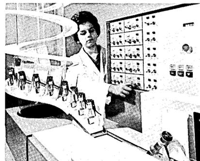
nel. A colorimeter is used to determine hemoglobin value of blood samples by determining the amount of transmitted light. The resulting voltage signal represents the hemoglobin value of the sample.
