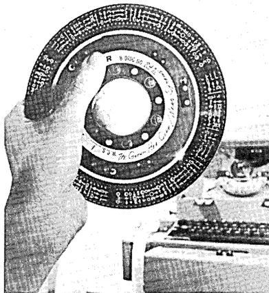
— Victrola-like disc is inserted in photographic unit (background) which contains 40 feet of tightly rolled photosensitive drafting film. Disc revolves and is positioned by commands from coded, 8-channel paper tape. As it does so, a light beam passes through selected symbols making exposures on the film.
