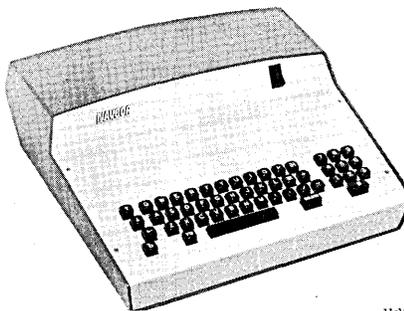
Options include a choice of direct electrical outputs from the reed switches through a diode matrix, or buffered parallel or serial outputs at any specified logic levels. Timing pulses are also available as outputs. (For more information, designate #56 on the Readers Service Card.)
