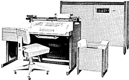
— The magnetic-ledger-card system, shown above, is the smallest NCR Series 500 System. It includes a processor, control console with both alpha and numeric keyboards, and a multi-form carriage printer. Input is available through magnetic ledger cards and keyboard entry. Output is through magnetic ledger cards and carriage printer.
