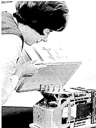
It measures just 15 1/2 x 9 3/8 inches x 8 3/8 inches high, weighs under 46 pounds and consumes only 140 watts of power maximum. The 1824 has been successful in meeting the stringent high reliability, weight, power consumption, acceleration, vibration and temperature requirements imposed on present day aerospace computers. The completely thin-film memory consists of 4096 48-bit words of
