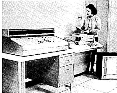
standard 100-word-per-minute teletype unit for each station and central control monitoring, and an ULTRONIC<sup>®</sup> Local Control Unit for installation at each station location (the Central Control Unit at the main office is the same in appearance and size). Not shown are the DATA PUMPS<sup>®</sup> (about the size of a telephone) which would be installed at each station.
