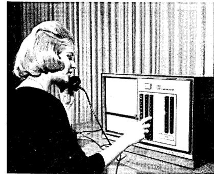
This latest model of CARD (Compact Automatic Retrieval Display) system is a desk top, self-contained microfiche reader. The device contains a file of up to 750 filmcards (microfiche), each of which contains 90 microfilmed pages, providing a total of 67,500 pages of information. Any amount of additional file storage can be contained in magazines external to the machine and be quickly interchanged with identical magazines in the Reader.
