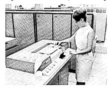
isters, adding machines and accounting machines equipped with optical typefonts, the company reports. The 420-2 reader scans 52 lines of print per second at up to 32 characters per line for a maximum of 1664 characters per second. This reader is internally programmable and has fast (10-second) tape change, automatic editing and variable output formats.
