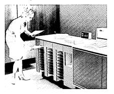
10-bin modules used. The arrangement shown in the picture provides 30 bins. Each bin holds up to 150 copies. A Xerox-designed transport system automatically carries each copy from the 2400 into the sorter. A selector control on the device sets the machine for the number of bins into which copies should be sorted.
