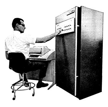
Sigma 2 is a small, very fast, extremely reliable real-time computer with highly sophisticated software.
