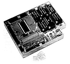
It uses only 1.25 watts of power less than the amount used to turn on a flashlight — to transfer data at a rate of 5000 pieces of information a second. All information is stored in 128 memory words which are randomly accessed. Each word is 21 bits long and is read out a bit at a time.
