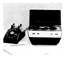
The Vernitron TC-l Telephone Coupler provides for a data transmission rate up to 300 BAUD. Operating frequencies are 1070 and  $1270H_Z$  for send, and 2025 and  $2225H_Z$  for receive. The Coupler comes
