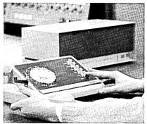
conventional rotary dial, the data telephone includes six pushbuttons which control the voice and data transmission functions and various test operations.
