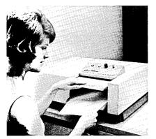
and the copy which is scanned line by line is fed by ordinary telephone lines to a central recognition unit capable of converting the data to punch paper, magnetic tape or punch cards. Since this scanner is located on the user's premises, original documents never have to leave the client. A single unit, as pictured above, can scan with 100% accuracy and convert to computer language the equivalent amount of work done by 12 key punch operators.
