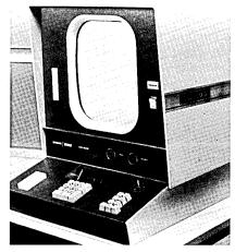
The S/D-500 System consists of a microimage repository that can store intermixed microimages of all sizes and formats, a remote television-style display terminal connected by closed-circuit television to the repository, and a 10-button keyboard control.
