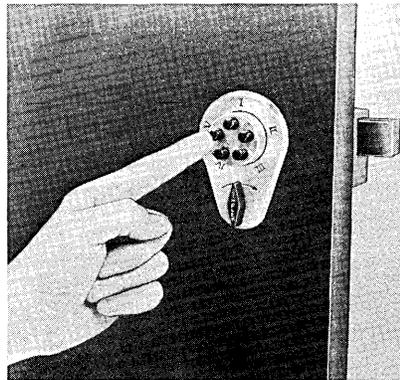
ation possibilities. As an example, 1, 3 and 5 can be pushed in sequence to open a door. Or 1 and 3 may be pushed at the same time, and then 5, to effect an opening. In the latter case, pushing 1 and 3 in sequence will not open the lock; they must be pushed at the same time. From one to five buttons can be used in a combination. Combination changes can be made by any authorized individual — in less than a minute.
