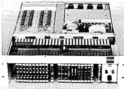
The system is modular in concept with a single memory plane design covering the entire line. Integrated circuits are used in the memory address register, memory information register and control and timing circuits. The memory core stack is a pluggable module and the complete power supply can be removed as a single unit. (For more information, designate #47 on the Reader Service Card.)
