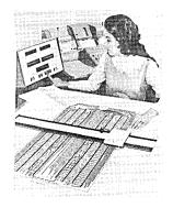
In the front cover picture, the design of a circuit is being converted directly into computer language. As the operator traces the drawing, a MicroMetric digitizing system converts drawing coordinates into digital language. For more information, see page 52.
