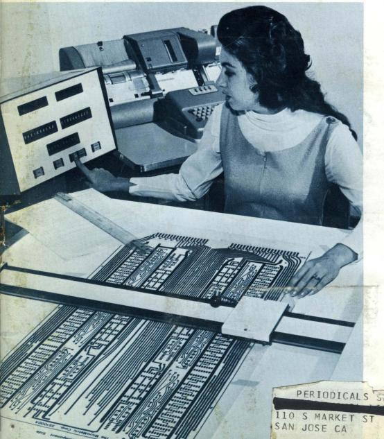
Programming a Computer by Tracing Lines
