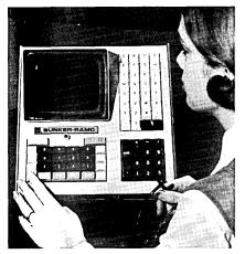
type keyboard enables entries and interrogations by operators with no typing skill. The simple operating procedure requires very little training.
