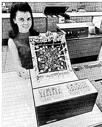
— Janice M. O'Brien, of Honeywell, is shown holding an integrated circuit in one hand and a photographic enlargement of a circuit in the other. Flatpacks on circuit boards are shown in foreground.
