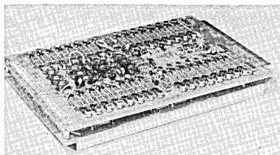
The Model 140 includes: full, half, and split cycle modes of operation; random address; parity line data, address, and control line input/output; TTL integrated circuit interface; 40 watts average power consumption; and 0-50°C operating temperature range. The compact device measures 8-5/8" W by 1-7/8" H by 12'1/2" D, and weighs 3.5 lbs. The MSI-140 core memory may be ordered as a separate memory subassembly or as part of a complete system.
