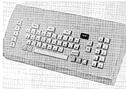
— Expanded keyboard designed and built for Air France by NAVCOR, Inc.
