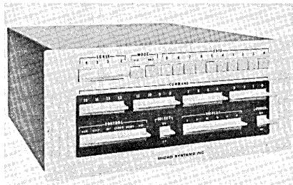
The new machine has a 1.1 microsecond full cycle core memory with 220 nanosecond micro-command execution time; core memory is expandable from zero to 32,768 bytes (8, 9, or 10 bits) in 4096 byte increments to meet the configuration for any application. Read-only storage is expandable from 256 to 1024 words in modules of 256 words. File registers are a set of 16 general-purpose 8-bit registers. (For more information, circle #46 on the Reader Service Card.)
