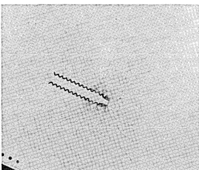
effect upon each grid point, and plotting devices produce "synthetic seismographic patterns" like the one shown in the picture above. When a seismographic pattern thus created resembles one generated by a real earthquake, the research team concludes that the laboratory earthquake was a close approximation of the real quake. They can then draw conclusions about the activity below the earth's surface that triggered the actual jolt.
