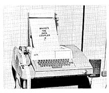
The terminal, suited to a wide range of applications such as time sharing, terminal to terminal communications and computer access, transmits and receives at 100 words per minute. A fully filtered transmitter and receiver data set rejects harmonic and spurious signals assuring error free transmission.
