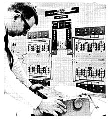
The 1800 checks the instruments for variation from normal every two minutes. To gather all other operating data, the computer "polls" each of the sensors every two minutes. The electronic messages are converted into numbers which are printed in report form hourly on the control room terminal. At midnight, a 24-hour summary is printed.
